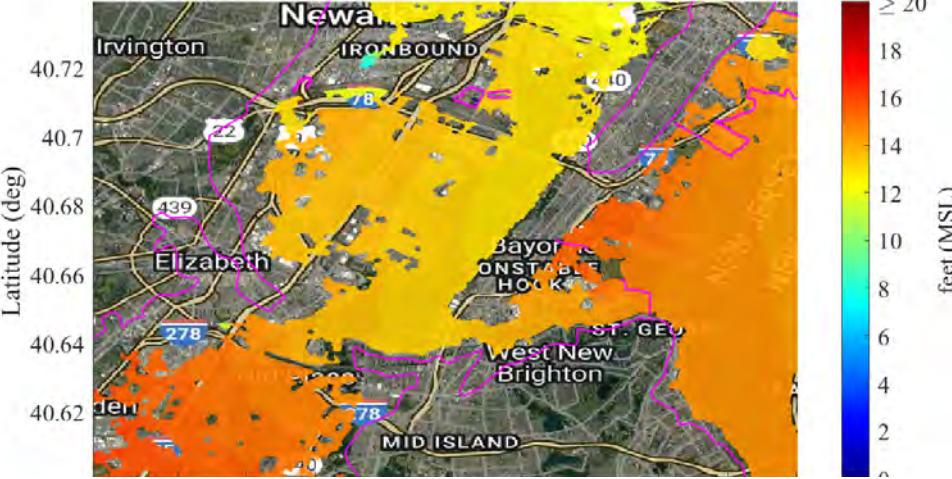
Maximum Water Surface Elevation
