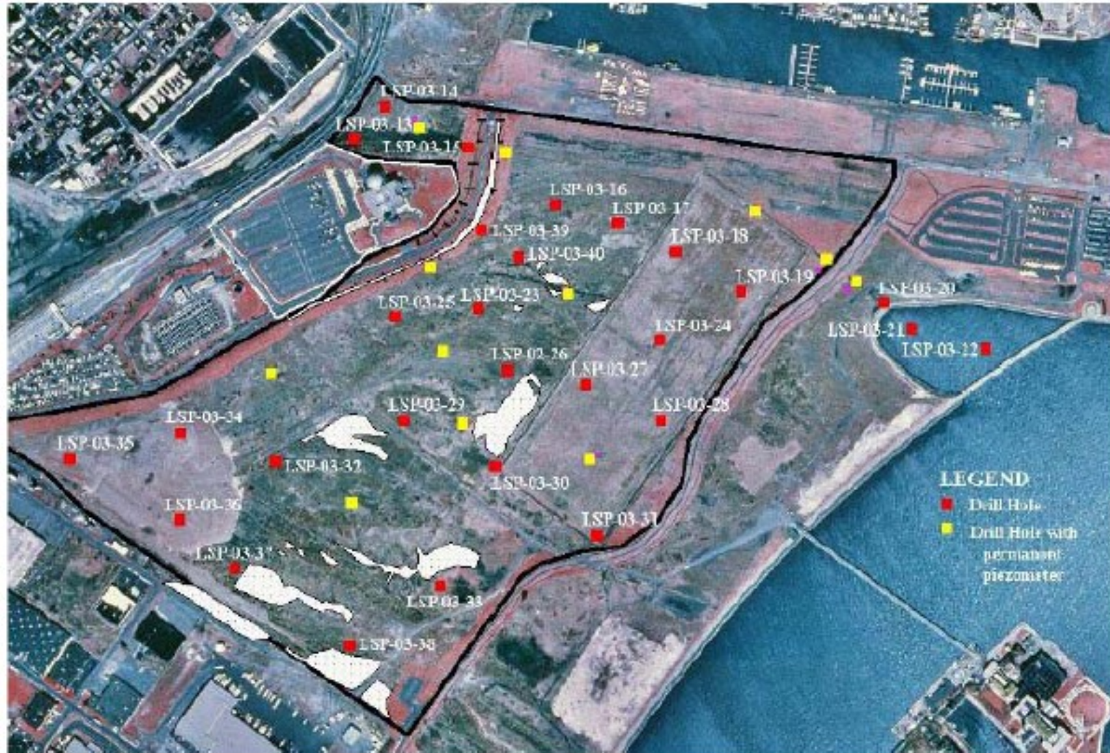
Figure 2.6. 1 st Round Geotechnical and HTRW sampling locations
