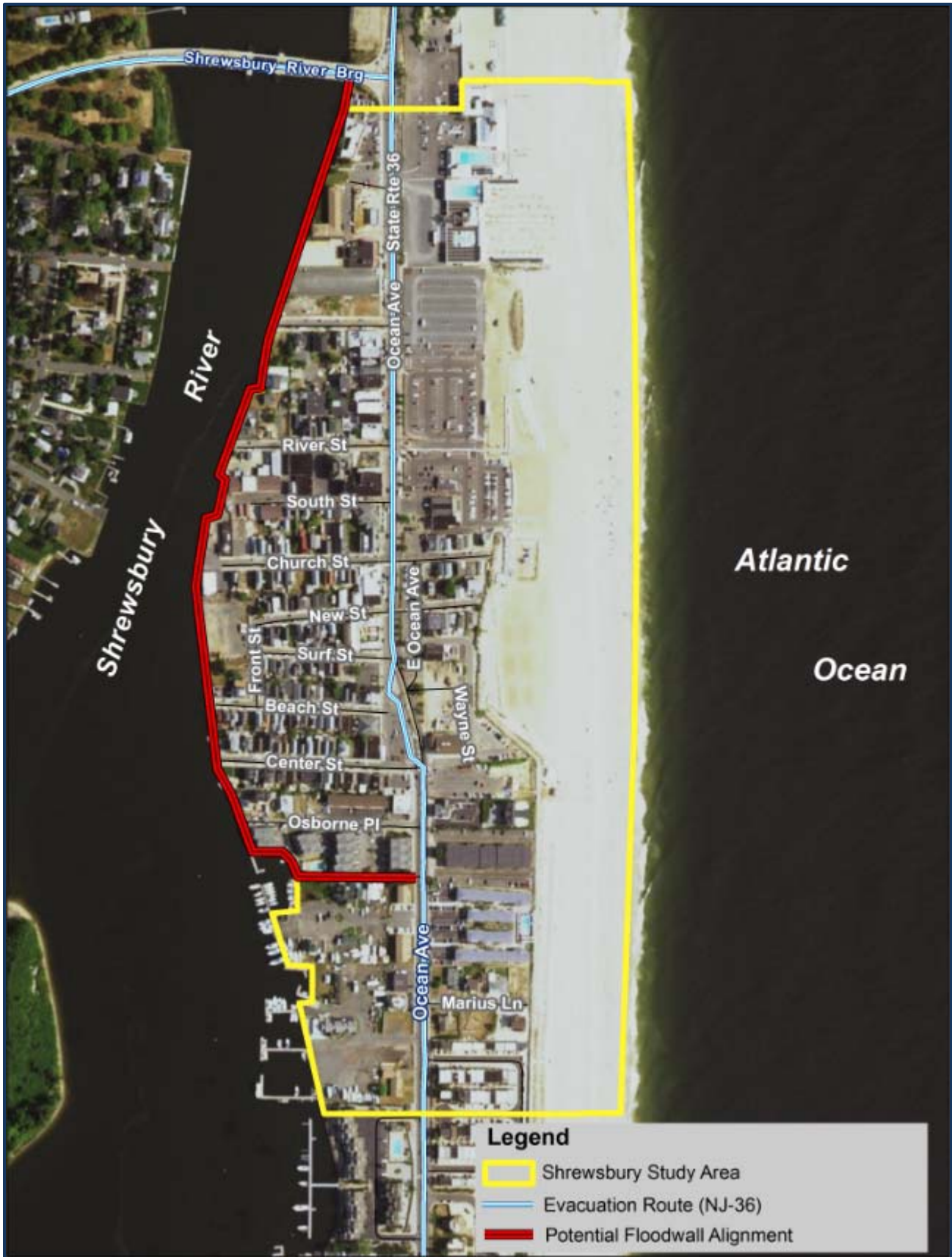
Figure 23: Floodwall alternative alignment.
