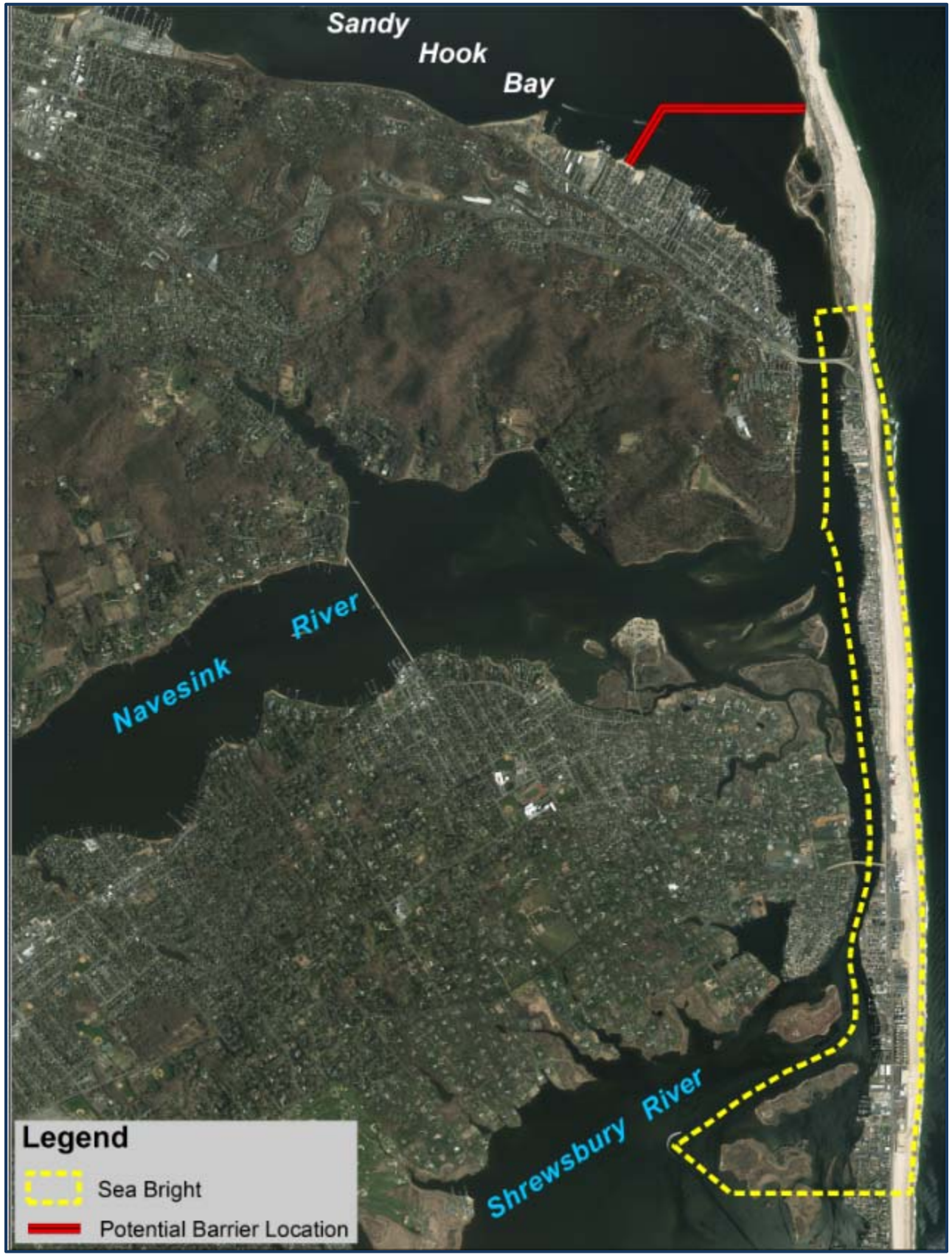
Figure 24: Storm surge barrier alternative.
