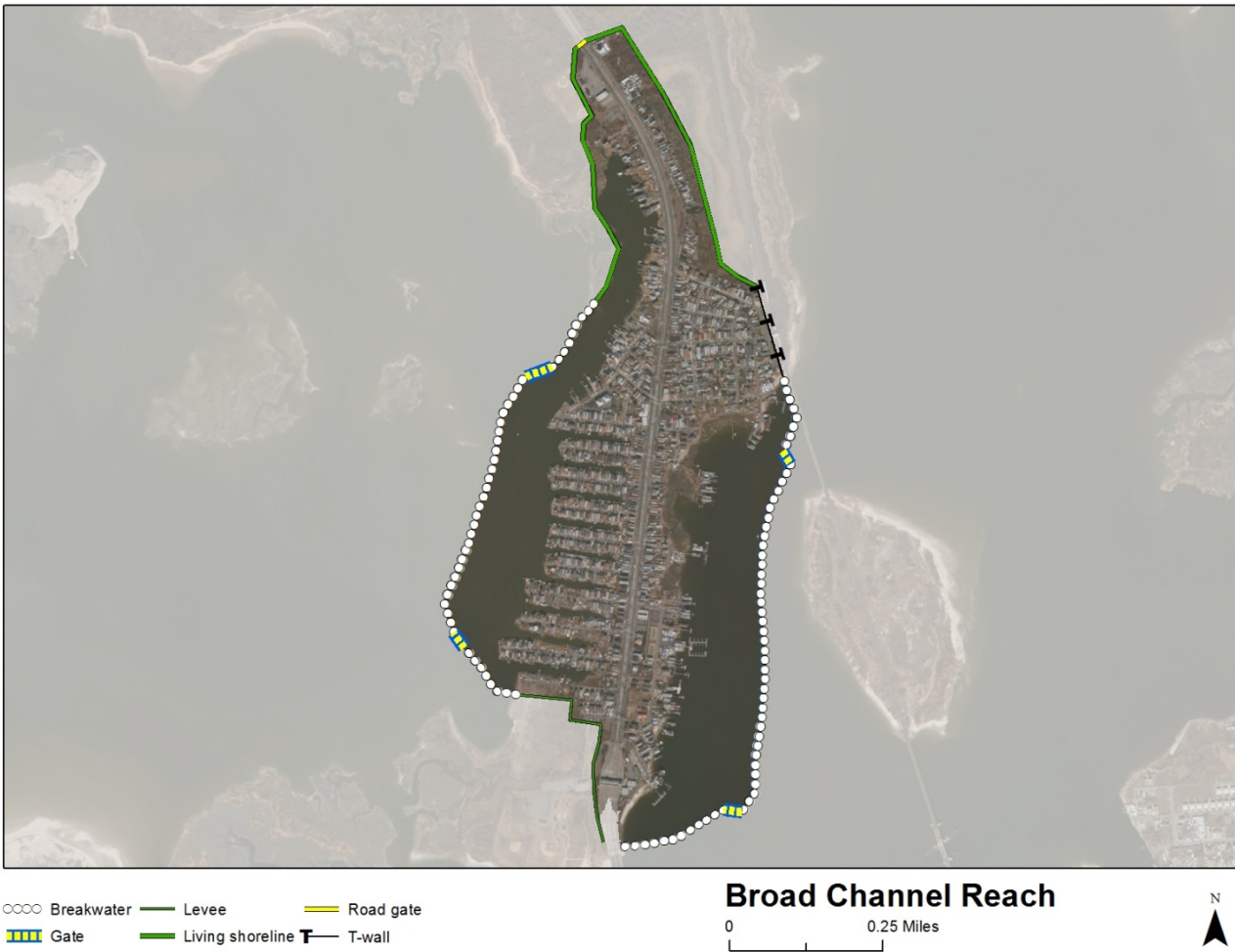
Figure 59: Plan D-6 Geographic Extent of Damage Reduction
