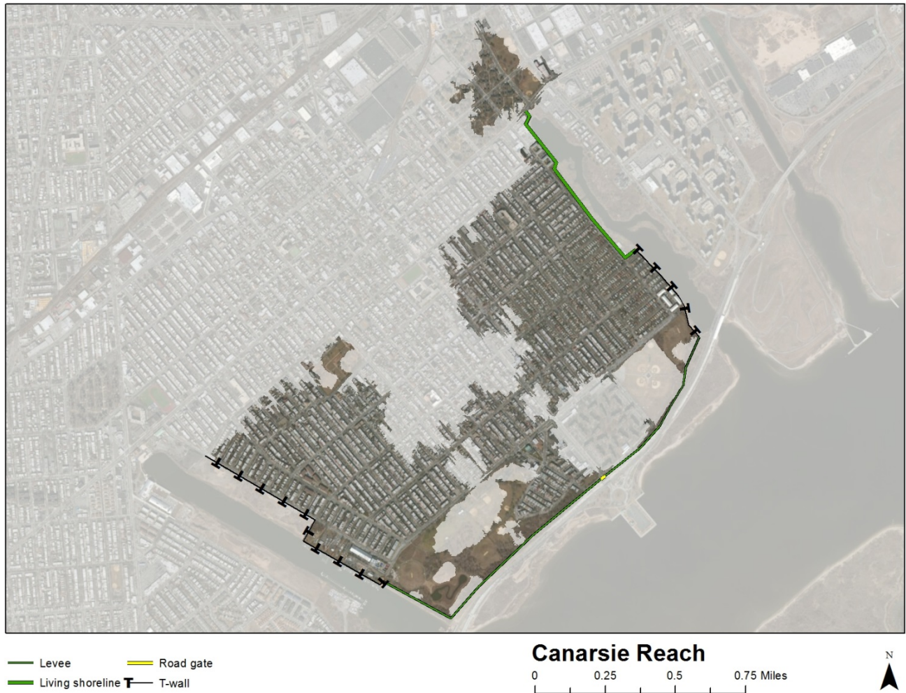
Figure 55: Plan D-2 Geographic Extent of Damage Reduction
