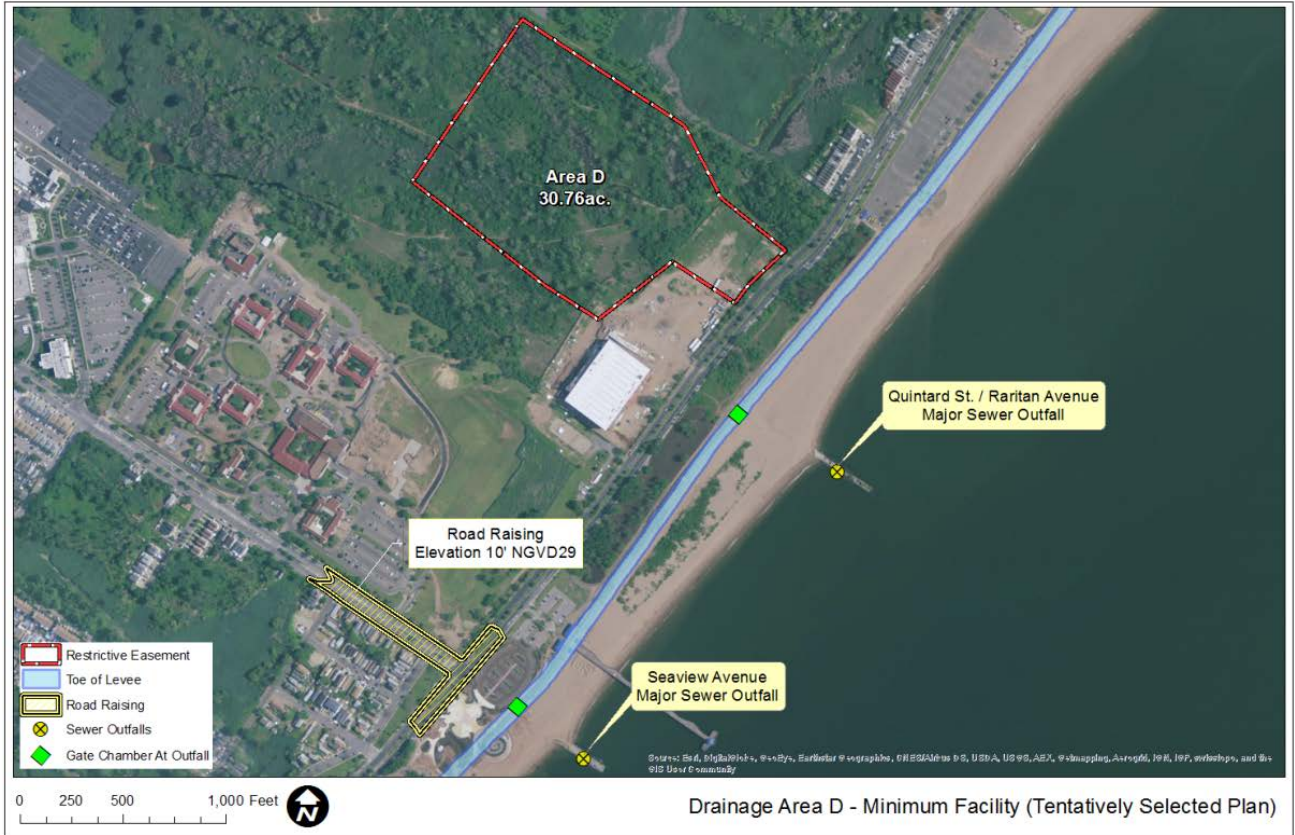
Figure 43 – Drainage Area D
