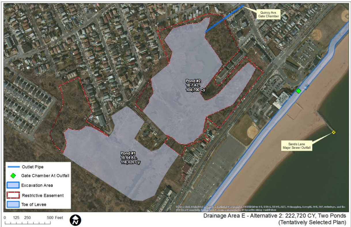
Figure 44 – Drainage Area E
