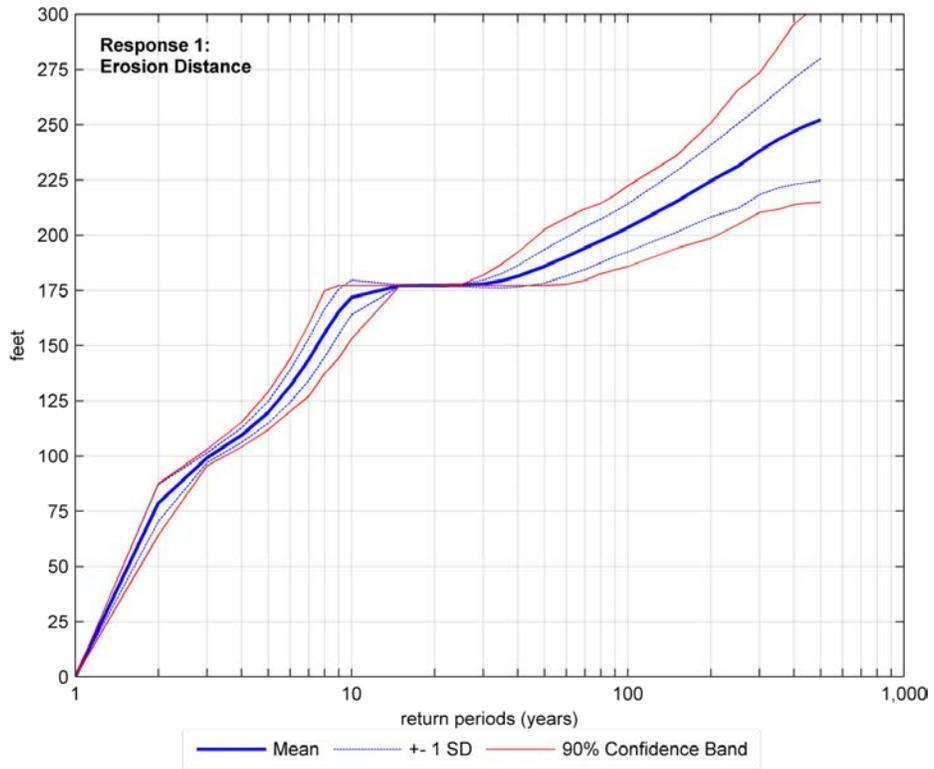
**Figure 4: Erosion distance vs. frequency for downtown Montauk**
