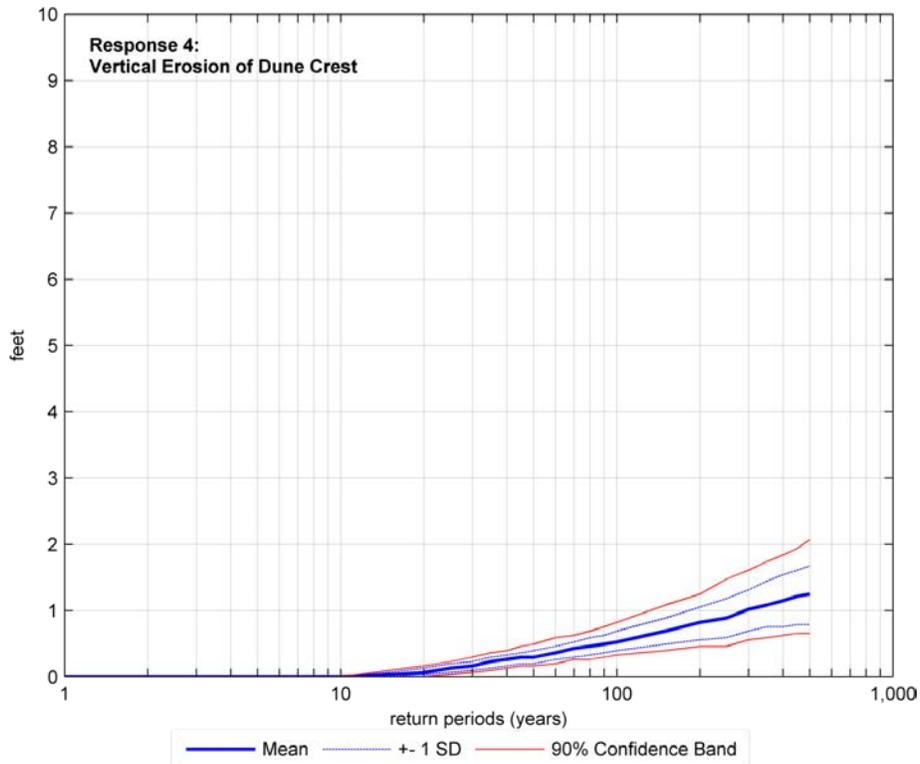
**Figure 5: Vertical erosion of dune crest vs. frequency for downtown Montauk**
