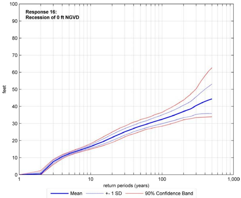
**Figure 6: Recession of 0-ft NGVD29 elevation vs. frequency for downtown Montauk**
