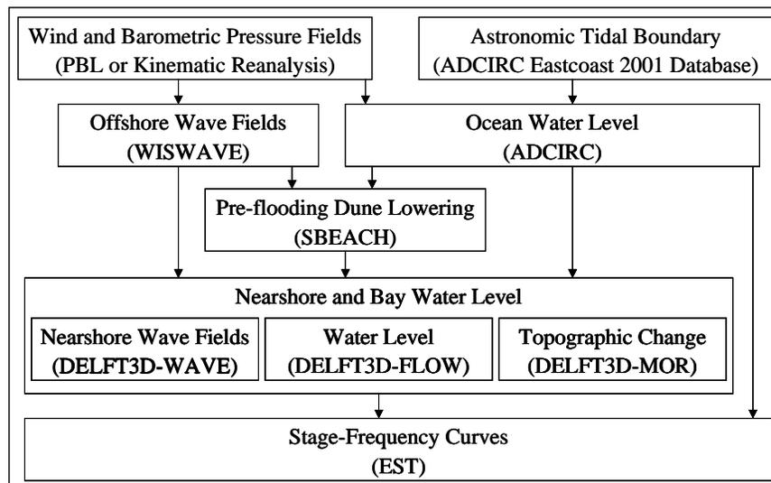
**Figure 3. FIMP storm water level modeling and stage-frequency methodology**
