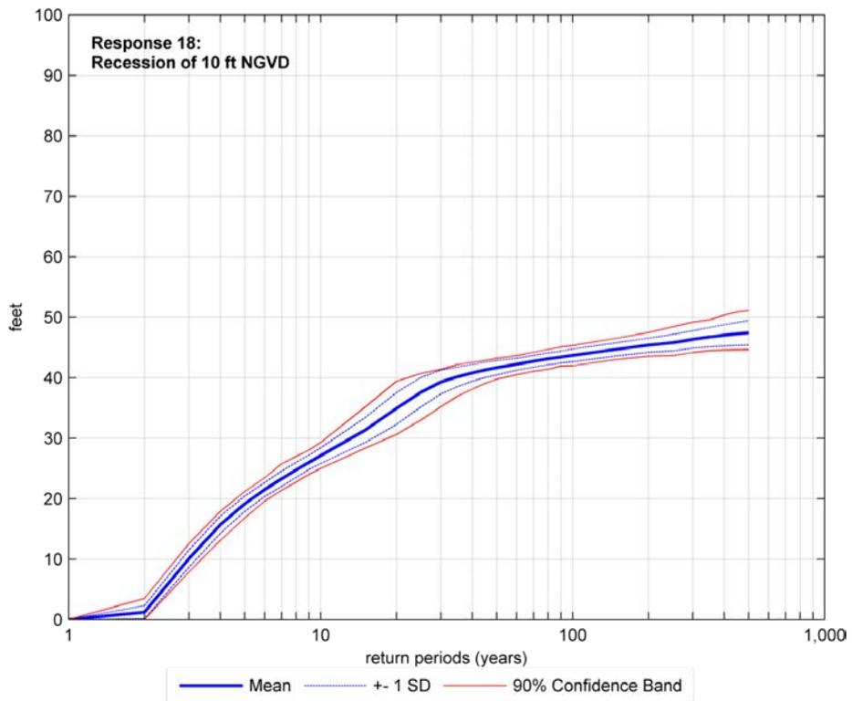
**Figure 7: Recession of 10-ft NGVD29 elevation vs. frequency for downtown Montauk**
