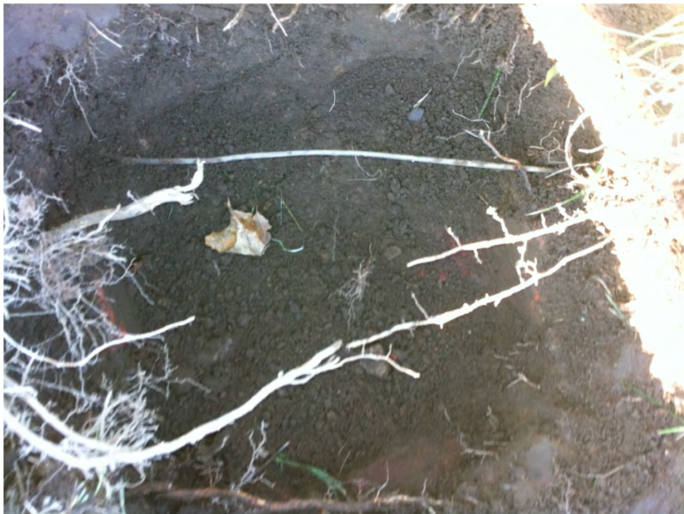
Photograph #30: 11/29/12 Area 4, Evidence of fill at hole dug at sampling location AI4-108. Wire and bricks.
