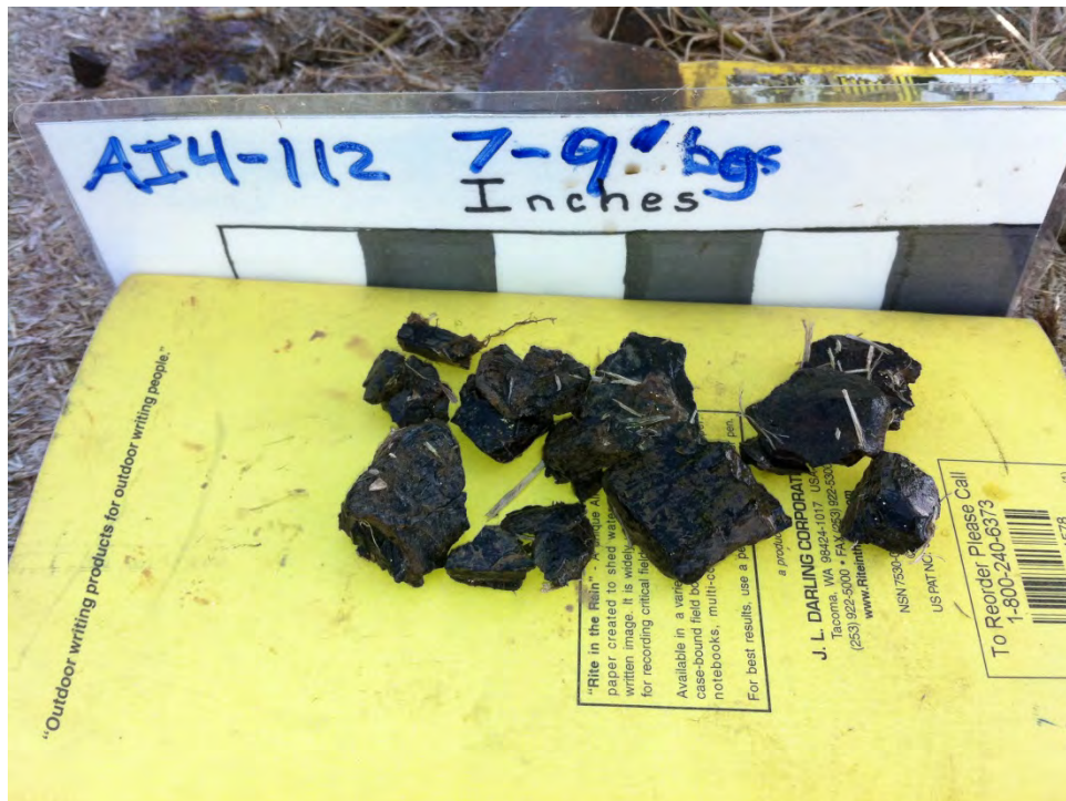
Photograph #33: 11/29/12 Area 4, Evidence of fill at hole dug at sampling location AI4-112. Coal. Glass was observed in the hole during backfilling.
