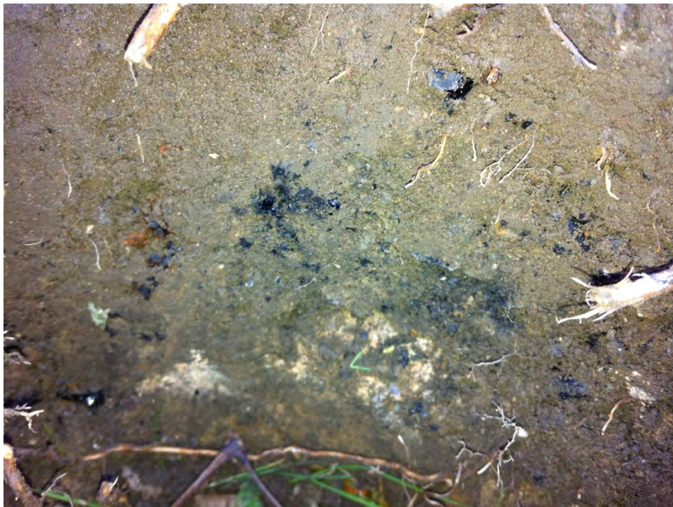
Photograph #32: 11/29/12 Area 4, Evidence of fill at hole dug at sampling location AI4-111. Coal and coal ash in hole.
