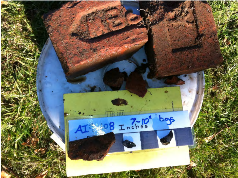
Photograph #29: 11/29/12 Area 4, Evidence of fill at hole dug at sampling location AI4-108. Bricks and coal.
