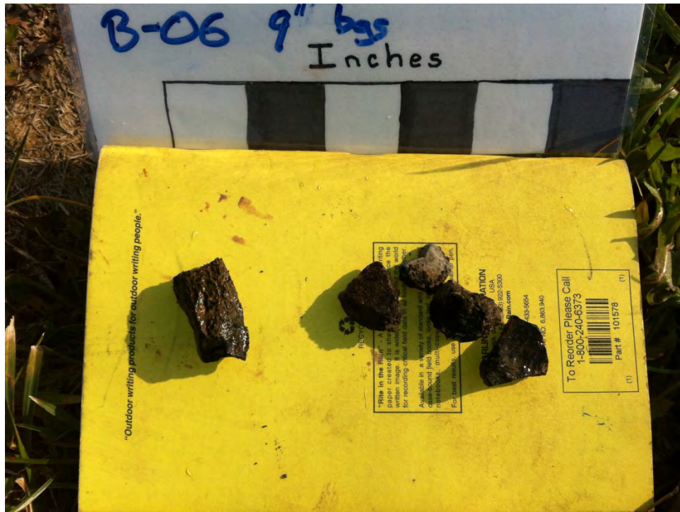
Photograph #25: 11/29/12 Area 4, Evidence of fill at hole dug at sampling location B-06. Coal and asphalt.
