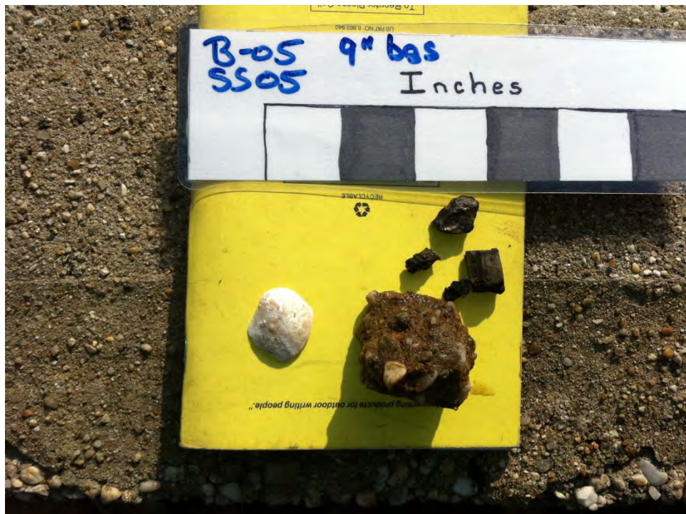
Photograph #24: 11/29/12 Area 4, Evidence of fill at hole dug at adjacent sampling locations B-05 and SS-5. Coal, concrete, and a shell.
