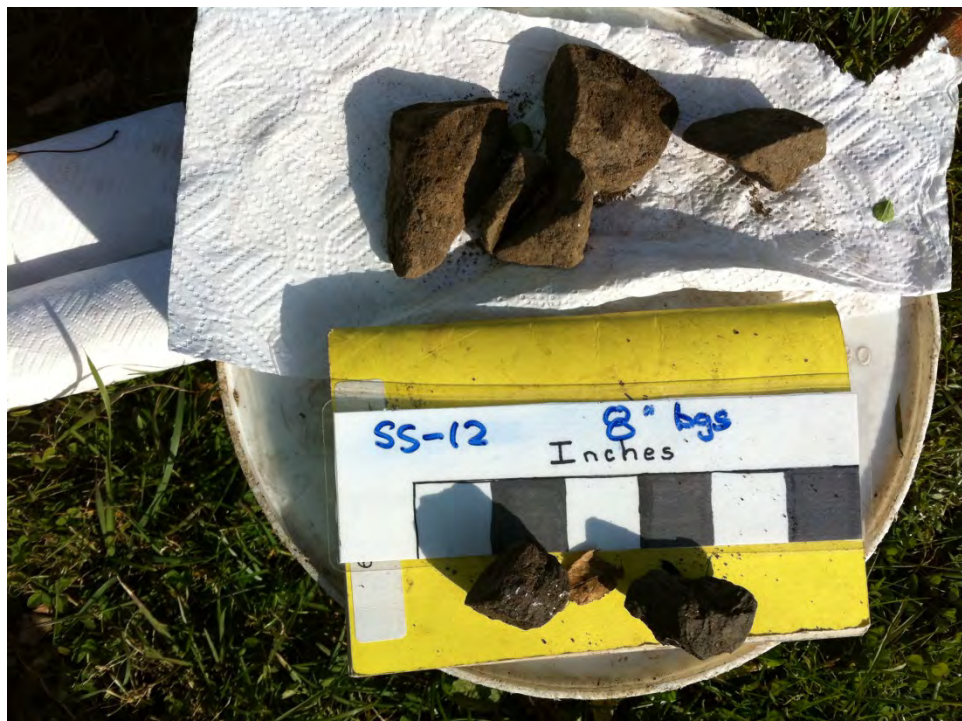
Photograph #26: 11/29/12 Area 4, Evidence of fill at hole dug at sampling location SS-12. Crushed stone up to 2-inch diameter, coal and asphalt.
