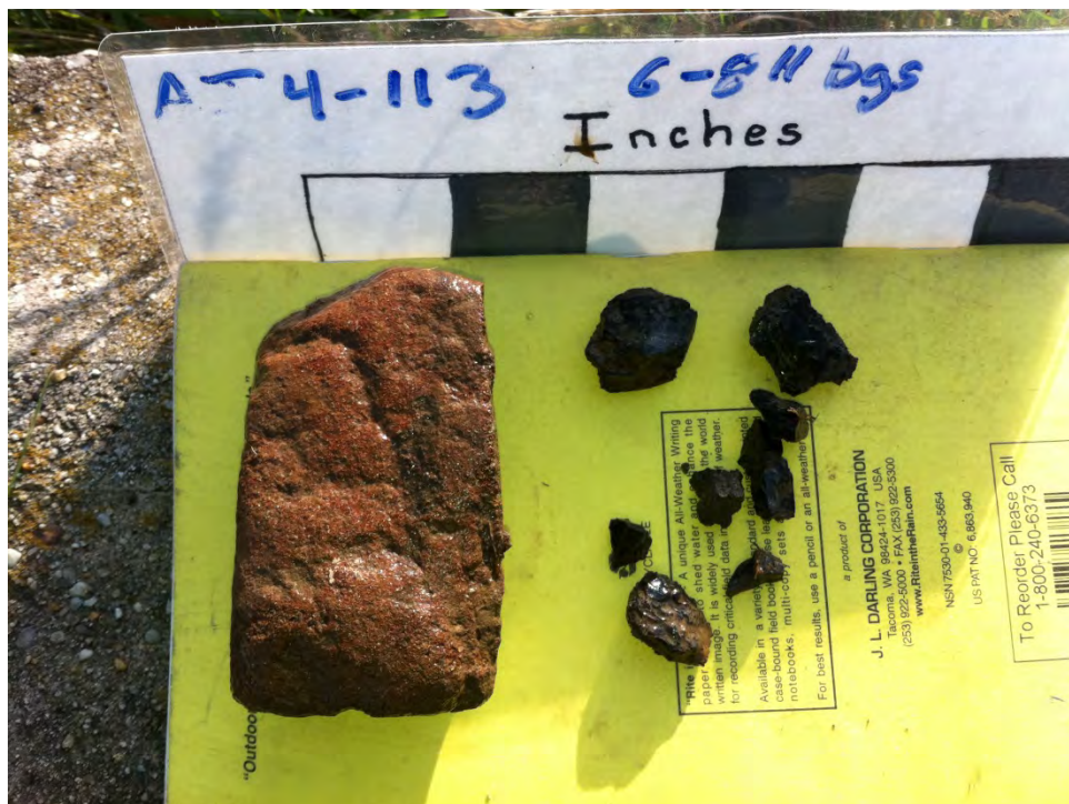
Photograph #34: 11/29/12 Area 4, Evidence of fill at hole dug at sampling location AI4-113. Coal and brick.
