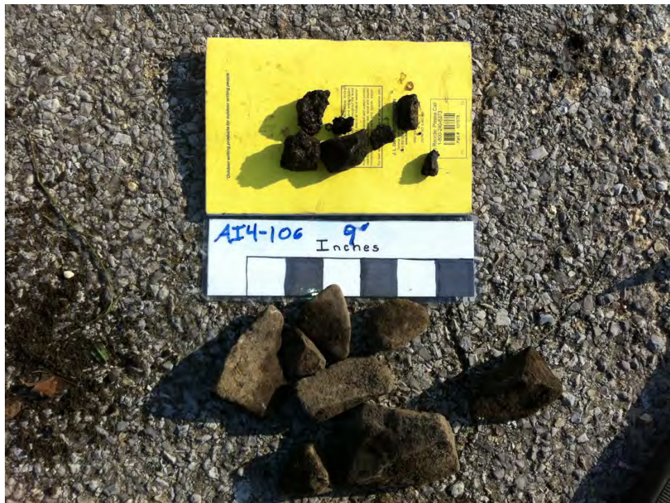
Photograph #28: 11/29/12 Area 4, Evidence of fill at hole dug at sampling location AI4-106. Crushed stone up to 2 inches in diameter, coal, and asphalt.
