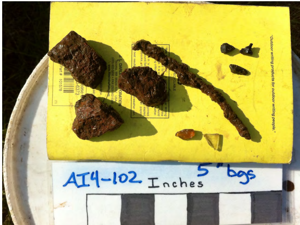
Photograph #27: 11/29/12 Area 4, Evidence of fill at hole dug at sampling location AI4-102. Coal, asphalt-coated rocks, rusty nail, and glass.
