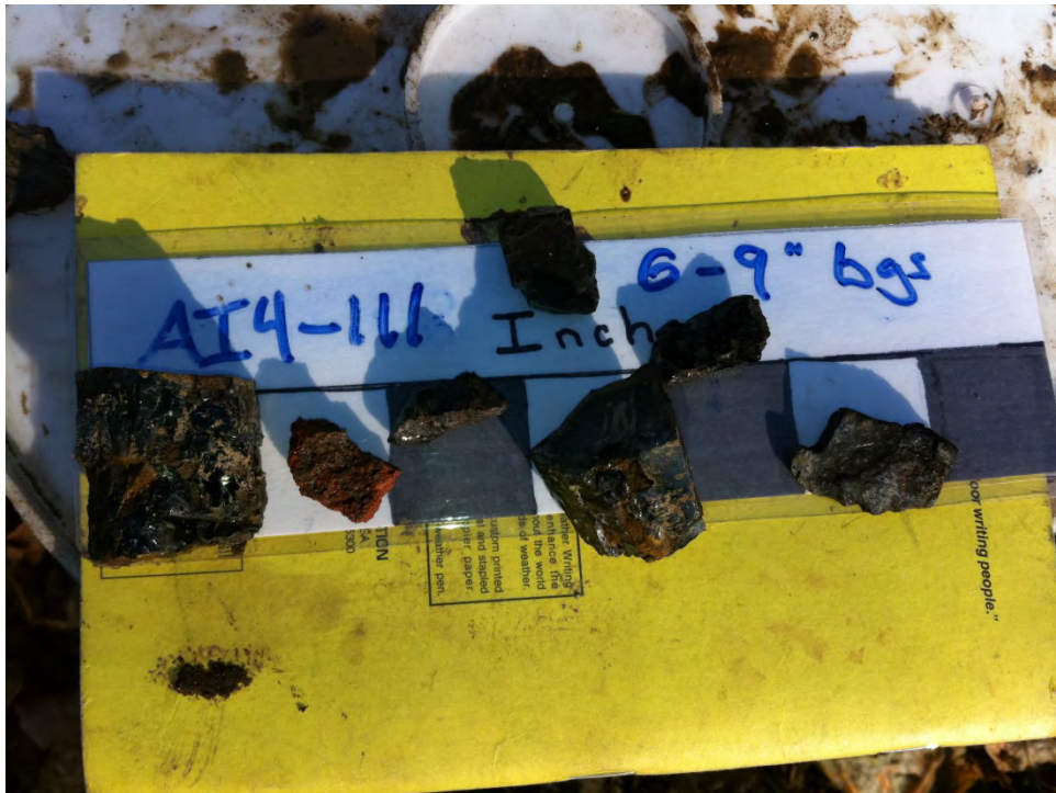
Photograph #31: 11/29/12 Area 4, Evidence of fill at hole dug at sampling location AI4-111. Coal and brick.
