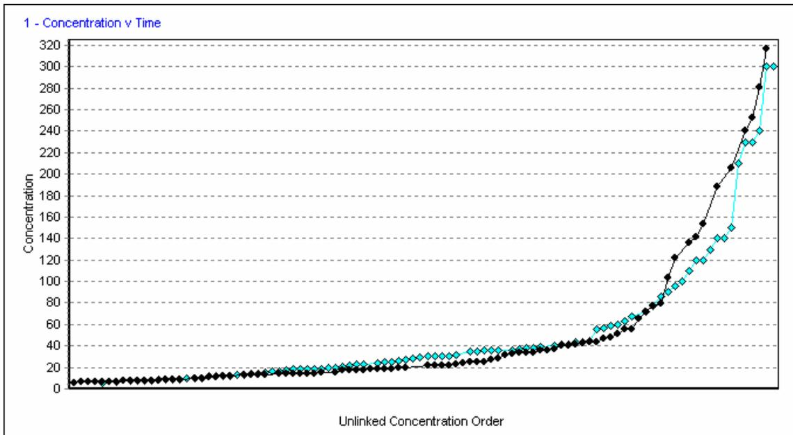
**Figure 32.** Comparison of gravimetric and acoustic estimates of TSS concentration for the entire population of 89 water samples in rank order. Gravimetric results are represented in blue, and acoustic estimates in black.
