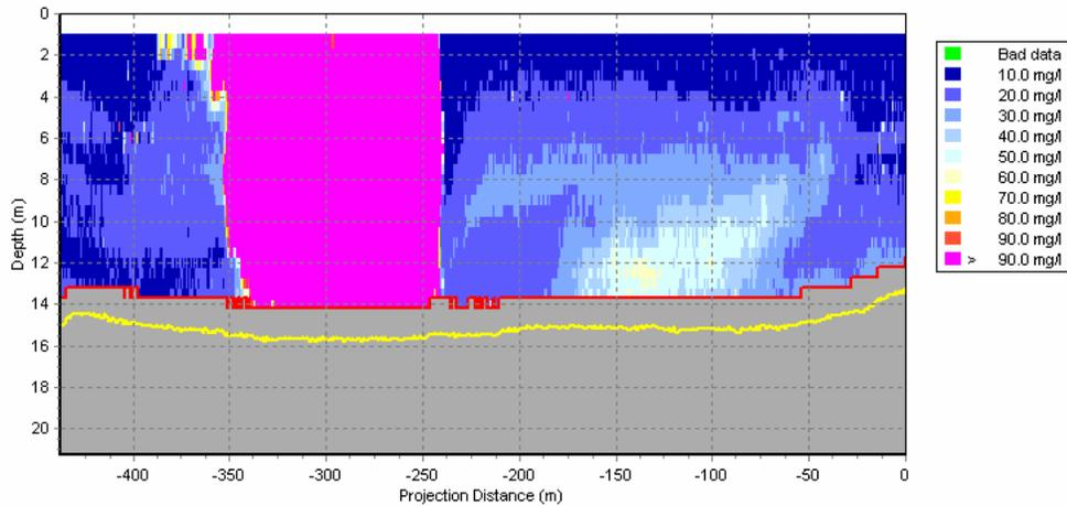
**Figure 23.** First transect directly behind the *Melbourne* (Time 0). The wake signature of the *Melbourne* is clearly visible on the left extending from the water surface to the bottom. The residual plume from the *Hudson* is still visible on the right.
