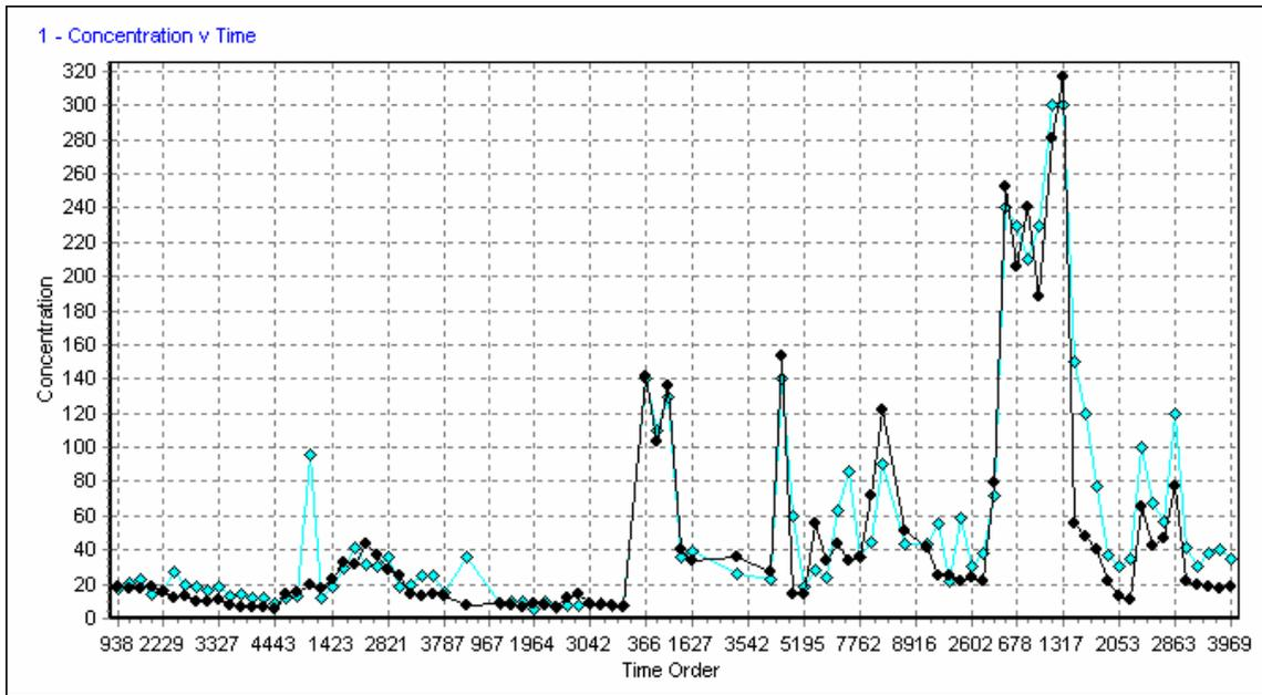
**Figure 33.** Comparison of gravimetric and acoustic estimates of TSS concentration for paired synoptic samples presented in the order of sample collection. Gravimetric results are represented in blue, and acoustic estimates in black.
