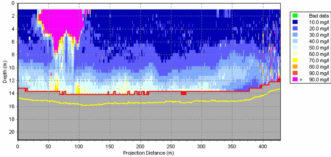
**Figure 15.** Seventh transect behind *YM North* 40 minutes after first transect with the wake signature of the tug and scow still visible on the left while the wake signature from the car carrier *ARC Freedom* has dissipated.
