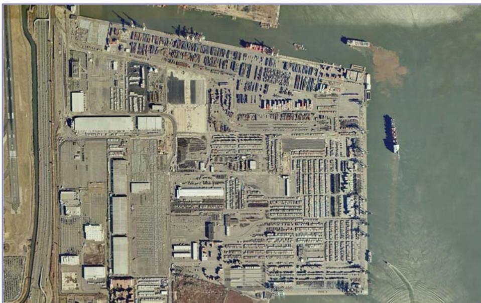
**Figure 1.** Aerial photograph of Port Elizabeth, New Jersey. Note the prominent plume behind the container ship that has entered the Elizabeth Channel stern first (at the upper right) and the container ship moving north along the eastern berthing areas (left side). An operating dredge is also visible at the entrance to the Elizabeth Channel. (Image courtesy of CHM2Hill).
