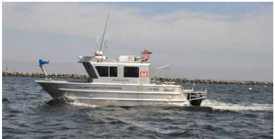
New York Survey Boat 3 conducts a hydrographic survey in Sandy Hook Bay on April 10, 2013 as part of a massive effort to map Hurricane Sandy's impacts to navigation channels throughout the region. The surveys provided updated post-Sandy data that was useful for mariners and needed for dredging efforts to restore channels impacted by Sandy to their authorized dimensions. (photo by Chris Gardner, New York District)
