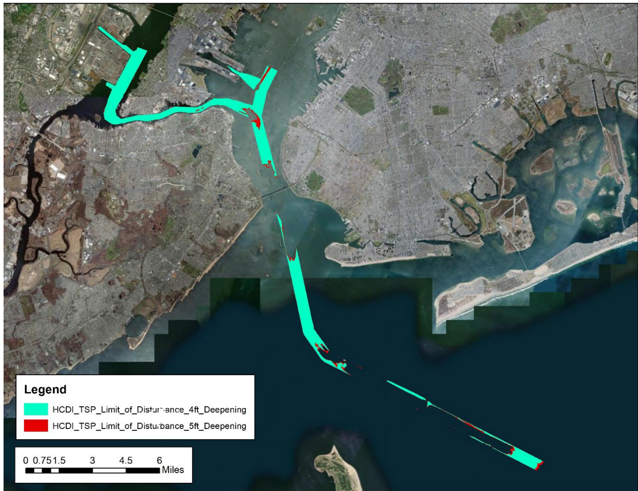
Figure 3. The Recommended Plan for the HDCI project is the 5-foot deepening. The difference in footprint of a 4-foot deepening versus a 5-foot deepening is shown here.
