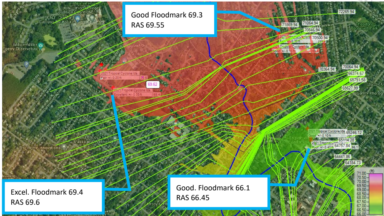
Figure 27. Comparison of peak stage to USGS surveyed floodmark during Ida at the downstream of Kenilworth gage
