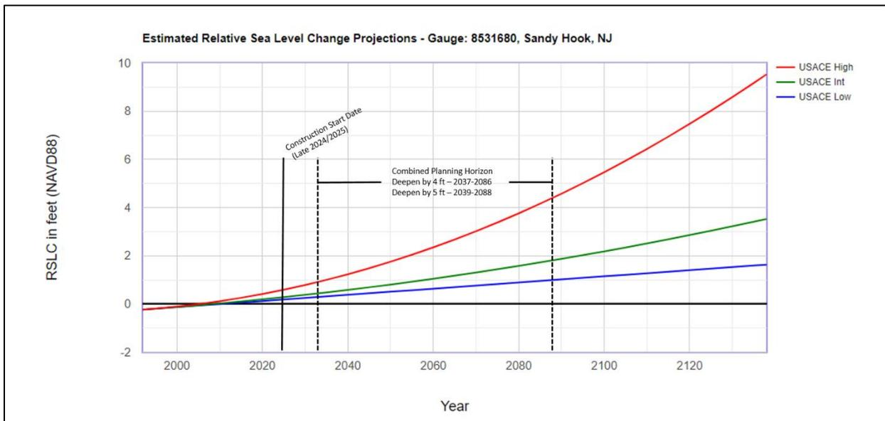
Figure 30. NOAA Gauge: Sandy Hook, NJ (#8518750) Relative Sea Level Change Projections, 1992-2138, with HDCI Construction Start Date and Planning Horizon.
