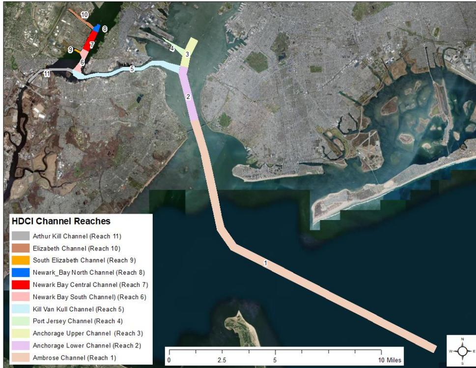
Figure 12. HDCI Reaches that are combined into Pathways
