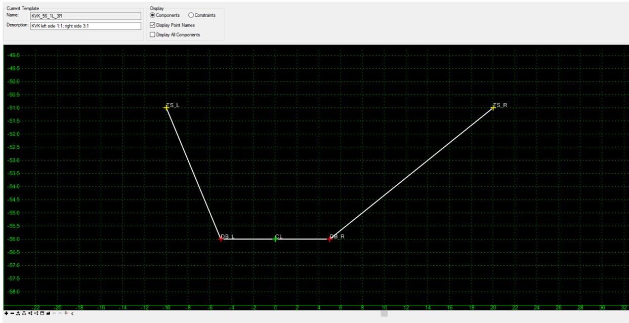
Figure 19. Sample Proposed Channel Template showing 1H: 1V Side Slope on the left; 3H: 1V Side Slope on the right
