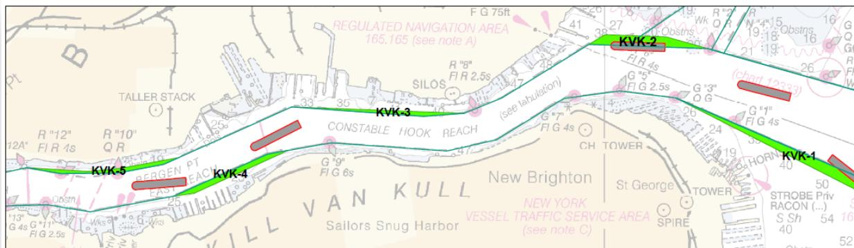
Figure 15. Areas of Widening and Efficiency (KVK-2) within the Kill Van Kull Channel (Design Ships Shown to Scale).
