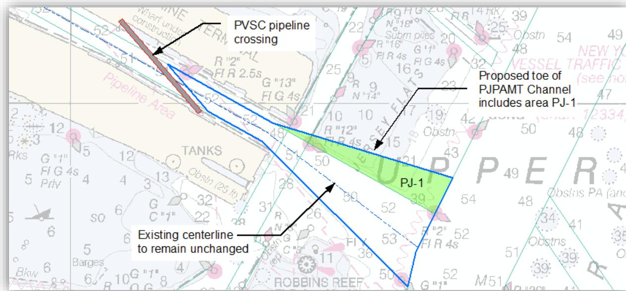
*Figure 25. The Port Jersey Channel Footprint is Changed by the Addition of Area PJ-1; the Channel Centerline Remains Unchanged.*
