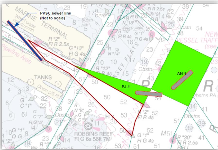
Figure 14. Port Jersey Channel, Showing Location of PVSC Trunk Line as it Crosses the Channel, Area PJ-1 and Area AN-1. (Design Ships are Shown to-Scale.)
