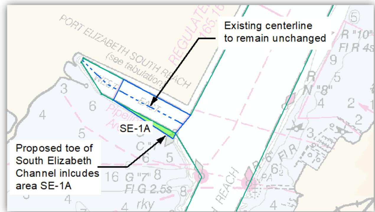
Figure 28. The Footprint of South Elizabeth Channel is Changed by the Addition of Area SE-1A; the Channel Centerline Remains Unchanged.
