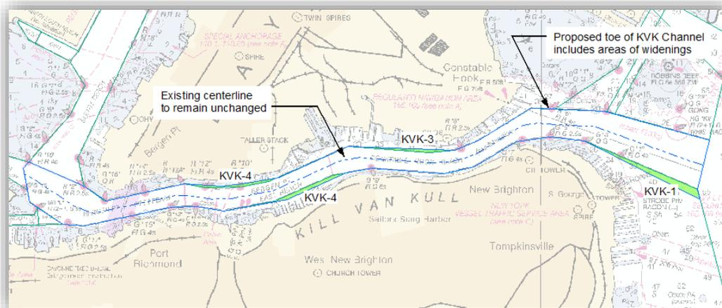
Figure 26. The KVK Channel Footprint is Changed by the Addition of Areas KVK-1, KVK-3, KVK-4, KVK-5; the Channel Centerline Remains Unchanged.
