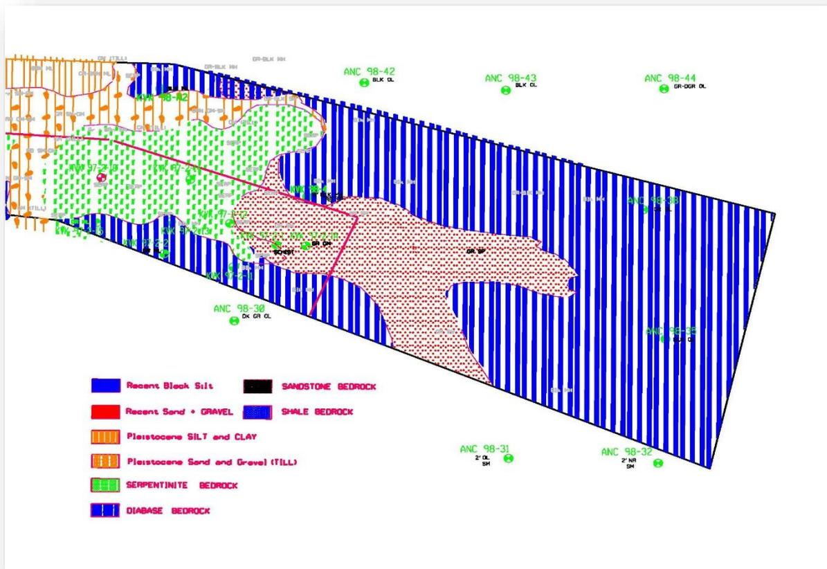
Figure 23. Sample File Showing Material Types in the vicinity of the Eastern Kill Van Kull Channel
