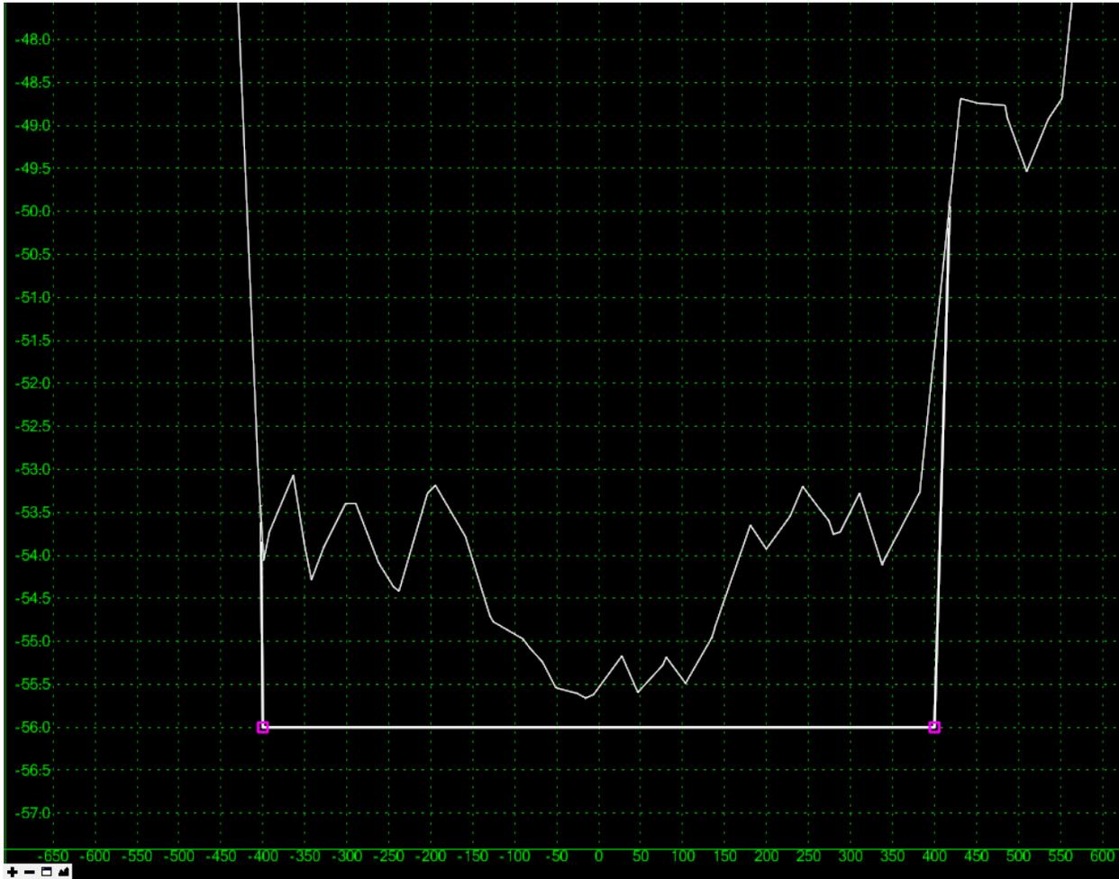
Figure 20. Proposed Channel Template being "pushed" through Existing Conditions Surface
