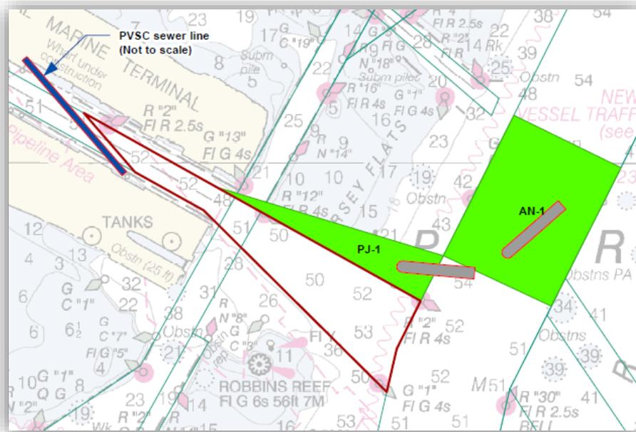
Figure 14. Port Jersey Channel, Showing Location of PVSC Trunk Line as it Crosses the Channel, Area PJ-1 and Area AN-1. (Design Ships are Shown to-Scale.)
