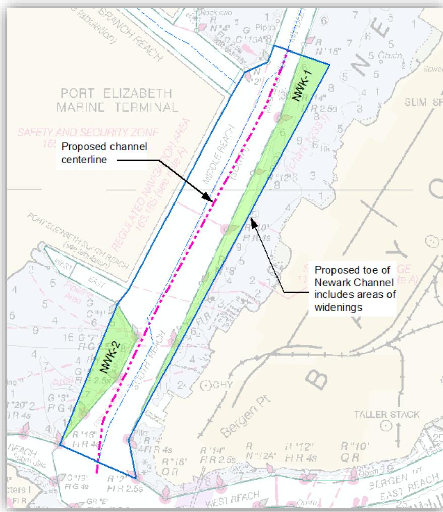
Figure 27. The Newark Bay Channel Footprint is changed by the Addition of Areas NWK-1 and NWK-2. The Proposed Channel Line is shown.
