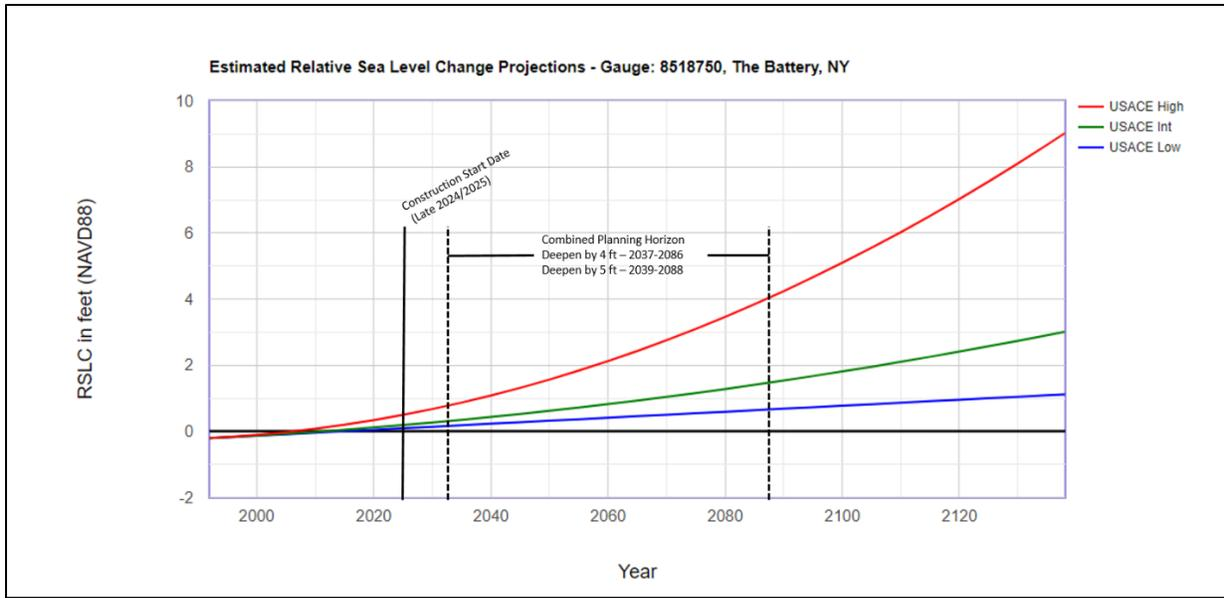
Figure 29. NOAA Gauge: The Battery, NY (#8518750) Relative Sea Level Change Projections, 1992-2138, with HDCI Construction Start Date and Planning Horizon.
