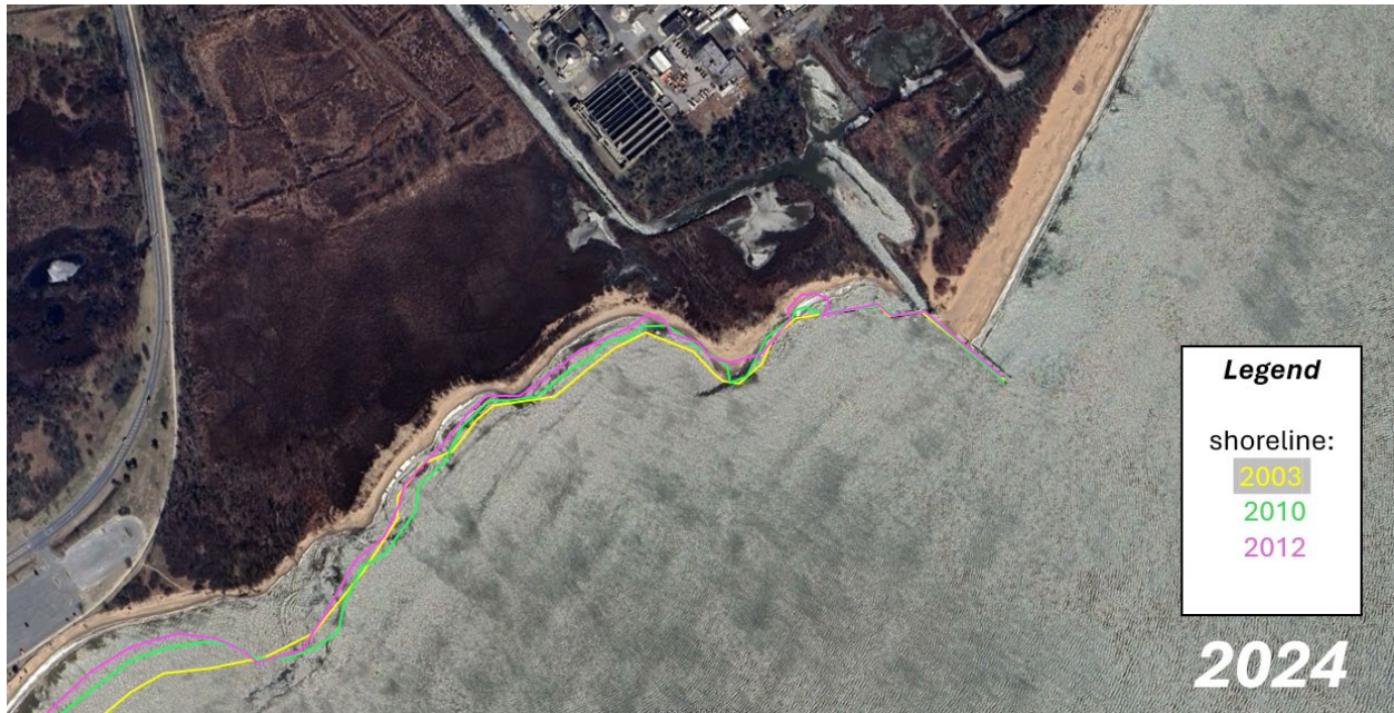
Figure 17: Observations of shoreline erosion via satellite imagery (Google Earth, n.d.)
