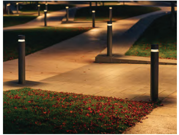
Illuminate paths as close to the ground as possible with shielded amber or red lights.
