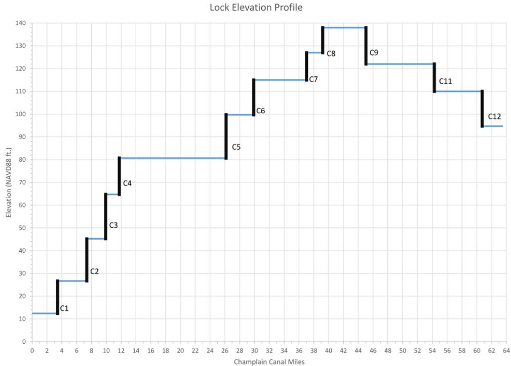
**Figure 4. Champlain Canal Lock Elevation Profile**
