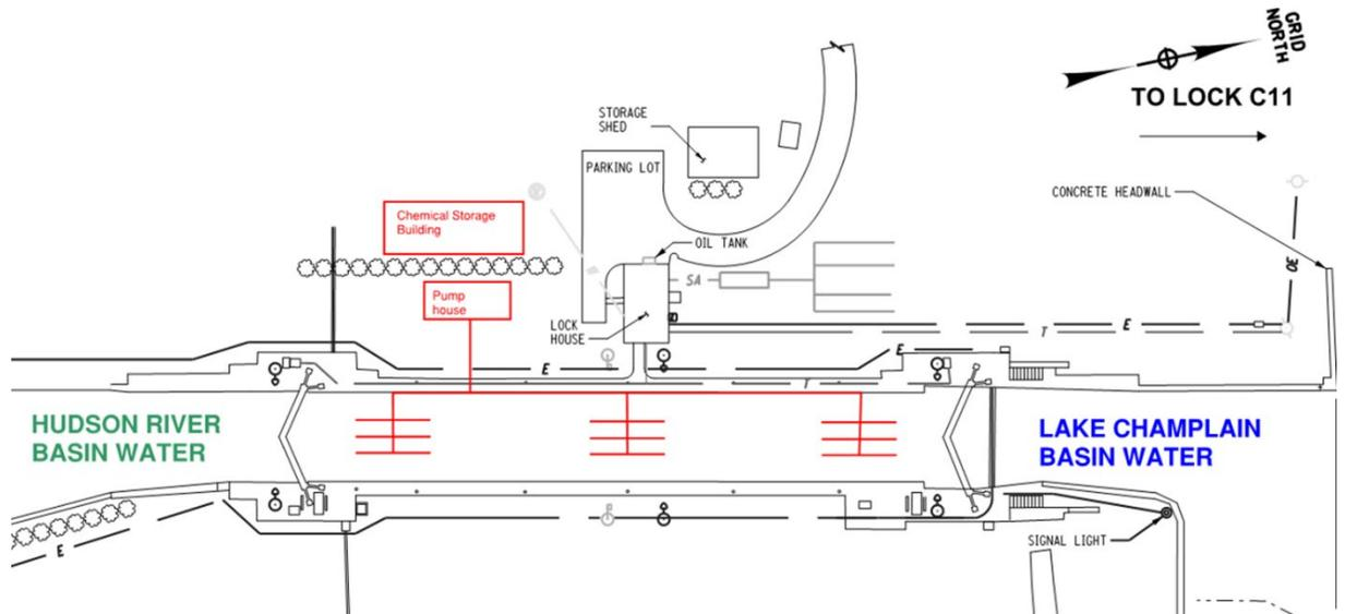
**Figure 18. Chlorination Treatment Chamber Layout at Lock C9.**
