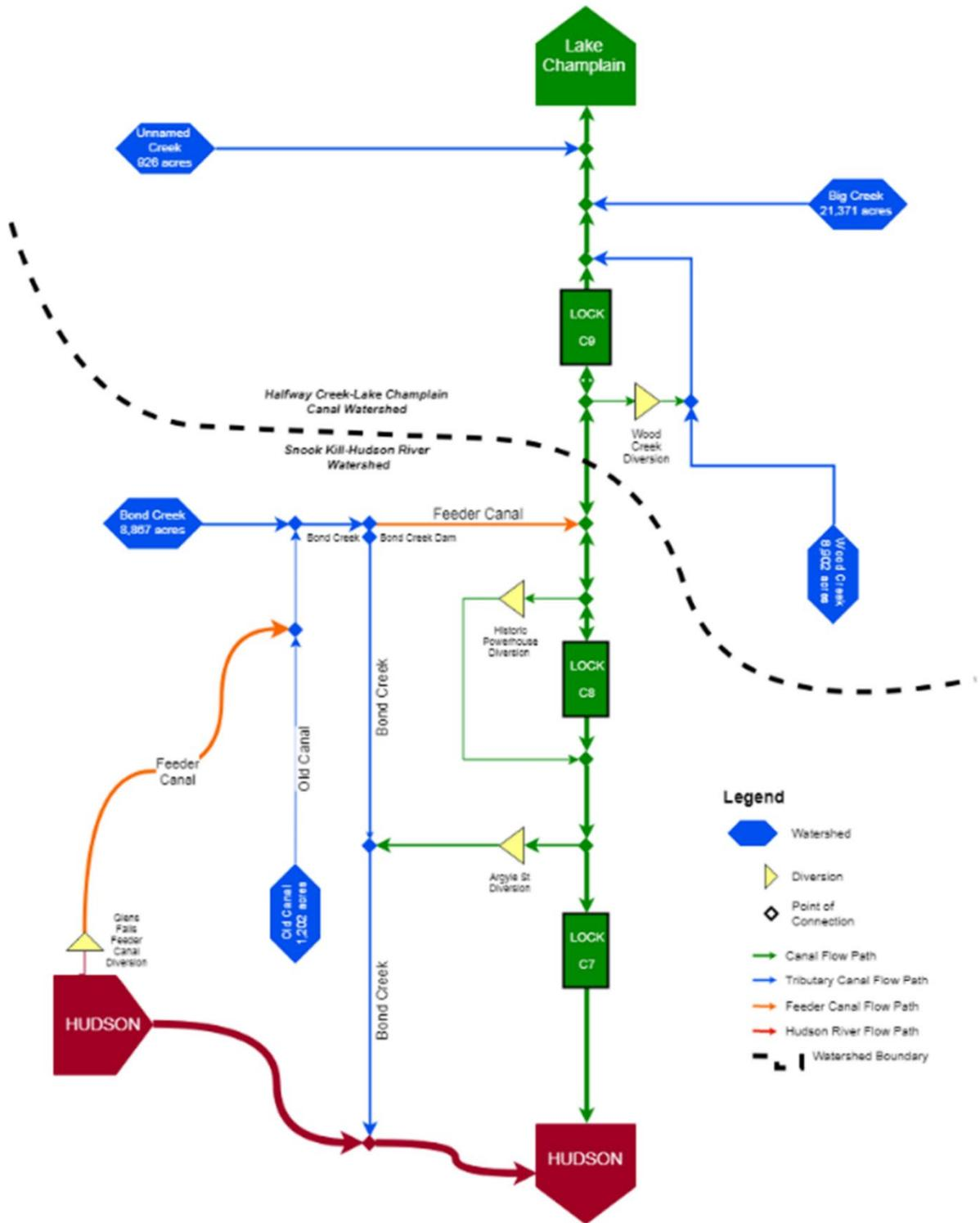
Figure 7. Champlain Canal Schematic (Locks C7-C9)
