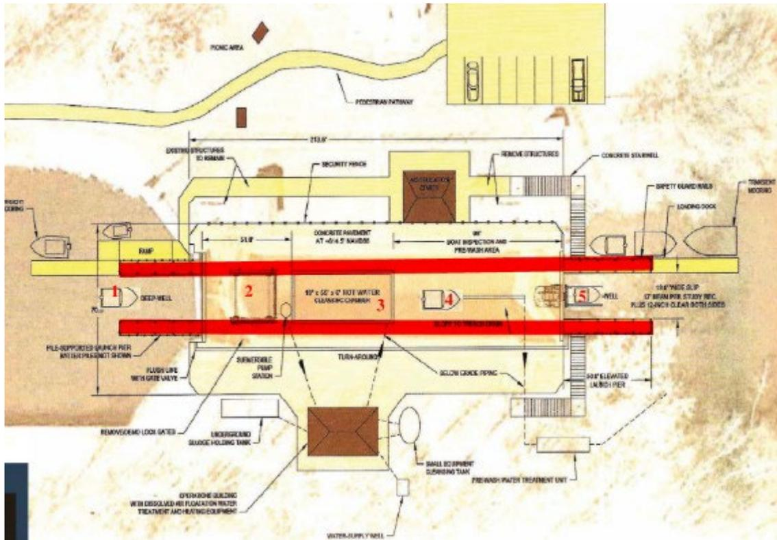
**Figure 12. Boat Cleaning Station for Small Vessels – Conceptual Plan**
