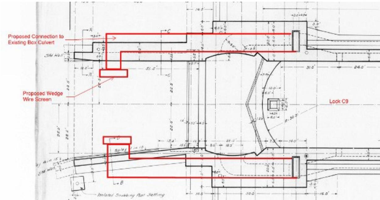
**Figure 14. Lock Feedwater with Wedge Wire Screen – Conceptual Plan**
