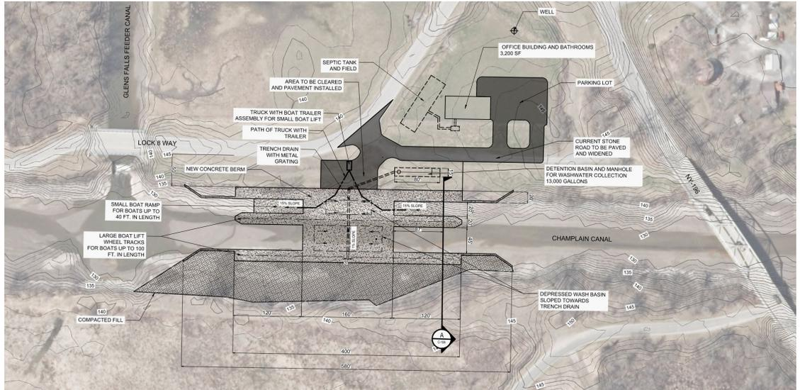
Figure 1. Alternative 2 General Layout Plan.
