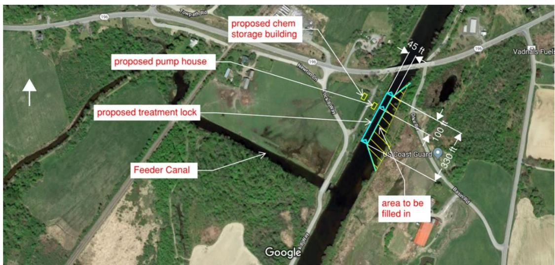
**Figure 19. New Chlorination Treatment Chamber at Route 196.**
