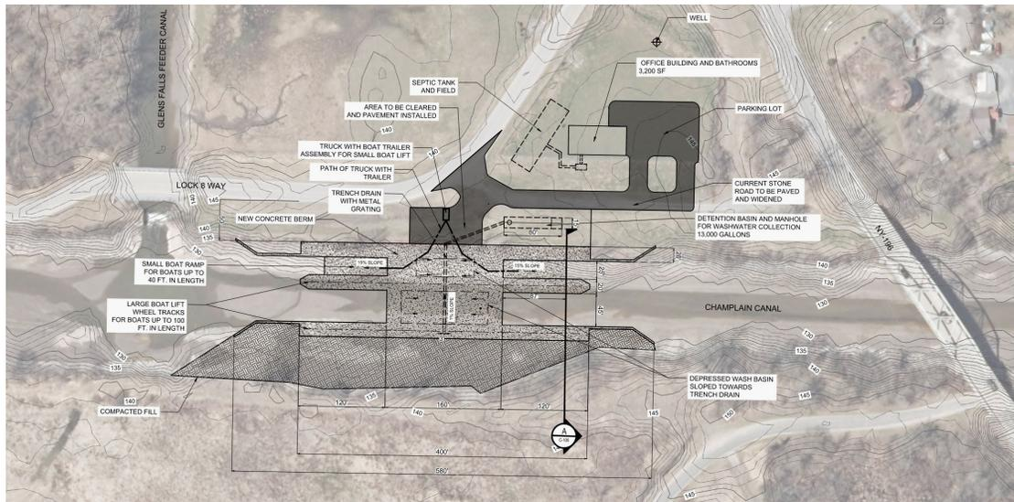
**Figure 22. Alternative 2 General Layout Plan.**
