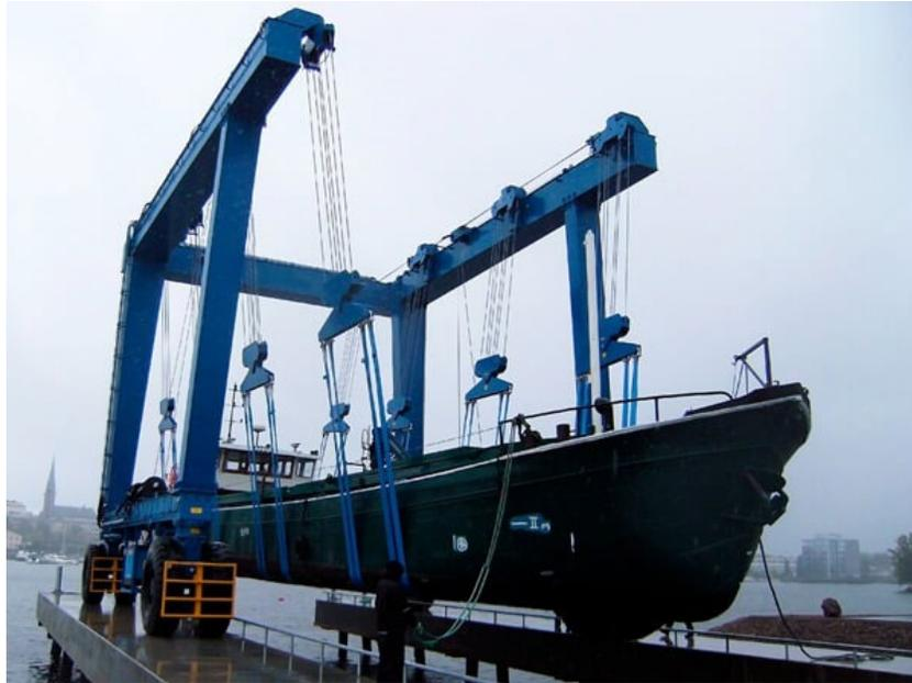
**Figure 11. Example Marine Boat Lift System for Small/Medium Vessels**
