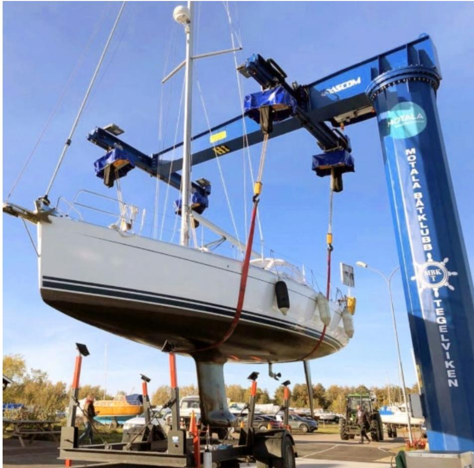
**Figure 13: Small Vessel Boat Lift via Cantilever Arm**
