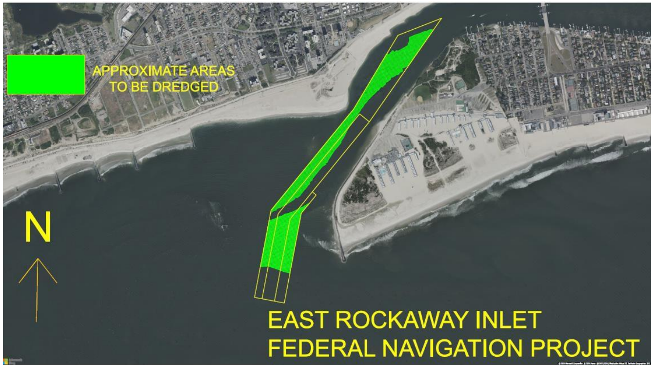
Figure 1: East Rockaway Inlet, approximate locations of dredging areas shown.
