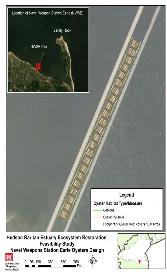
Restoration of 10 acres using Gabions and Oyster Pyramids
