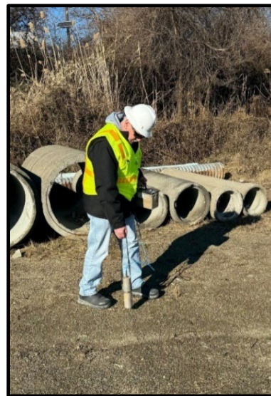
Ground surveys will be performed using handheld gamma detectors.
