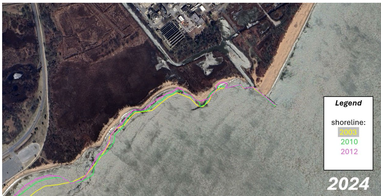
Figure 11: Observations of shoreline erosion via satellite imagery (Google Earth, n.d.)
