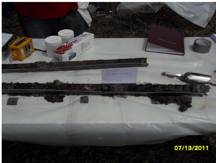
Soil core from SB-006
