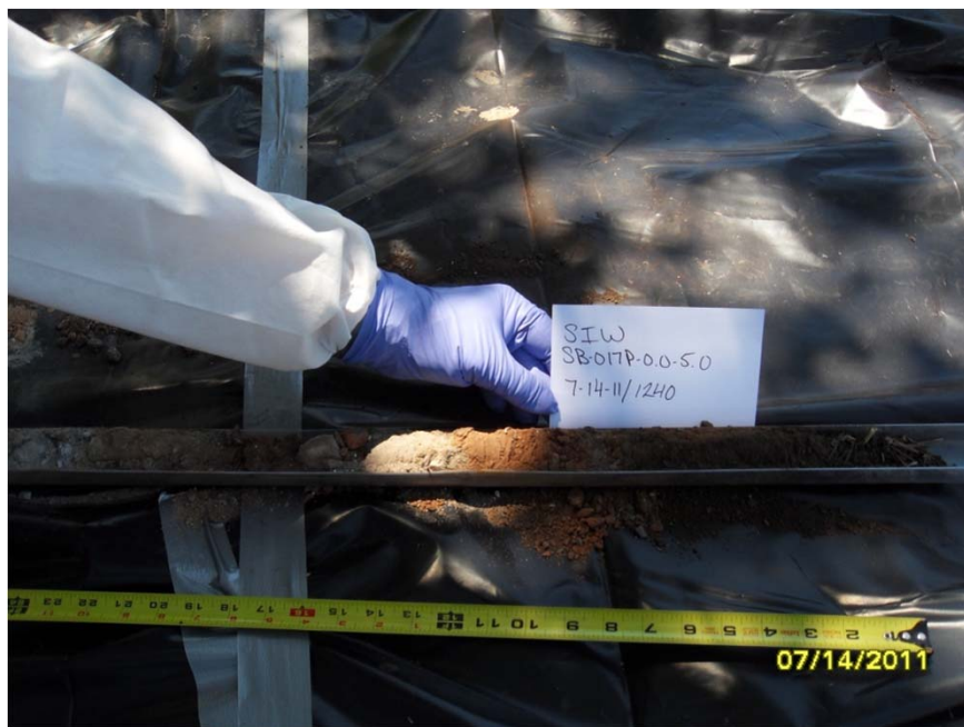
Soil core from SB-017
