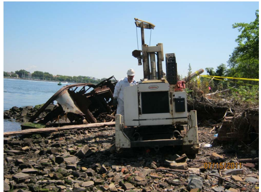
Subsurface sample collection on beach
