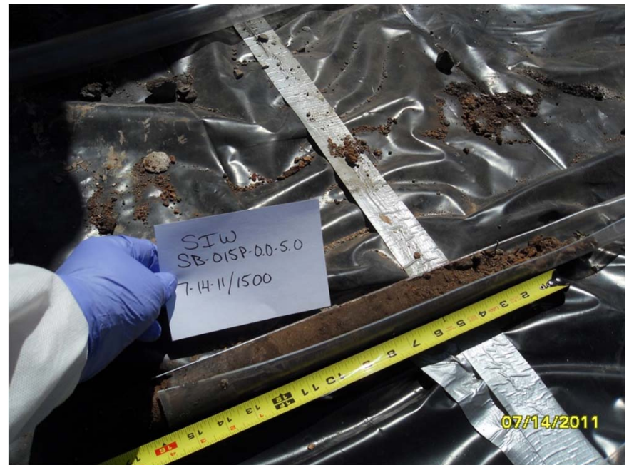
Soil core from SB-015
