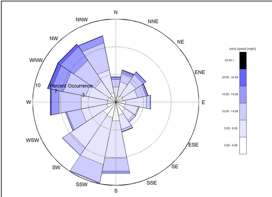
**Figure 2-1: Wind Rose Plot of Resultant Wind Speed and Direction for JFK International Airport Wind Data (1984 to Present).**
