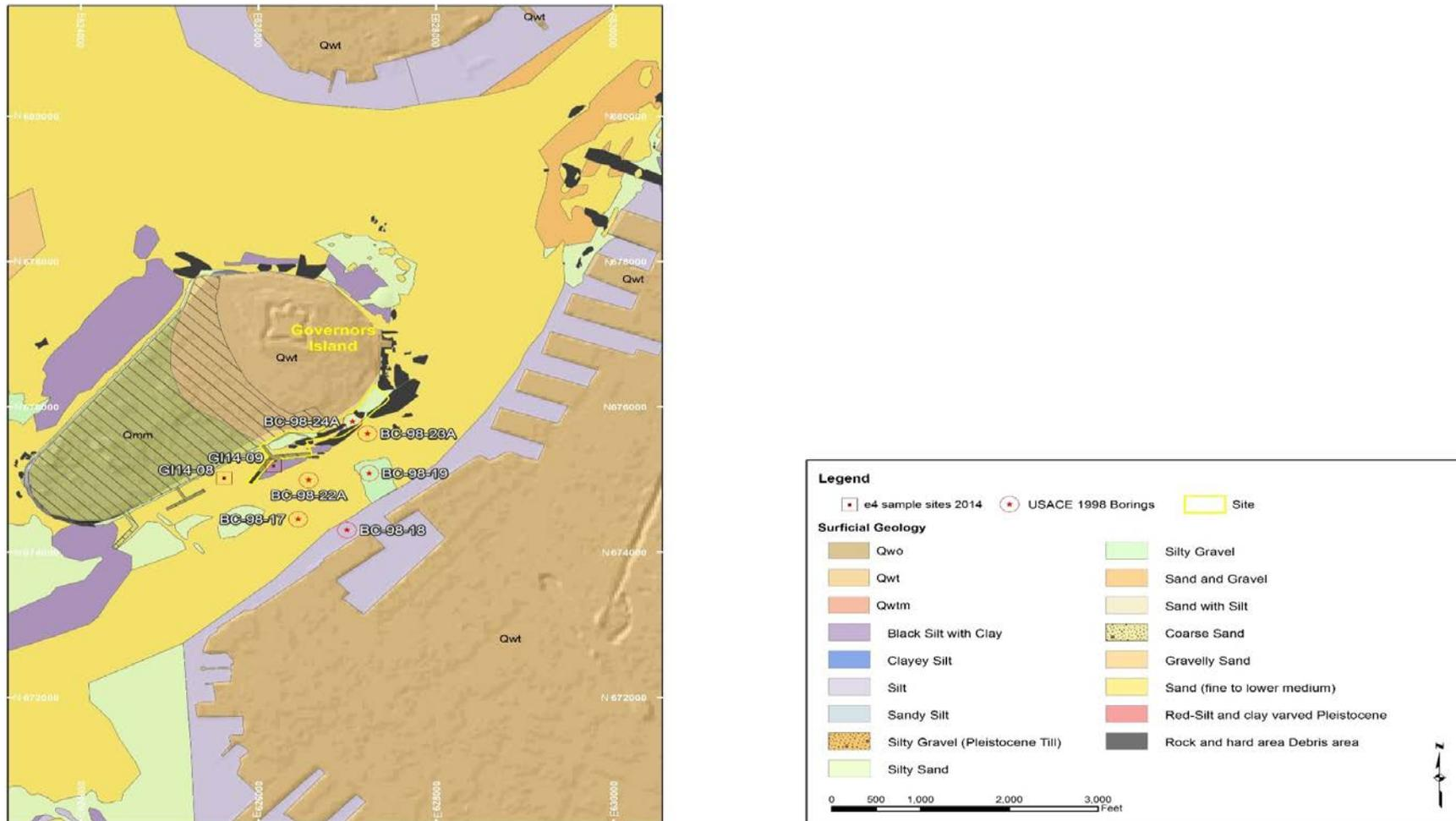
**Figure 2-25: Surficial geology and boring locations of the Governors Island site.**
