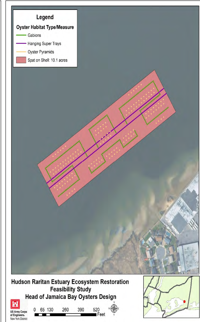
Restoration of 10.1 acres using Gabions, Hanging Super Trays, Oyster Pyramids and Spat on Shell
