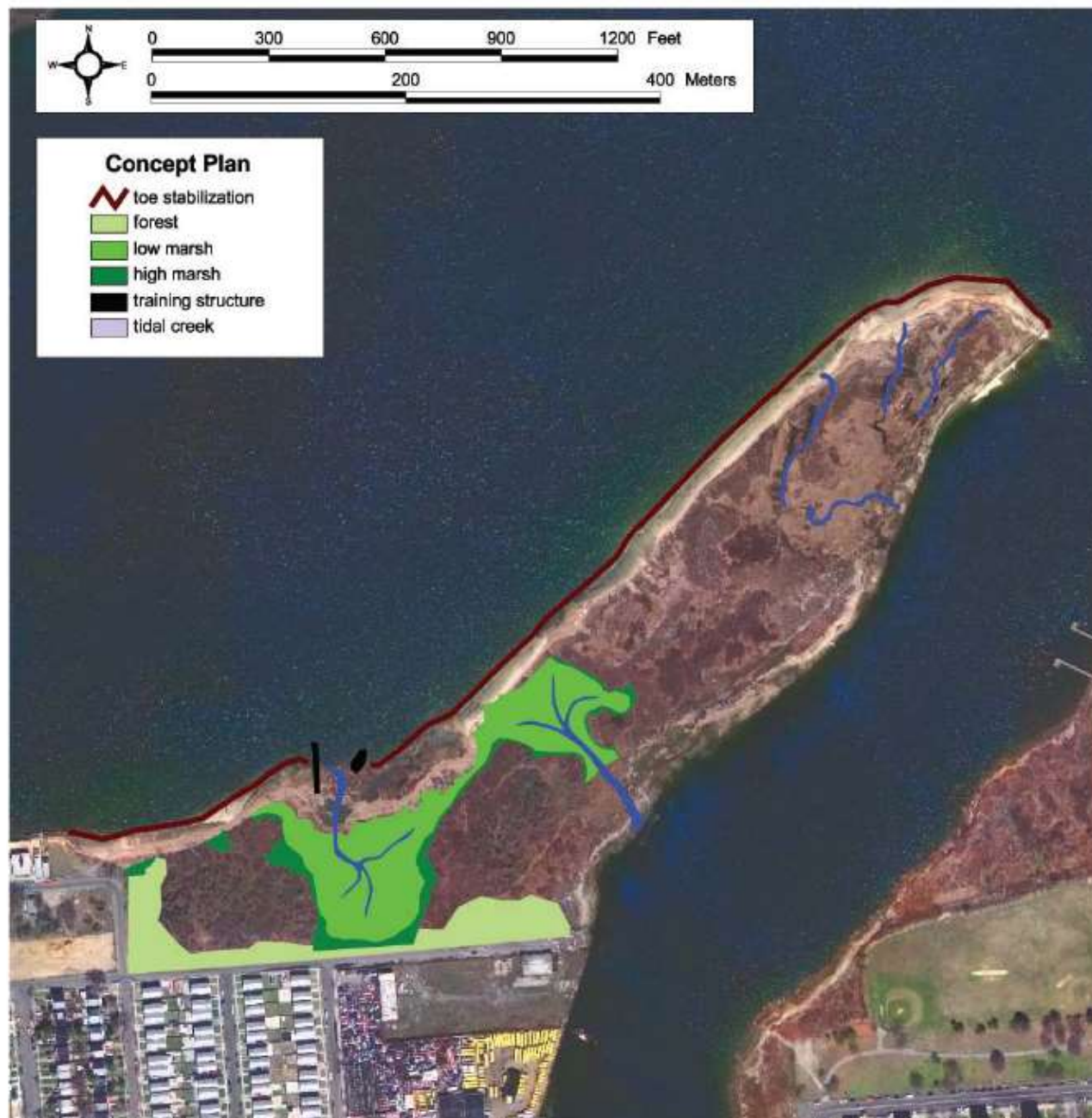
Figure D2-26. Dubos Point Alternatives 1, 2 and 3 (Difference is in the amount of toe stabilization under consideration)
