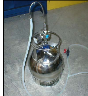
Figure 4 - Vapor intrusion studies were conducted at several buildings in which sub-slab soil gas and indoor air were sampled for the presence of VOCs to determine if vapor from groundwater was entering buildings.
