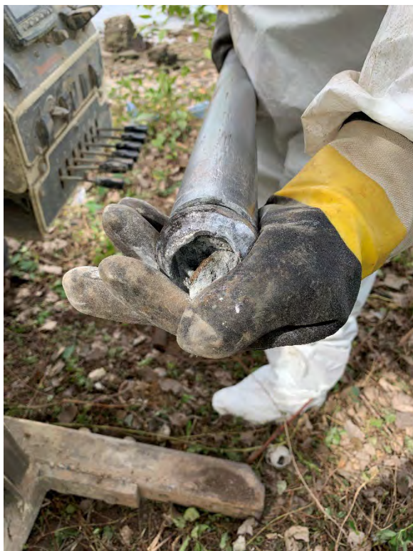
Broken macro core barrel (SB-04, at 4-feet bgs)
