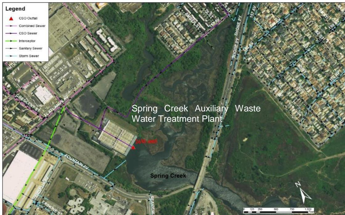
**Figure 3. Spring Creek Auxiliary Waste Water Treatment Plant and Sewer Line Alignment**
