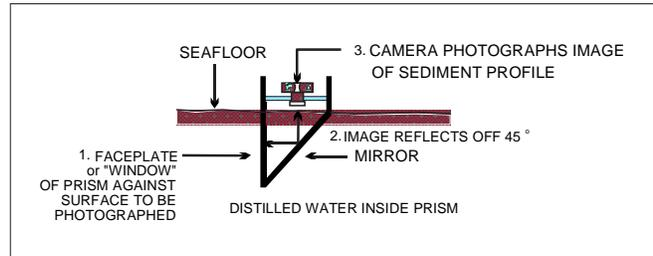
**Figure 2.4-1.** Schematic diagram of Benthos, Inc. Model 3731 REMOTS® (and Ocean Imaging Systems digital head) sediment-profile camera and sequence of operation on deployment. The image in the upper left shows the sediment-profile camera with plan-view camera attached.
