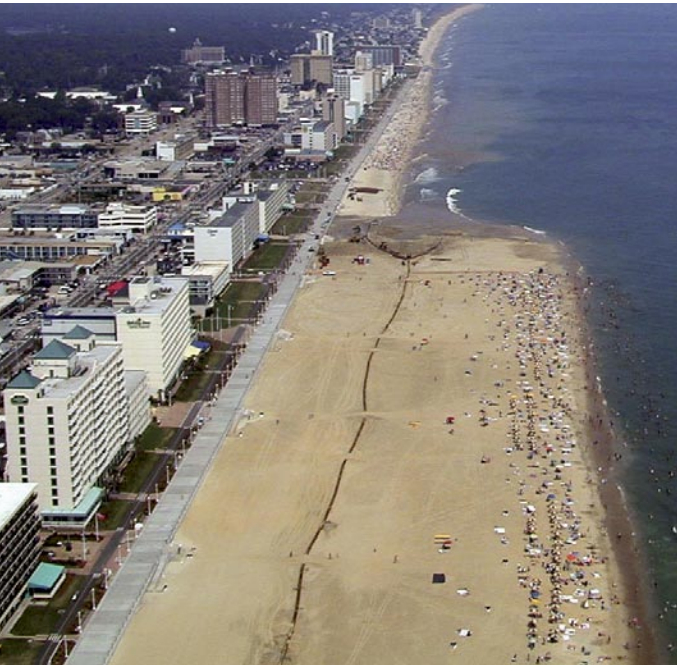
This beach nourishment project is under construction at Virginia Beach, Va.
