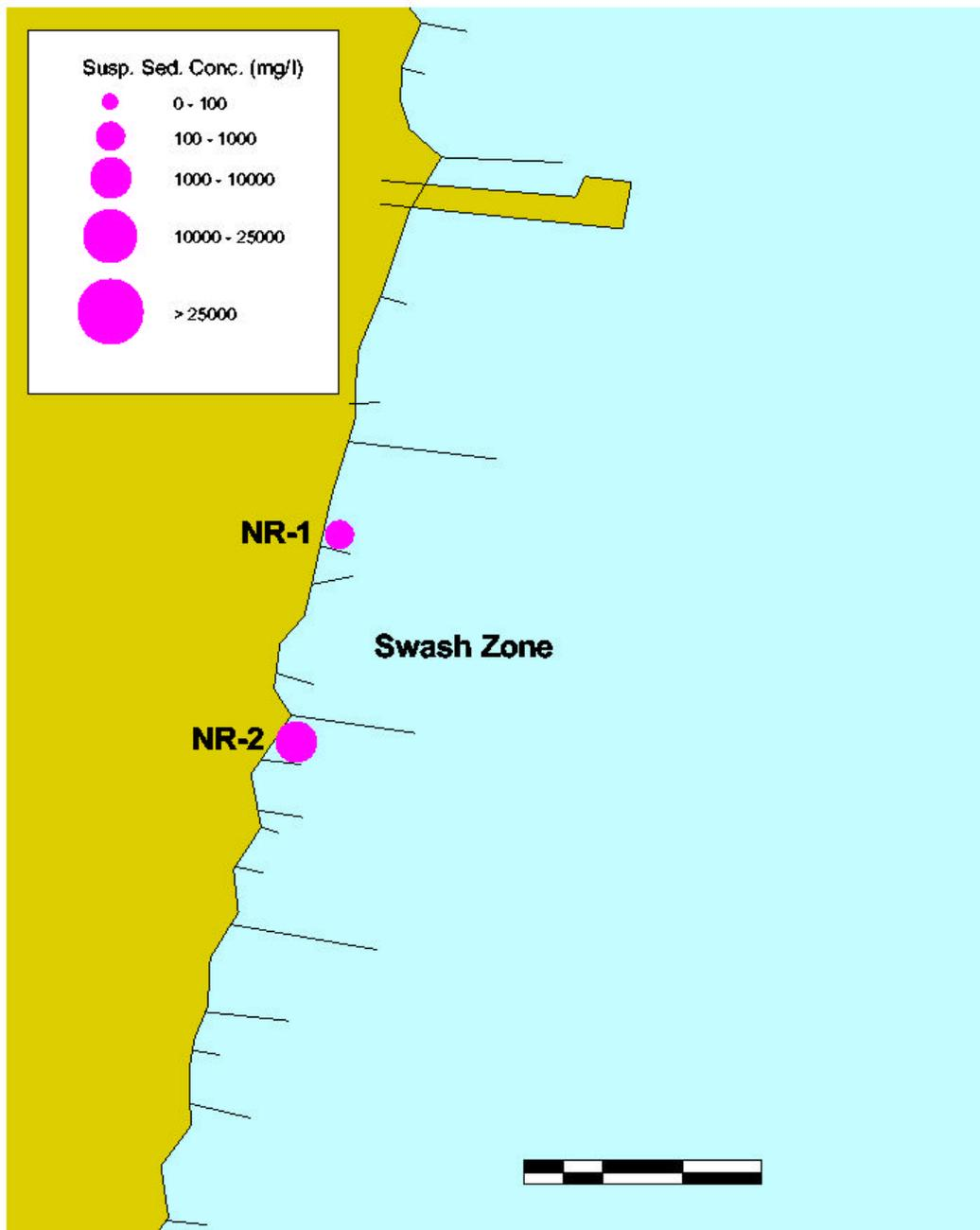
Figure 7-23. Suspended sediment concentrations at the North Reference Site swash zone on September 19, 1999. S = Surface, M = Mid Depth, B = Bottom.
