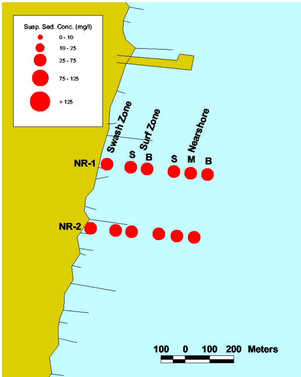
Figure 7-17. Suspended sediment concentrations at the North Reference Site on September 9, 1999. S = Surface, M = Mid Depth, B = Bottom.
