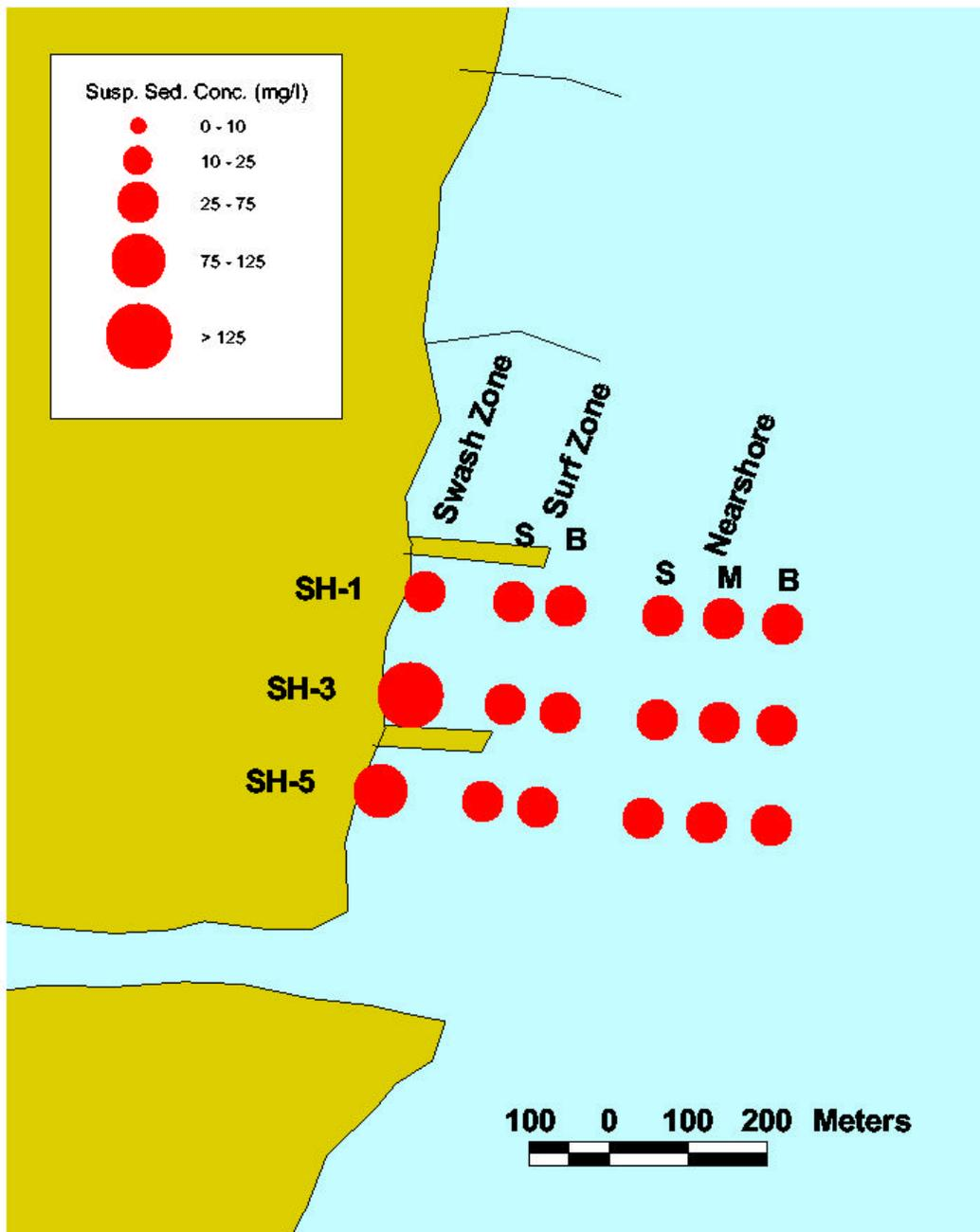
Figure 7-18. Suspended sediment concentrations at the Shark River Reference Site on September 9, 1999. S = Surface, M = Mid Depth, B = Bottom.
