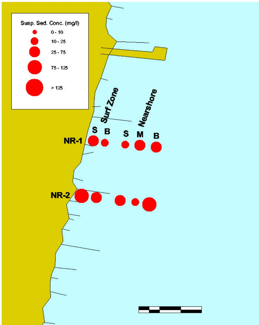
Figure 7-24. Suspended sediment concentrations at the North Reference Site on September 19, 1999. S = Surface, M = Mid Depth, B = Bottom.
