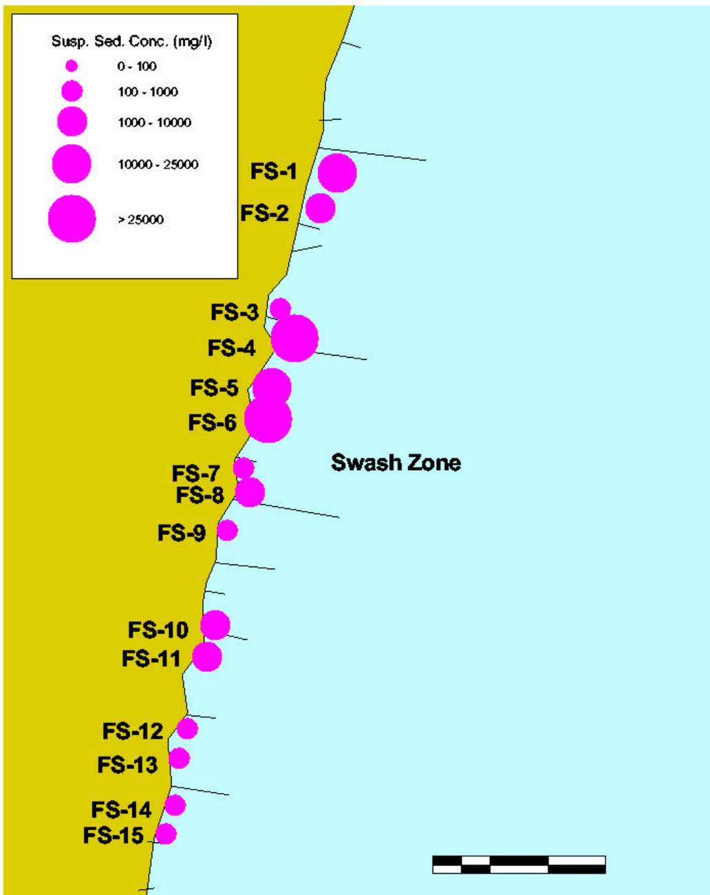
Figure 7-21. Suspended sediment concentrations at the Fill Site swash zone on September 19, 1999. S = Surface, M = Mid Depth, B = Bottom.
