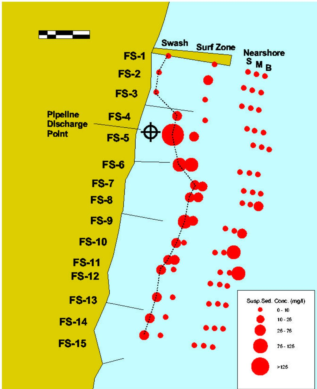
Figure 7-10. Suspended sediment concentrations at an active beach fill site on September 4, 1997. Dotted line represents approximate new beach face. S = Surface, M = Mid Depth, B = Bottom.
