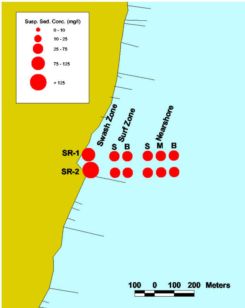
Figure 7-19. Suspended sediment concentrations at the South Reference Site on September 9, 1999. S = Surface, M = Mid Depth, B = Bottom.
