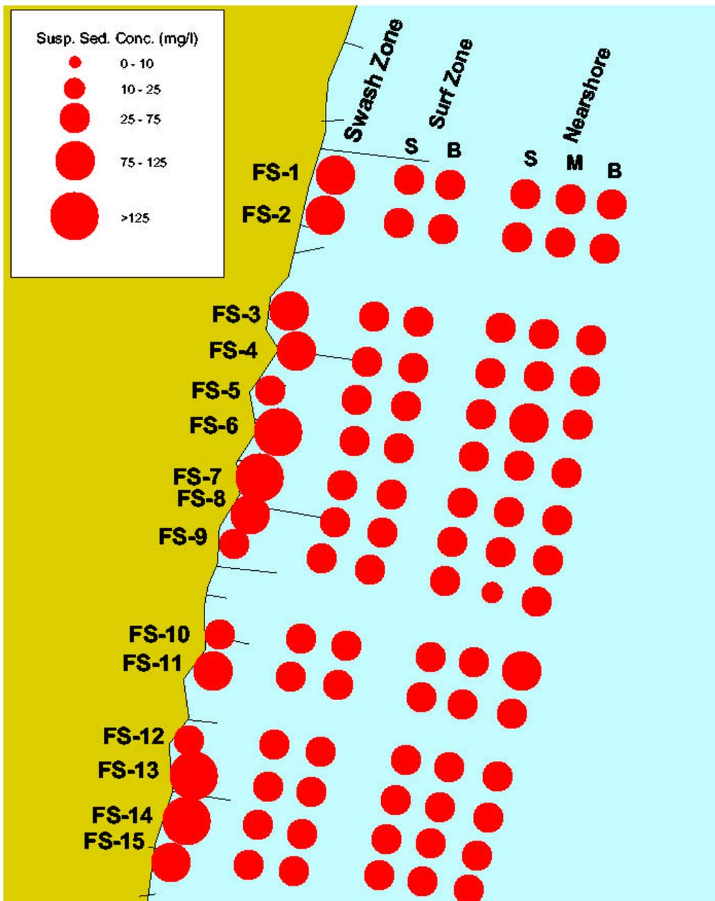
Figure 7-16. Suspended sediment concentrations at the Fill Site on September 9, 1999. S = Surface, M = Mid Depth, B = Bottom.
