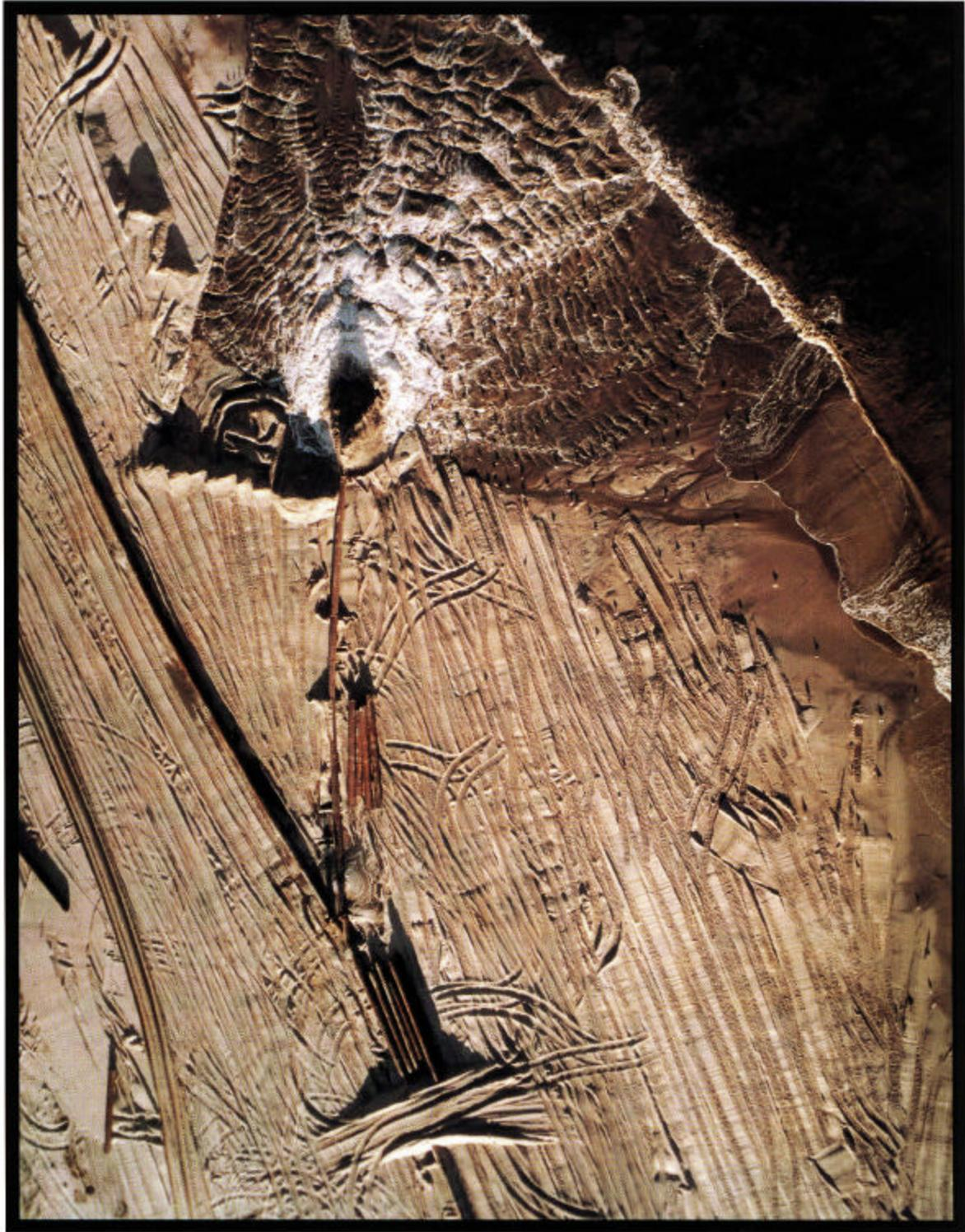
Figure 7-1. Aerial view of typical beach nourishment operation showing a pipeline discharge at a project site on Long Island, New York. (Courtesy of Great Lakes Dredge and Dock Company)
