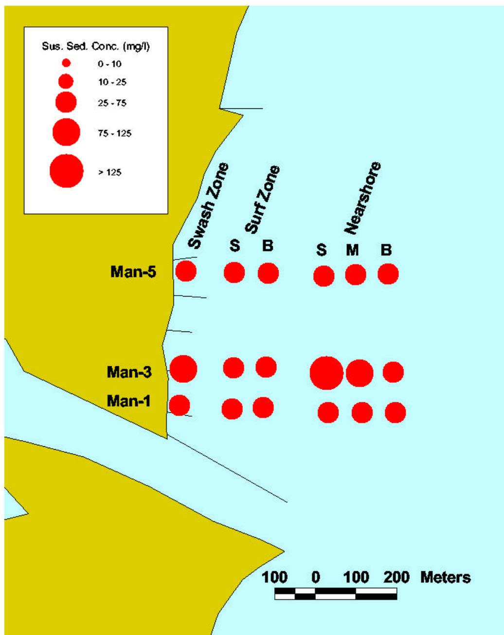
Figure 7-20. Suspended sediment concentrations at the Manasquan Reference Site on September 9, 1999. S = Surface, M = Mid Depth, B = Bottom.
