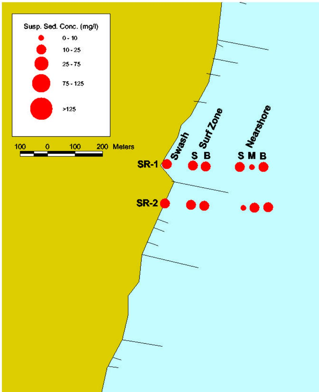
Figure 7-15. Suspended sediment concentrations at the South Reference Site on September 20, 1998. S = Surface, M = Mid Depth, B = Bottom.
