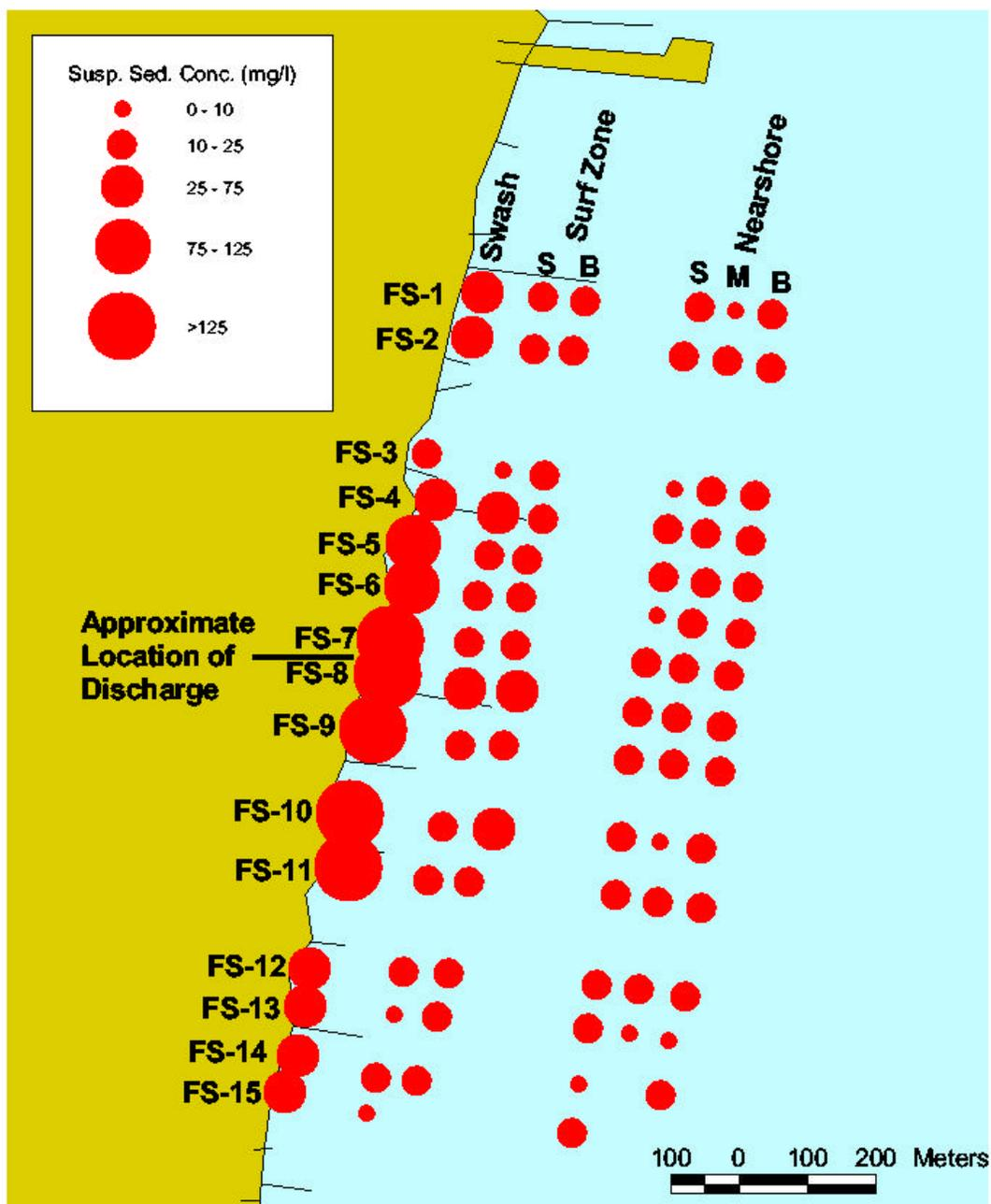
Figure 7-13. Suspended sediment concentrations at an active beach fill site on September 20, 1998. S = Surface, M = Mid Depth, B = Bottom.
