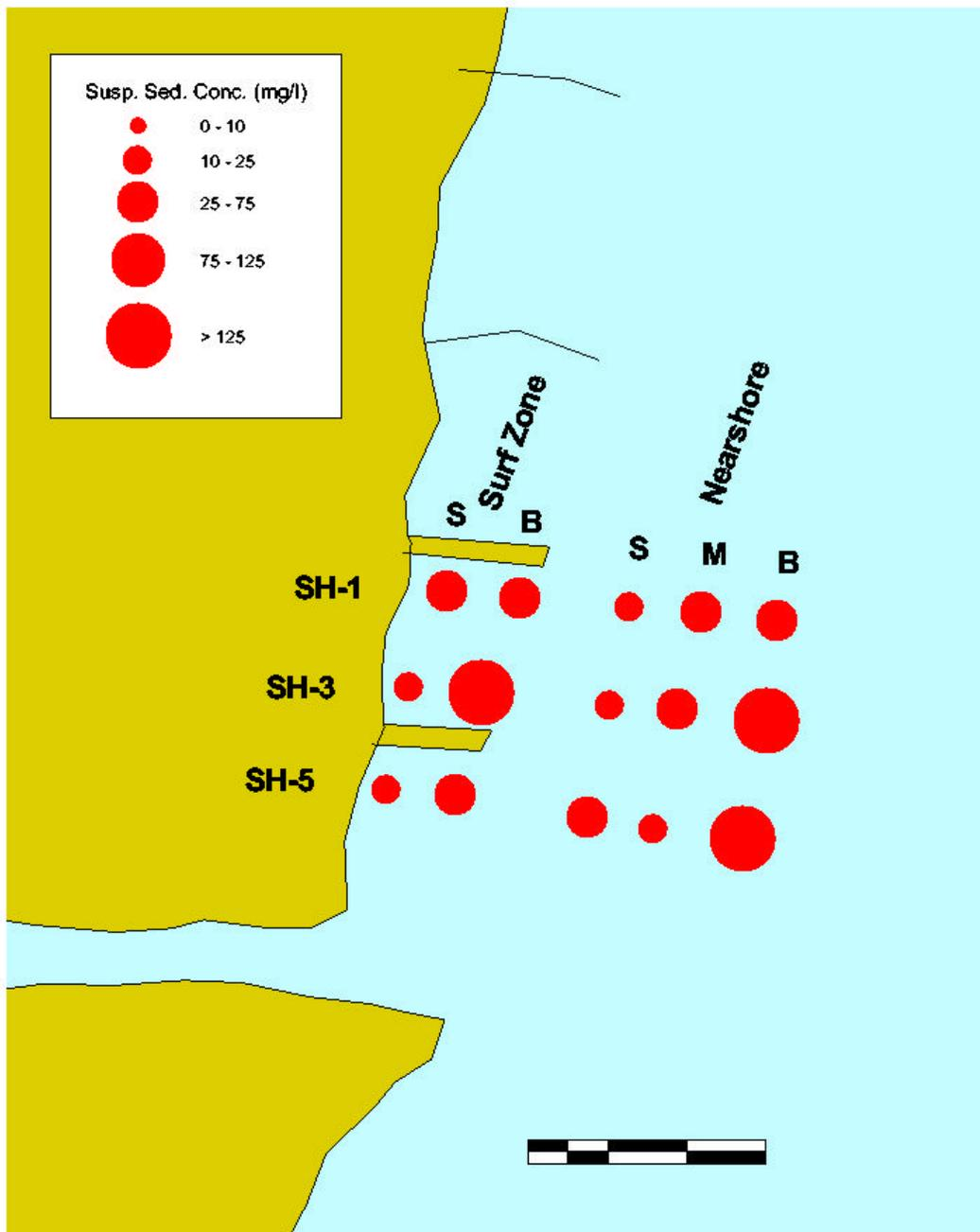
Figure 7-26. Suspended sediment concentrations at the Shark River Reference Site on September 19, 1999. S = Surface, M = Mid Depth, B = Bottom.
