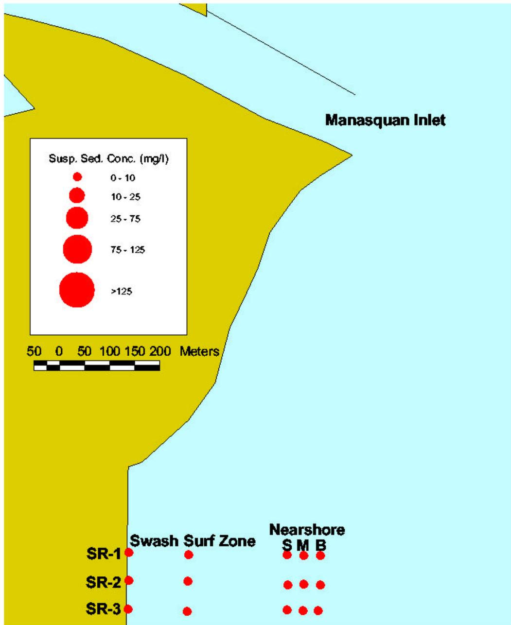
Figure 7-12. Suspended sediment concentrations at the South Reference Site on September 4, 1997. S = Surface, M = Mid Depth, B = Bottom.
