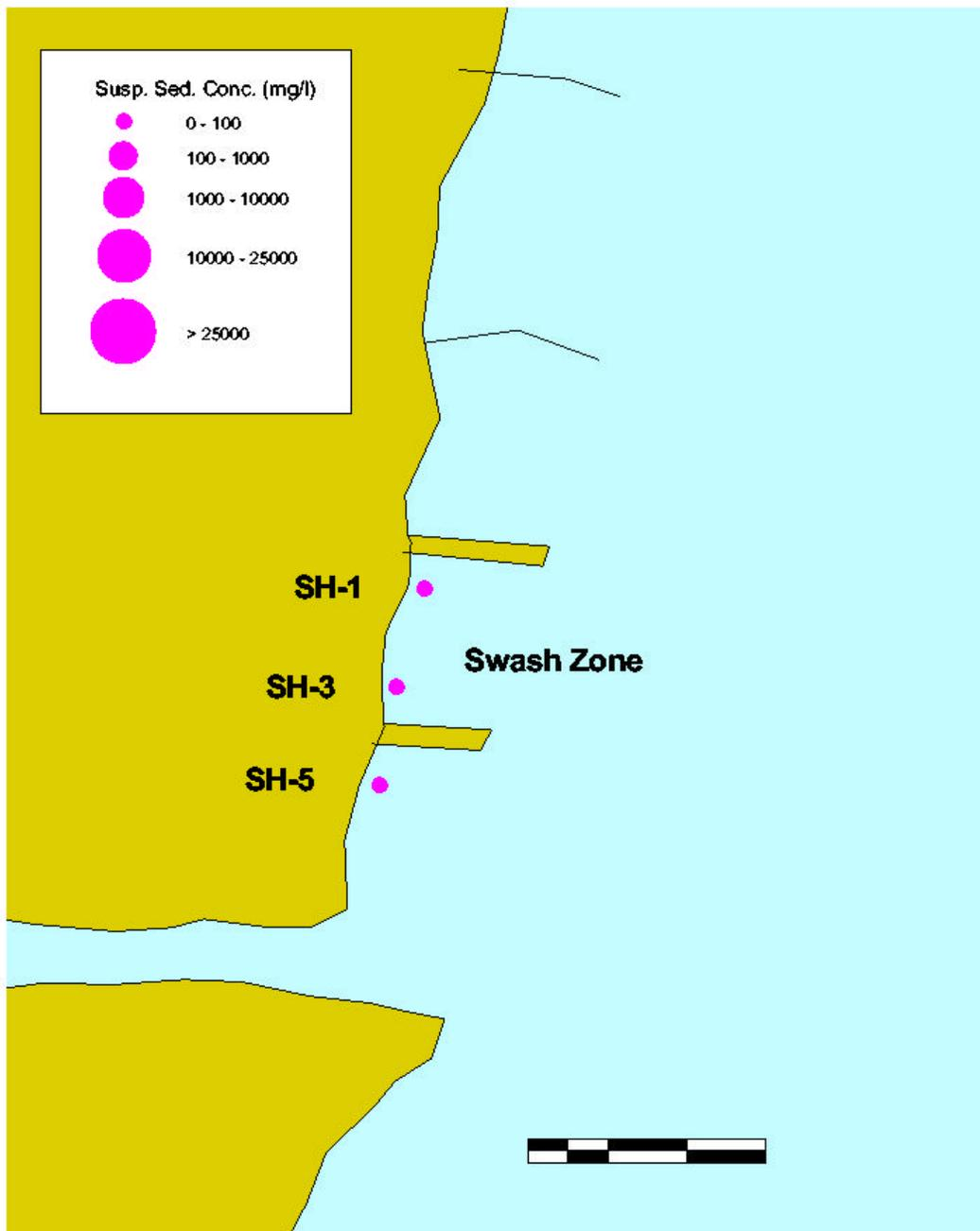
Figure 7-25. Suspended sediment concentrations at the Shark River Reference Site swash zone on September 19, 1999. S = Surface, M = Mid Depth, B = Bottom.
