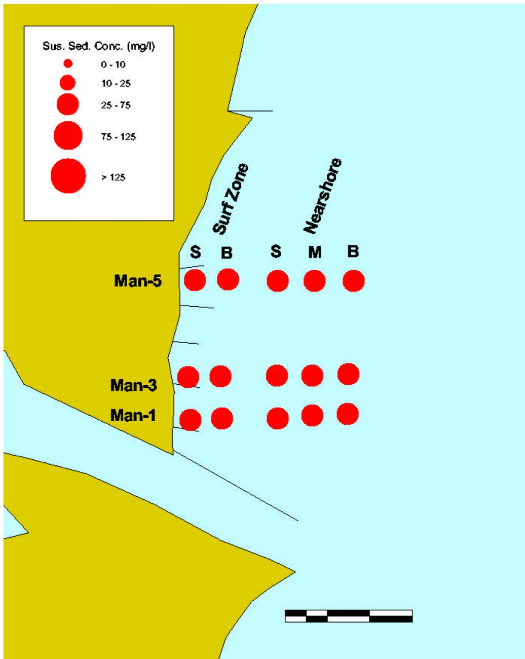
Figure 7-30. Suspended sediment concentrations at the Manasquan Reference Site on September 19, 1999. S = Surface, M = Mid Depth, B = Bottom.
