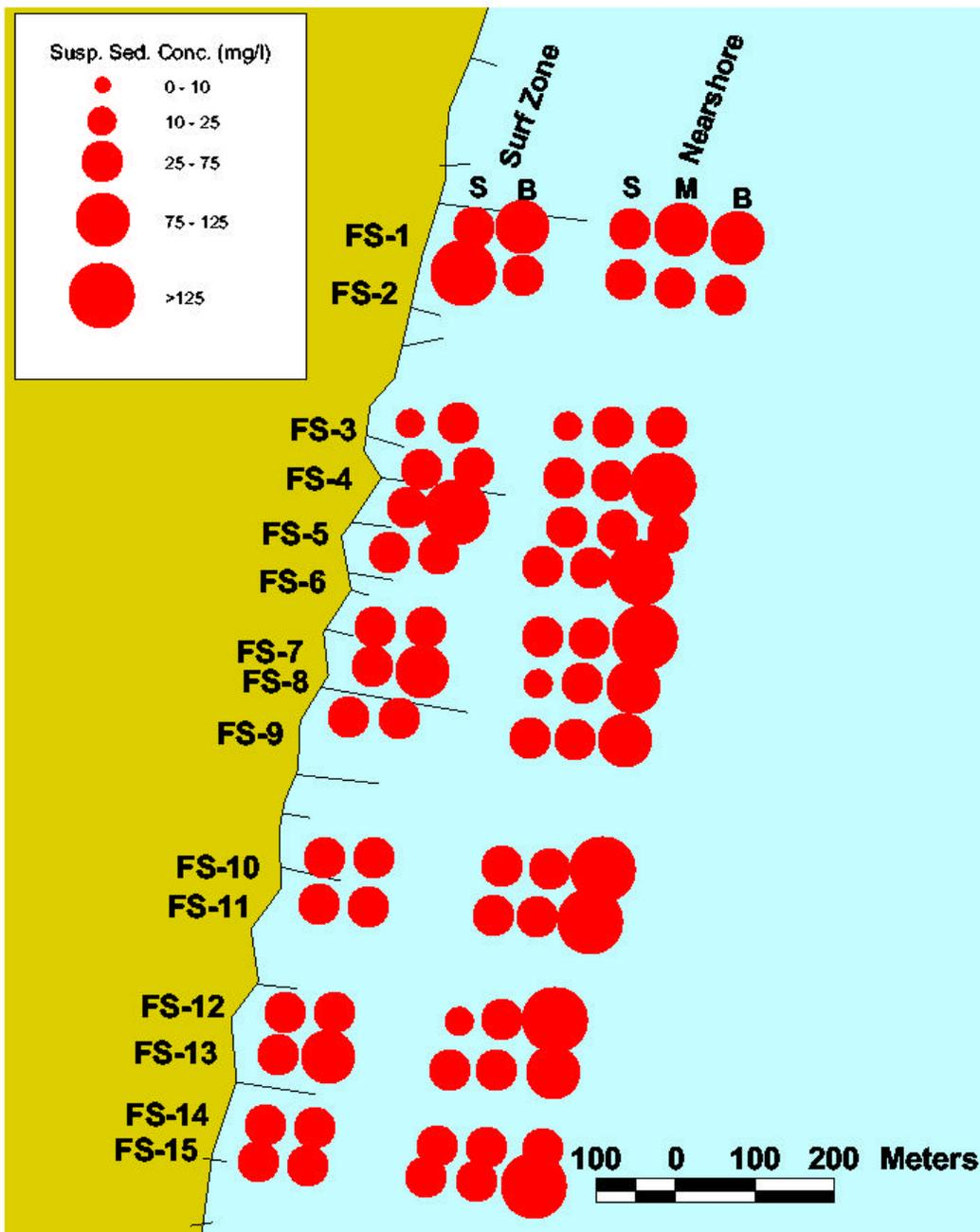
Figure 7-22. Suspended sediment concentrations at the Fill Site on September 19, 1999. S = Surface, M = Mid Depth, B = Bottom.
