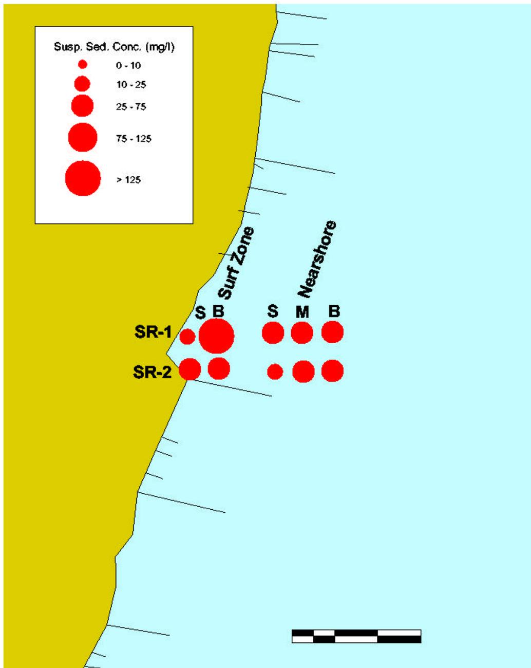
Figure 7-28. Suspended sediment concentrations at the South Reference Site on September 19, 1999. S = Surface, M = Mid Depth, B = Bottom.
