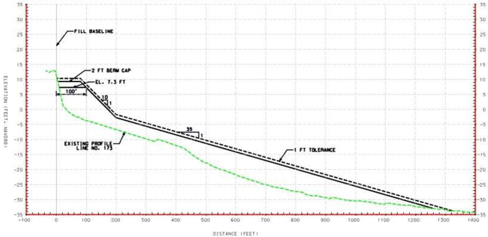
**Figure 4: Typical Design Profile Cross Section for the Elberon to Loch Arbour Reach**
