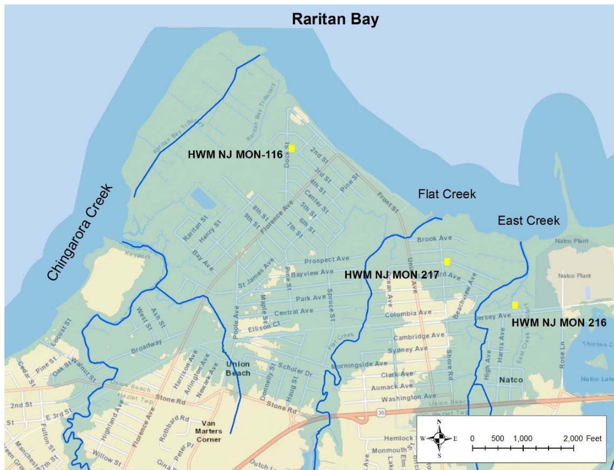
Figure 11: Hurricane Sandy Inundation Limits and USGS High Water Marks
