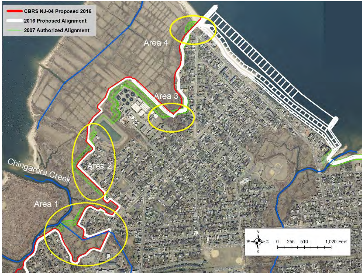
Figure 15. HSLRR Recommended Plan Changes in Alignment to Avoid CBRS Boundary
