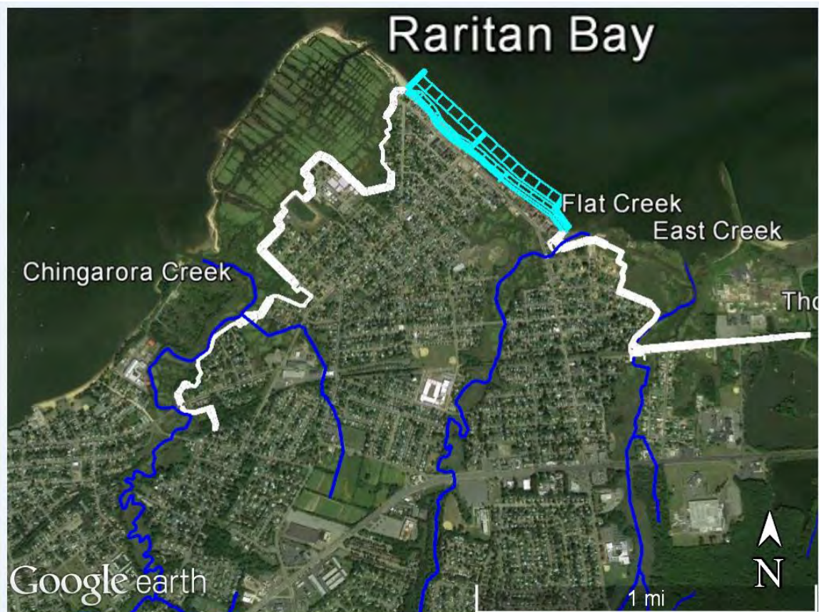
Figure 2: Overview of Authorized Project Alignment; White = Levees or Floodwalls Light Blue = Beach and Dune
