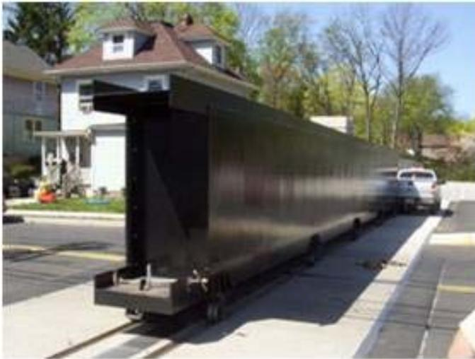
**Figure 18. Roller Gate Road Closure**
