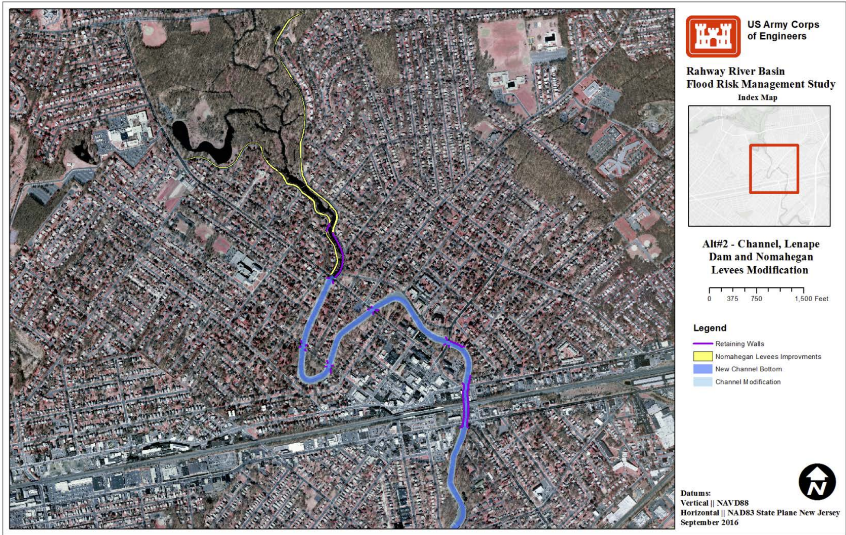
Figure 31: Channel and Nomahegan Levee modification footprint.
