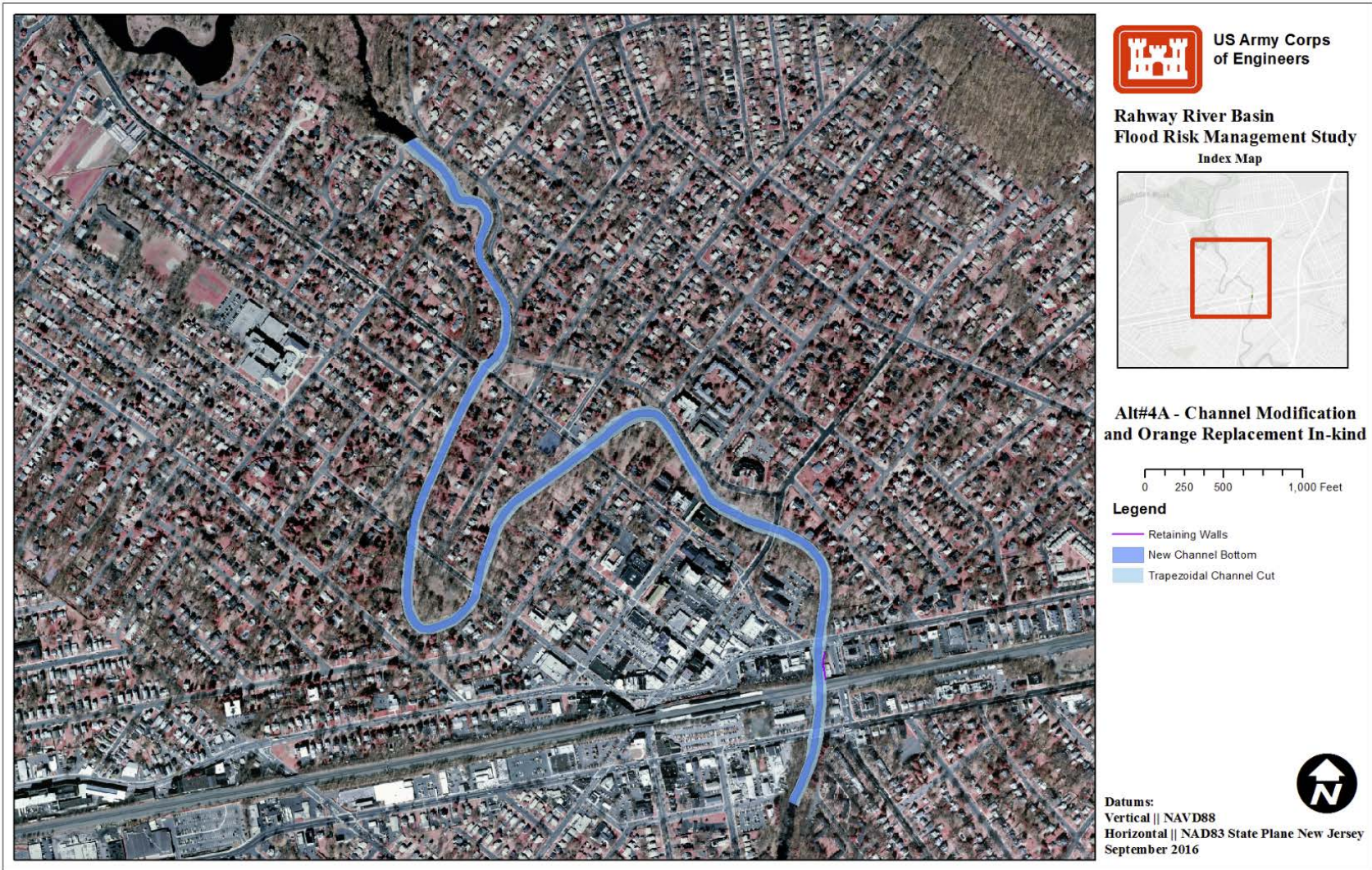
Figure 34: Reduced channel modification along the Rahway River in Cranford.
