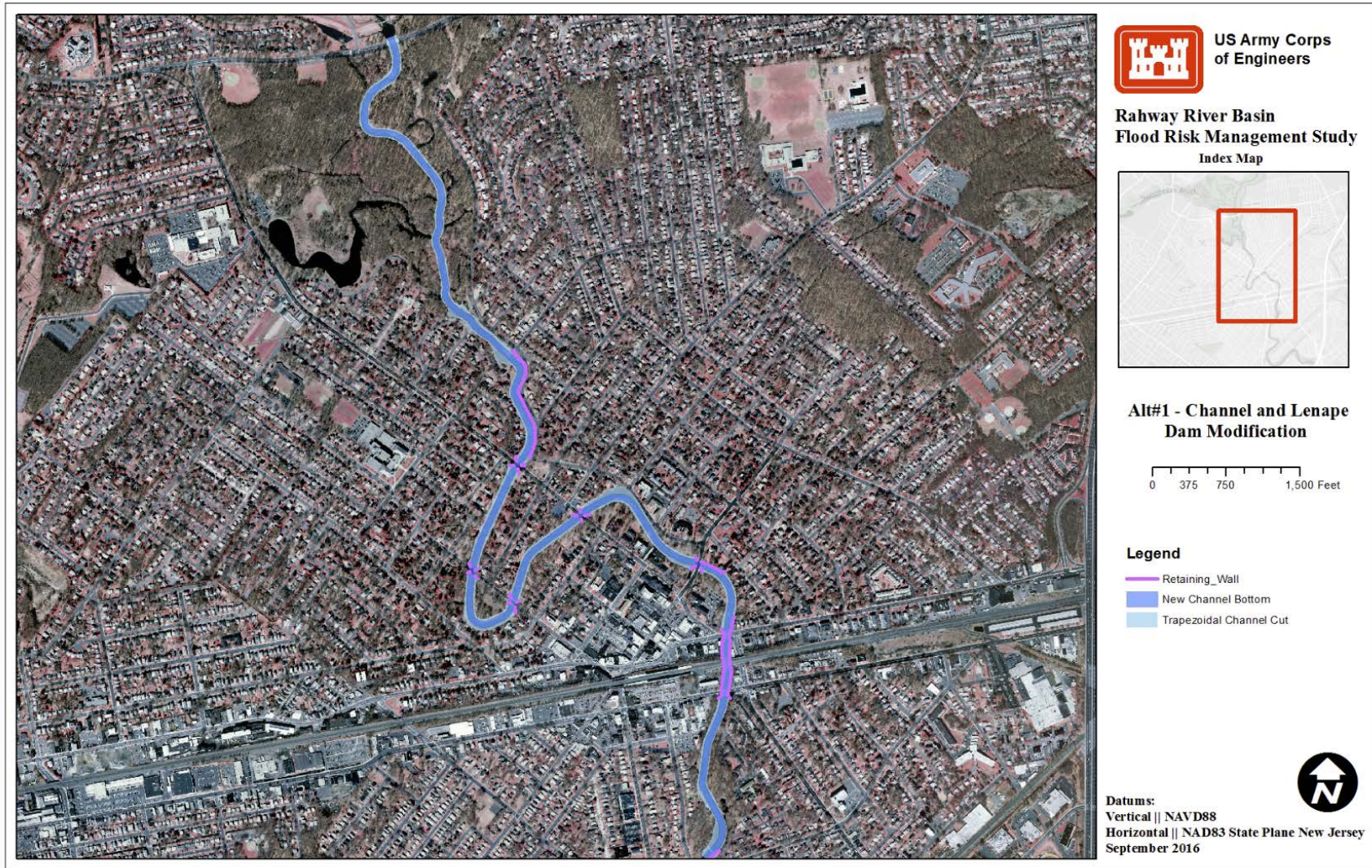
Figure 30: Channel modification footprint from Lenape Dam to Lincoln Ave. Bridge.
