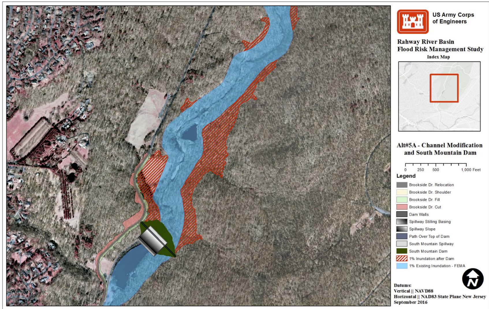
Figure 38: Proposed South Mountain dry detention dam and Brookside Drive relocation.
