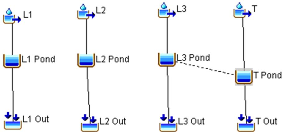
**Figure 20: Lister Avenue and Turnpike HEC-HMS Model Schematic**
