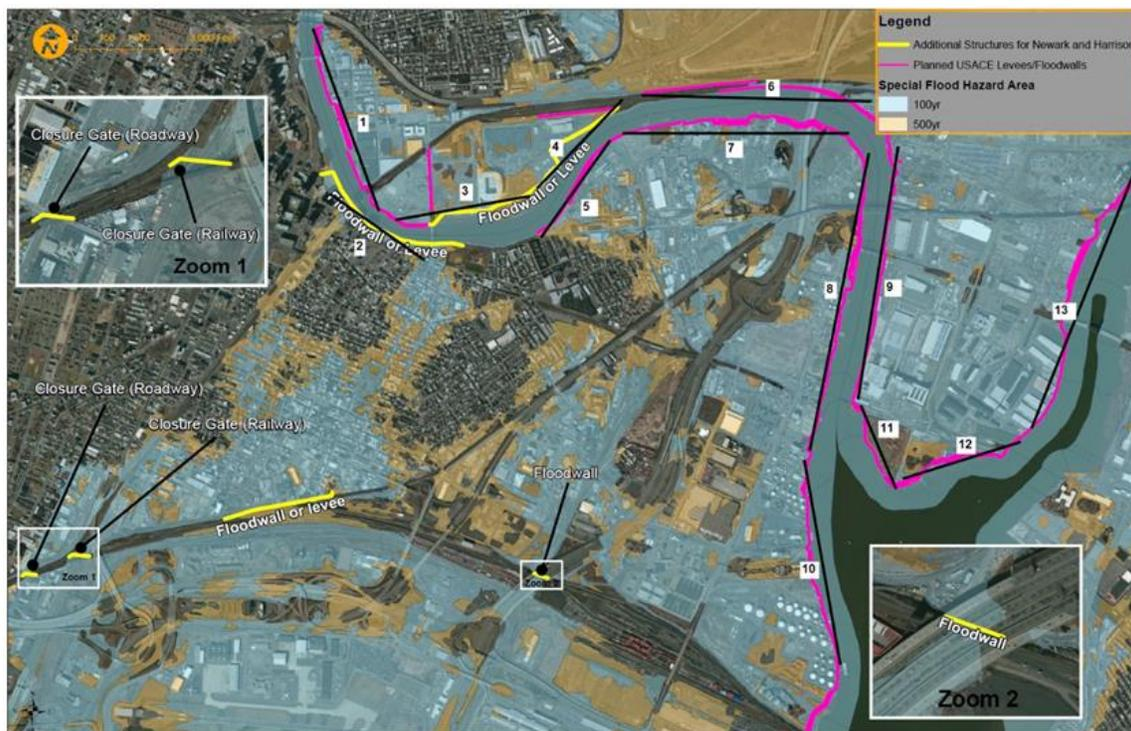
**Figure 8: Segmentation of Levee / Floodwall System**
