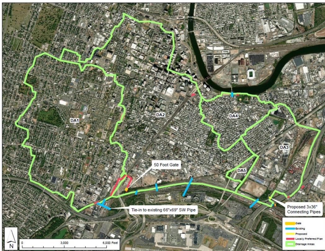
Figure 23: Passaic Tidal Project Existing and Recommended Interior Drainage Features
