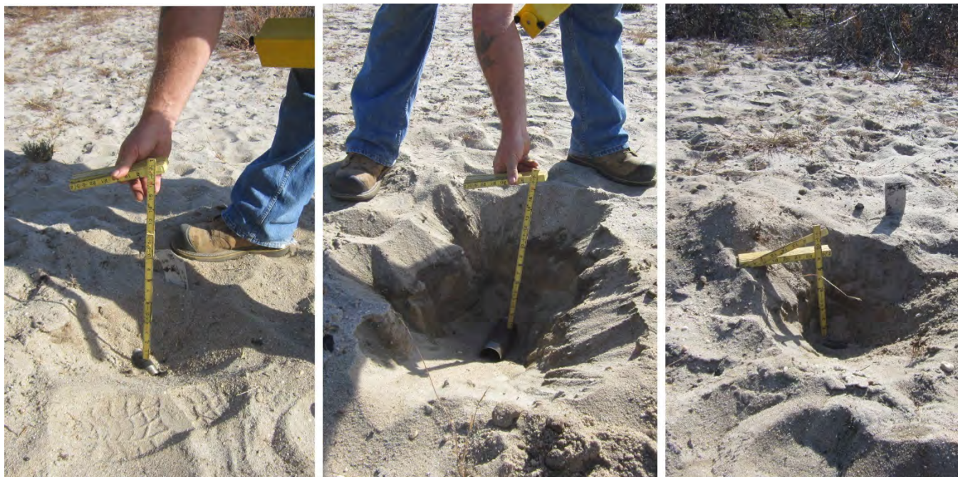
Photo 01 - Three industry standard objects (ISOs) buried in instrument verification strip (IVS).
