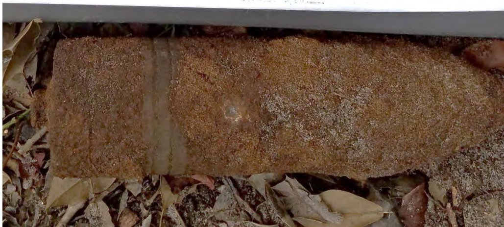
Photo 14 - 57mm round, M86 APHE (MEC, anom. 117-14). Date: 30 Nov. 2017
