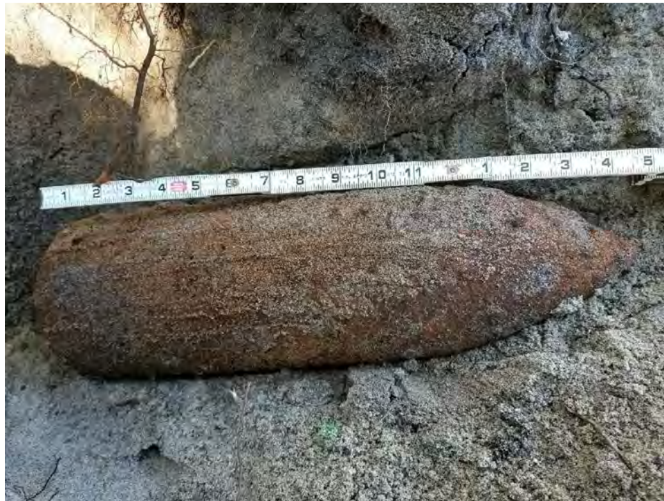
Photo 09 – 5 inch Naval projectile, fired, unfuzed (MD, anom. 199). Date: 27 Oct. 2017
