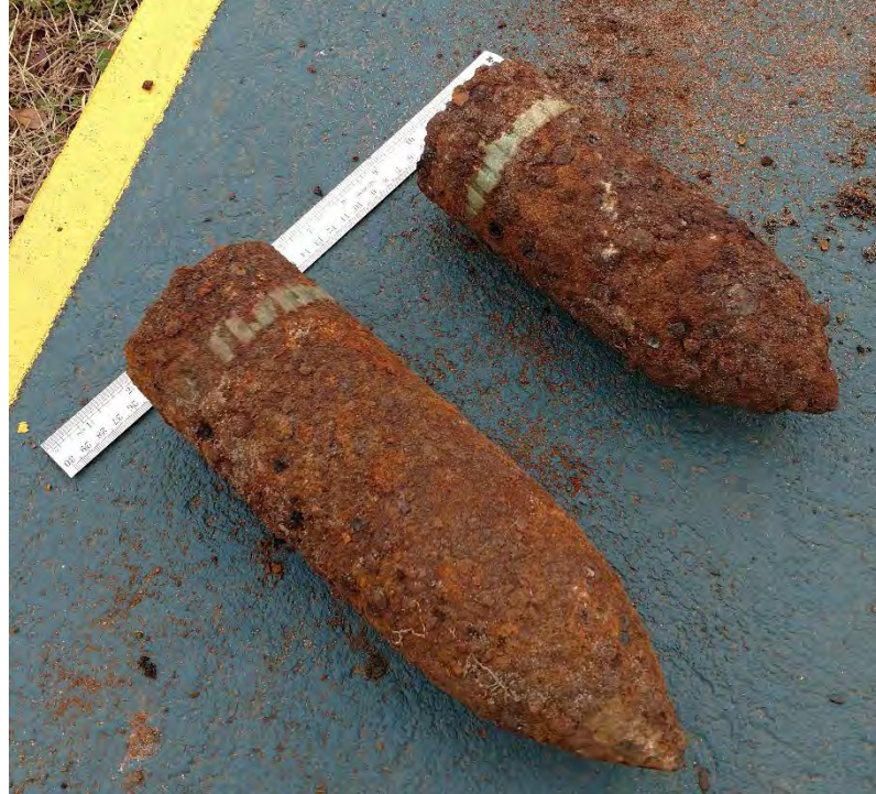
Photo 13 – Post-detonation photo of 4 inch MK10 APHE projectile with base plug (MEC, left, anom. 5-01), and 3 inch Mk 3 Model 7 projectile with tracer (MEC, right, anom. 140-05). Date: 7 Dec. 2017
