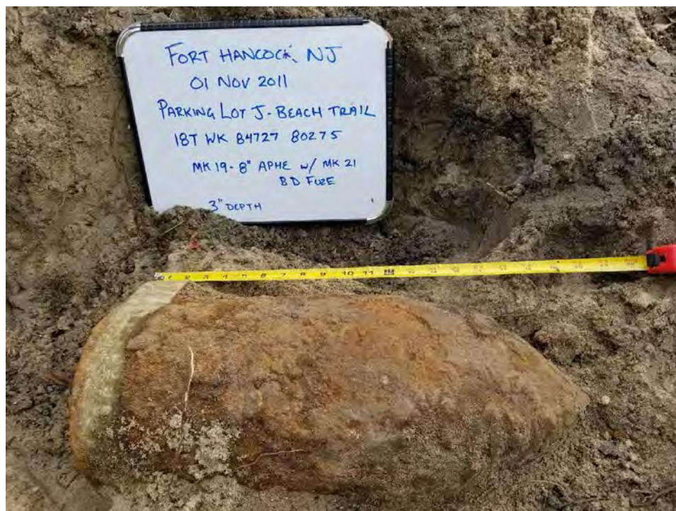
Photo 16 - 8 inch Mk19 HEAP Projectile (MD, anom. 512, on trail outside MRS 08). Date: 1 Nov. 2017
