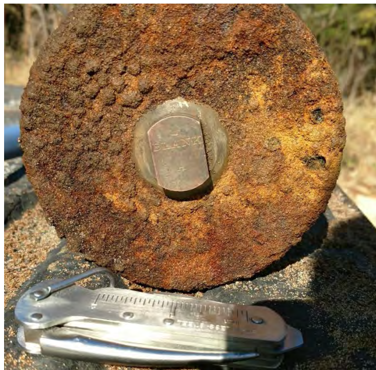
Photo 10 – “BLANK” printed on 5 inch projectile (MD, anom. 199). Date: 27 Oct. 2017
