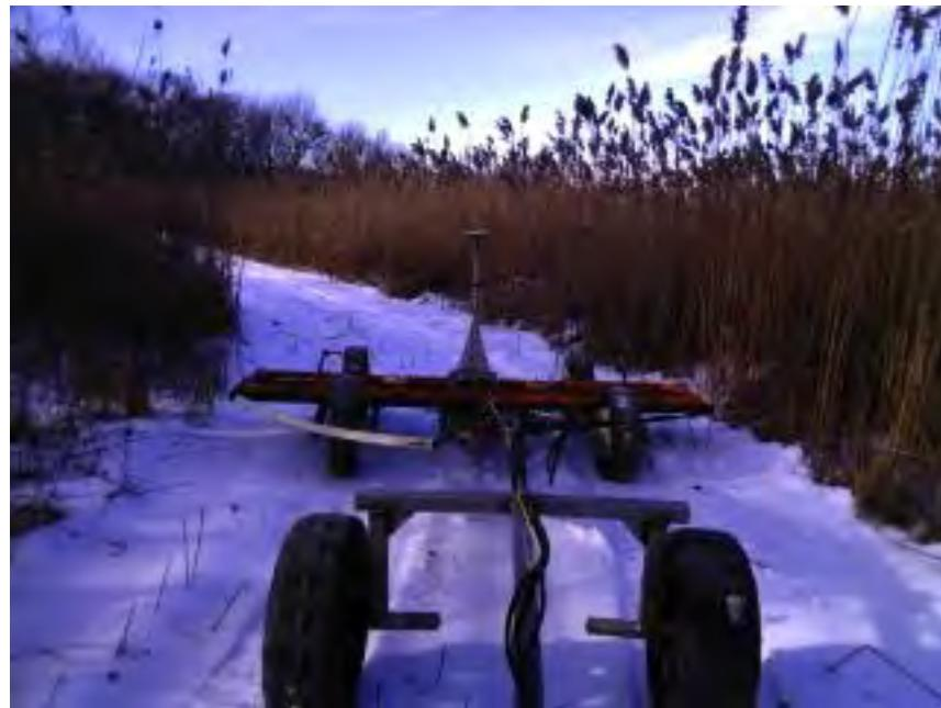
**Figure 2.** EM61-MK2 3-coil TA collection with RTK-GPS
