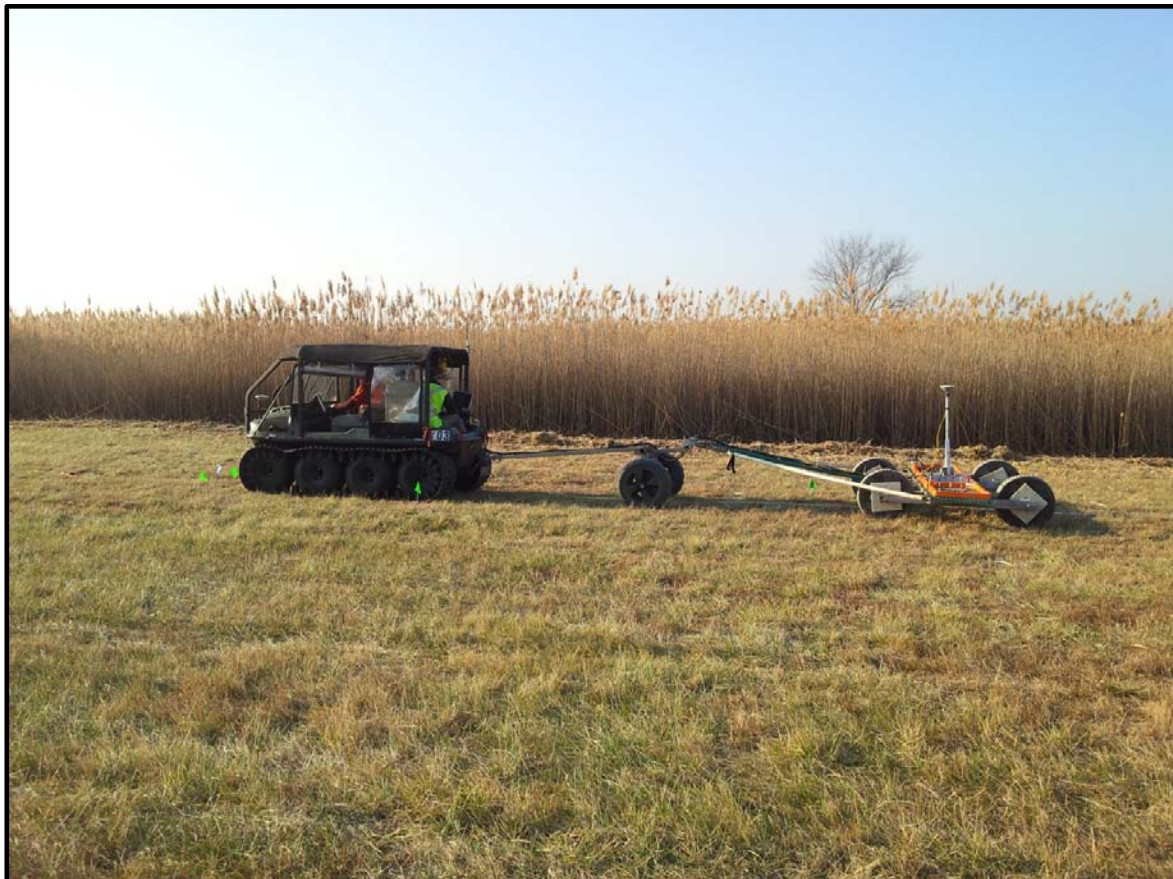
FIGURE 3-1 Triple-Coil Towed-Array EM61-MK2 IVS Survey
