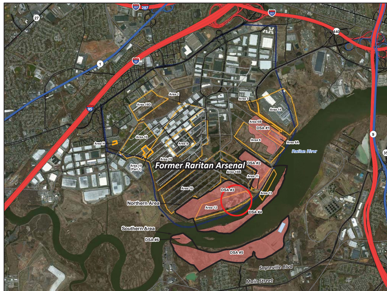
Figure 1 Former Raritan Arsenal boundary [blue outline] Investigation Areas [yellow box] Dredge Spoil Area [red box]
