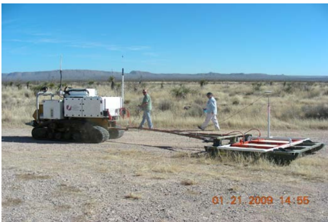
Advanced Mobility Research and Development System (AMRADS) autonomous platform with EM-61 towed array
