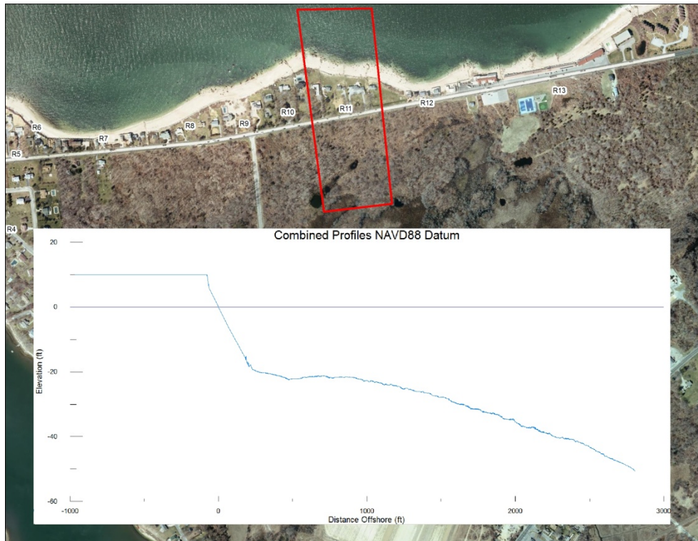
Figure 26: Representative and idealized beach profile for Reach R11.
