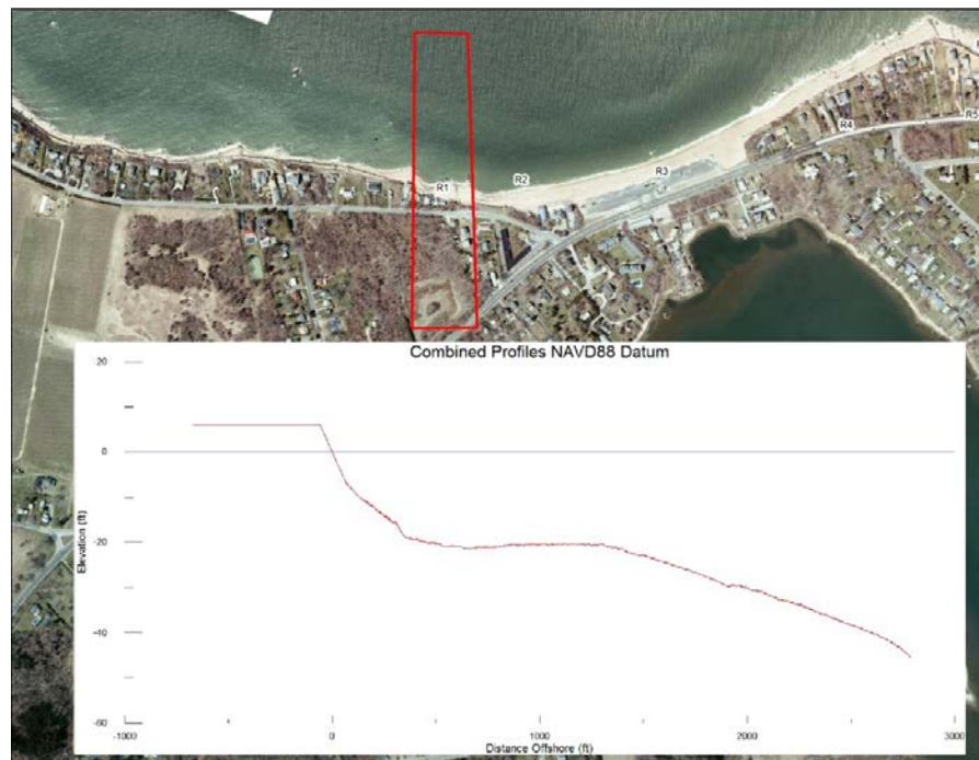
Figure 16: Representative and idealized beach profile for Reach R1.
