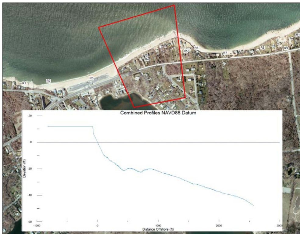
Figure 19: Representative and idealized beach profile for Reach R4.
