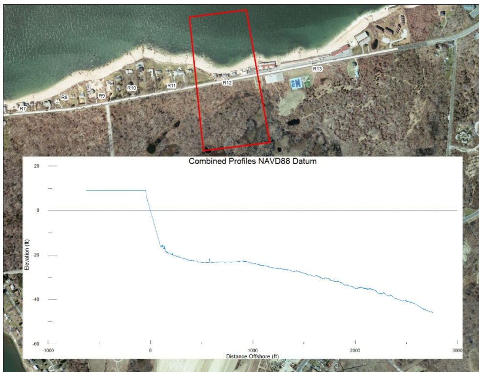
Figure 27: Representative and idealized beach profile for Reach R12.
