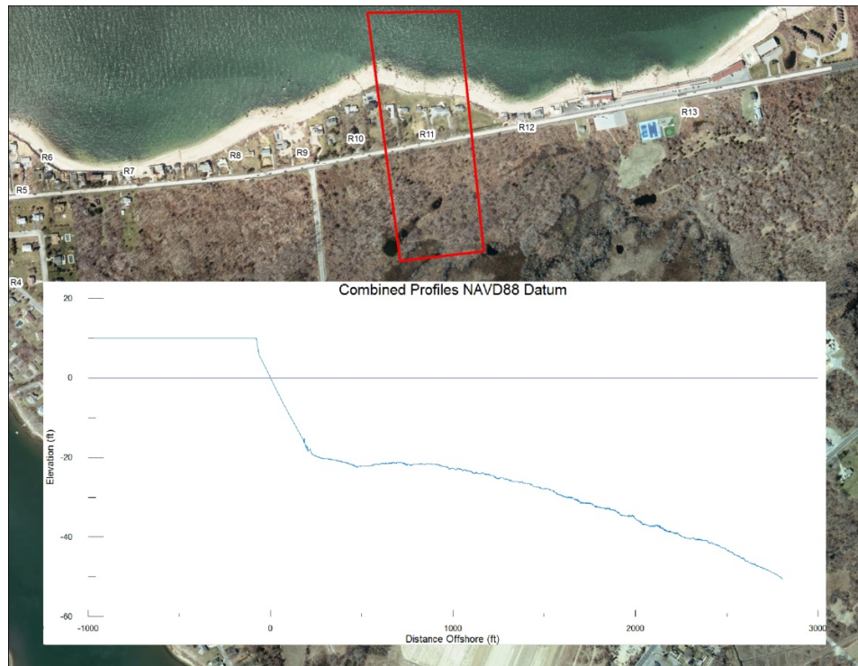
Figure 33: Representative and idealized beach profile for Reach R11.
