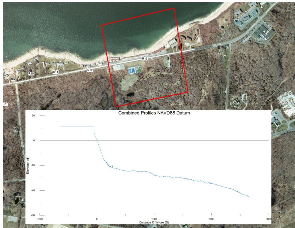
Figure 35: Representative and idealized beach profile for Reach R13.
