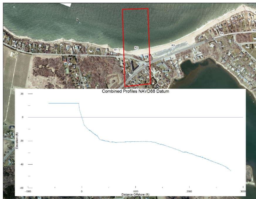
Figure 24: Representative and idealized beach profile for Reach R2.
