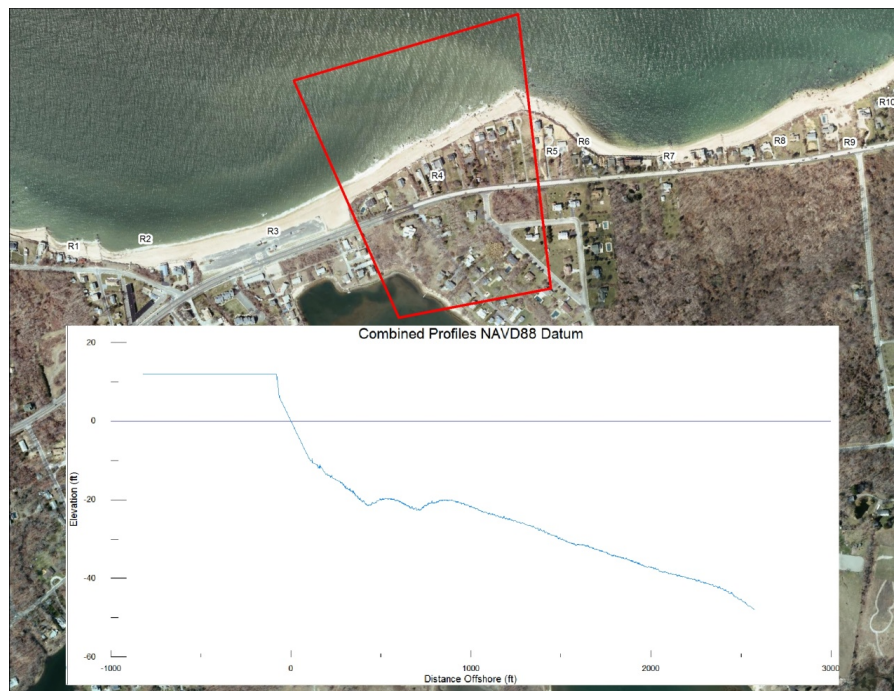
Figure 26: Representative and idealized beach profile for Reach R4.
