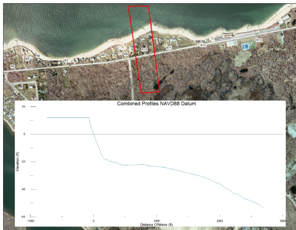
Figure 32: Representative and idealized beach profile for Reach R10.
