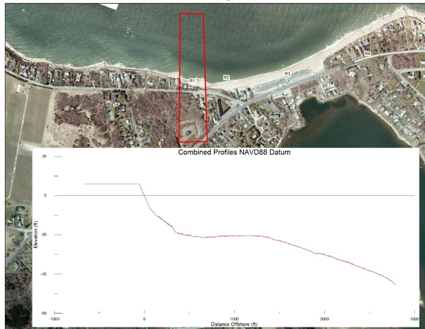
Figure 23: Representative and idealized beach profile for Reach R1.
