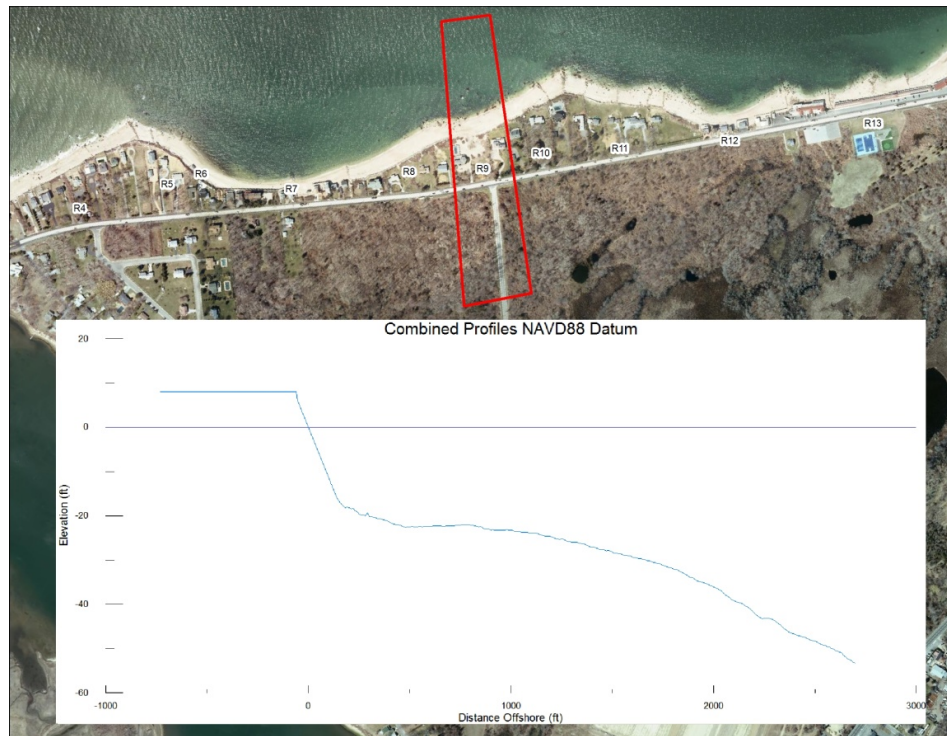
Figure 31: Representative and idealized beach profile for Reach R9.
