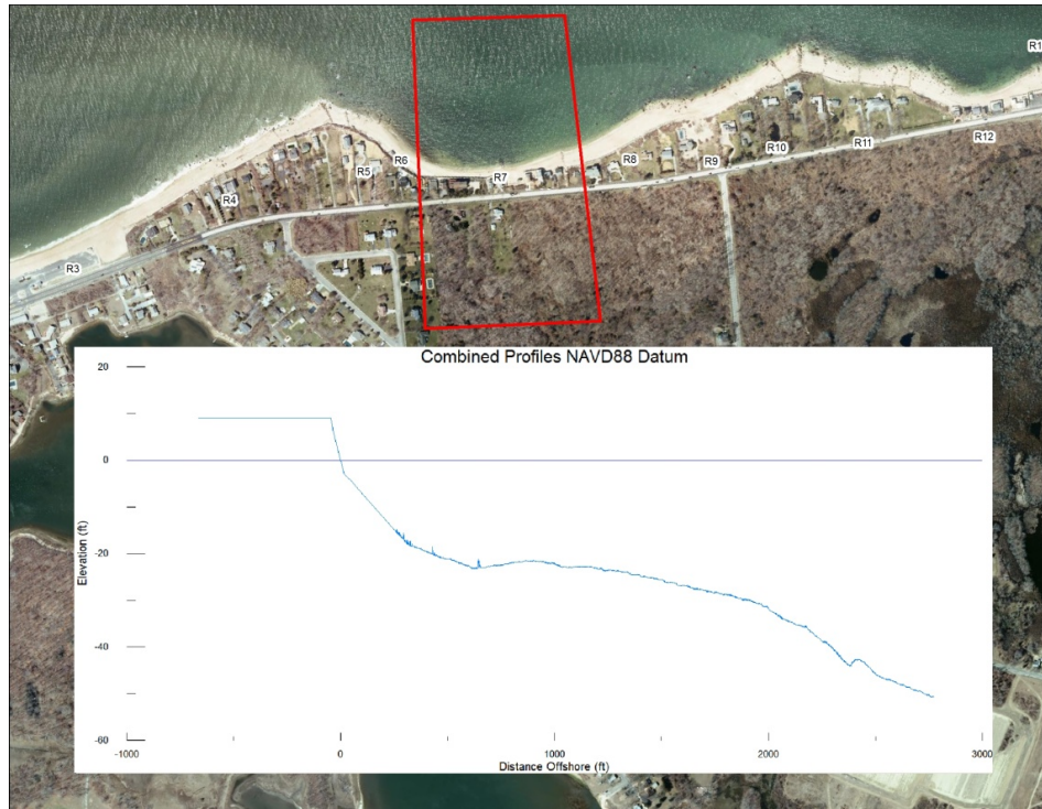
Figure 29: Representative and idealized beach profile for Reach R7.
