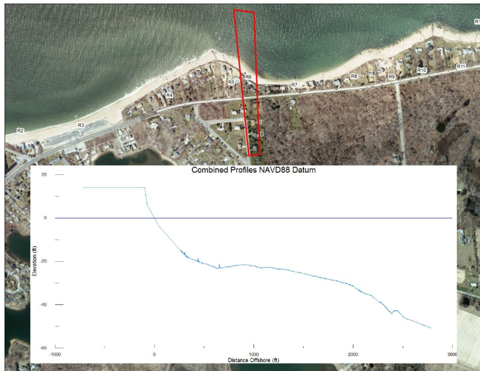
Figure 28: Representative and idealized beach profile for Reach R6.
