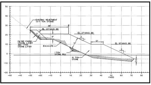
HSLRR revetment typical cross section
