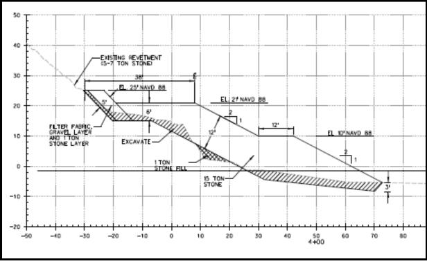
Figure 3. HSLRR Revetment Typical Cross Section
