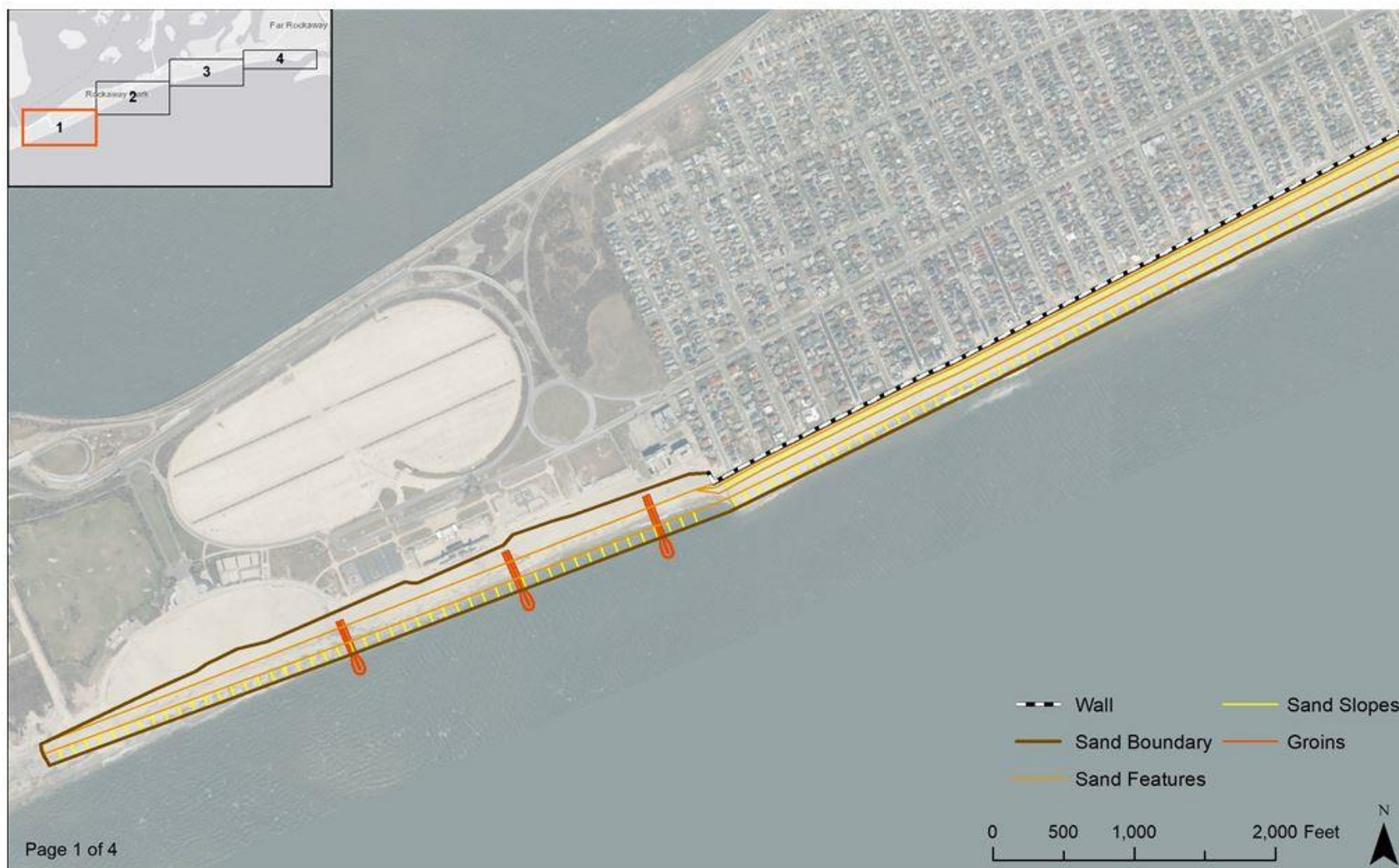
Figure 2a: Atlantic Ocean Shorefront Component of Recommended Plan (1 of 4)
