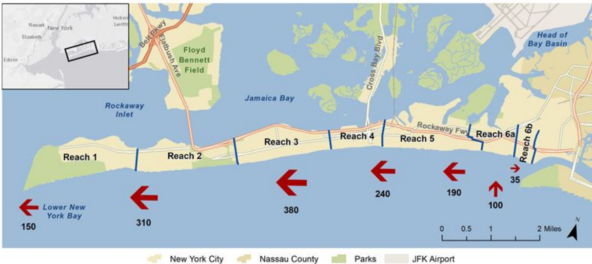
Figure 3-1: Future Without Project Sediment Transport Pathways at the Atlantic Ocean Shorefront Planning Reach
