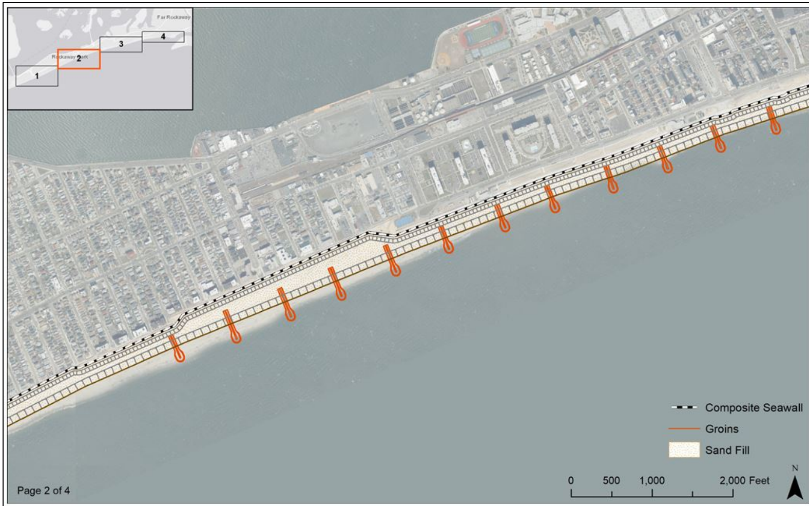
Figure 4: Groin Rehabilitation, beach fill and composite seawall along the Atlantic shoreline.
