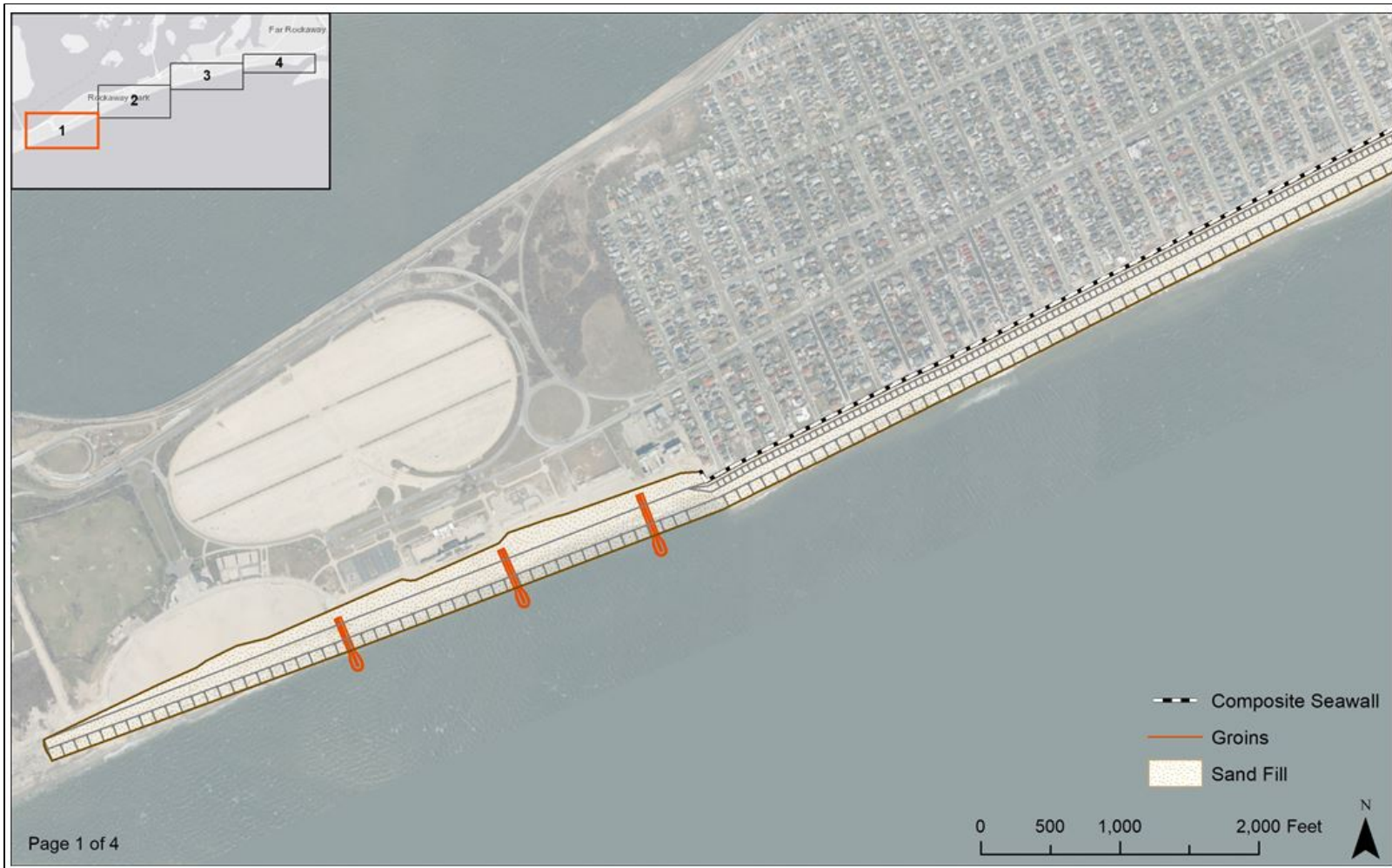
Figure 3: Groin rehabilitation and beach fill in Jacob Riis Park with the composite seawall just outside the park extending east along the Atlantic shoreline.
