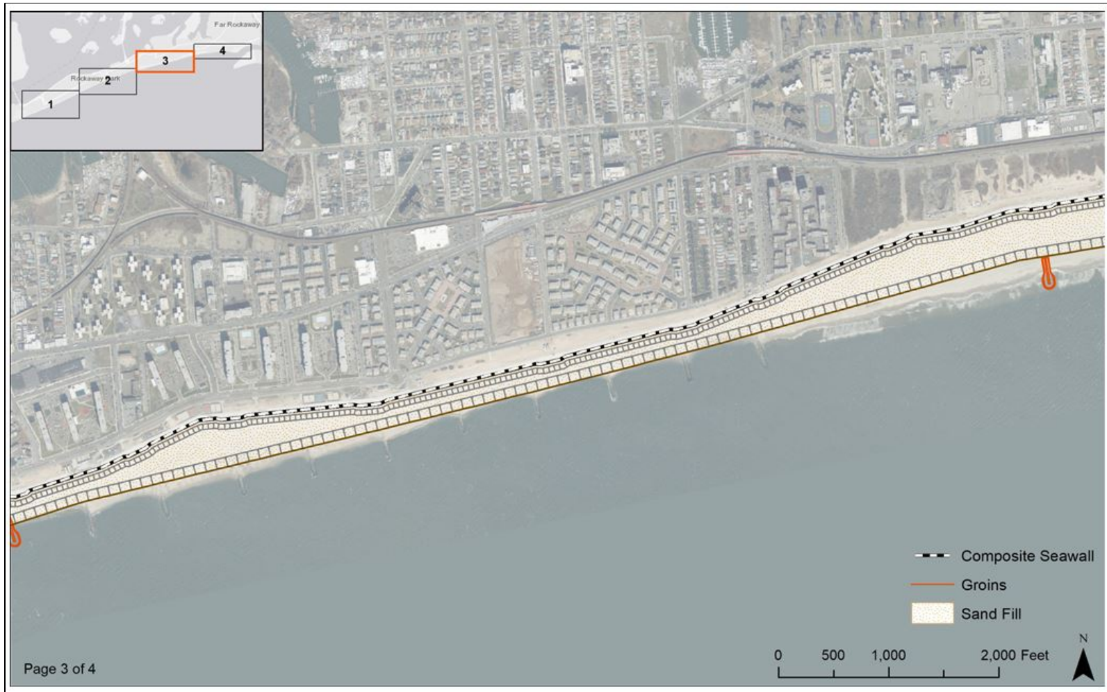
Figure 5: Composite seawall, beach fill and new groin construction (east) along the Atlantic shoreline.
