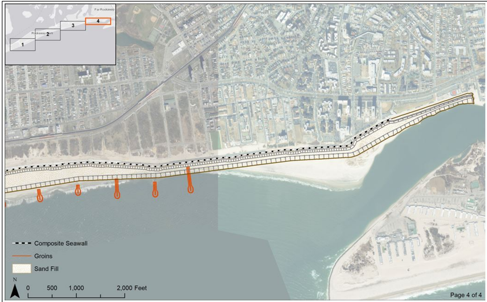
Figure 6: New groin construction, beach fill and composite seawall along the Atlantic shoreline.
