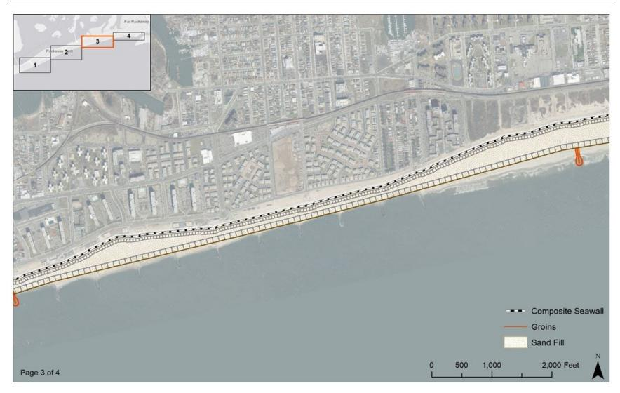
Figure 6-6c: Atlantic Shorefront Component of Recommended Plan (3 of 4)
