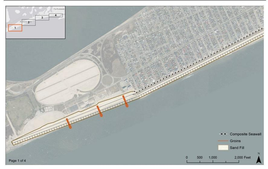
Figure 6-6a: Atlantic Shorefront Component of Recommended Plan (1 of 4)
