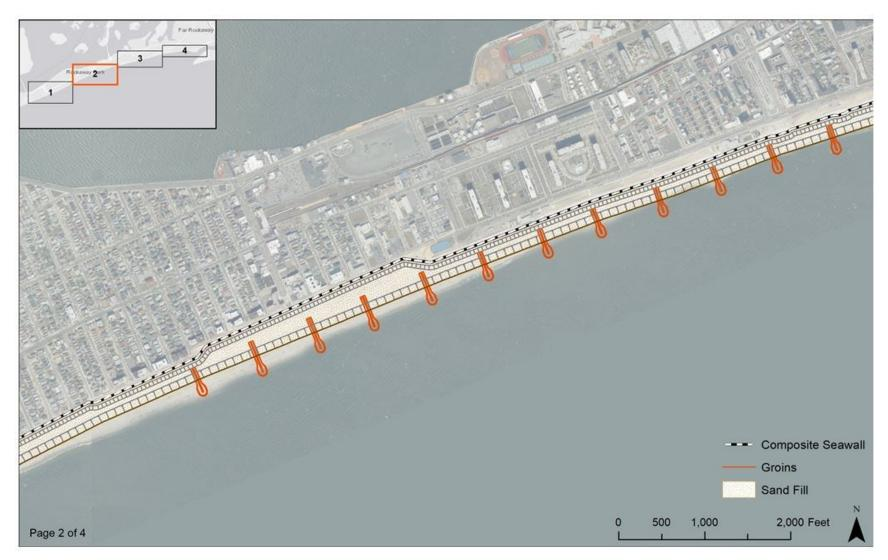
Figure ES-4b: Atlantic Shorefront Component of Recommended Plan (2 of 4)
