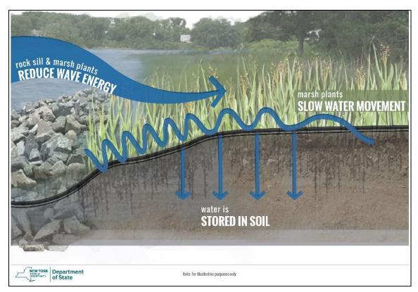
Figure 4-4: Marsh and Rock Sill NNBF Concept Illustration
