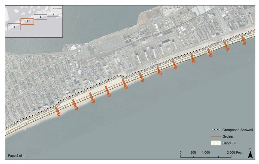
Figure 6-6b: Atlantic Shorefront Component of Recommended Plan (2 of 4)
