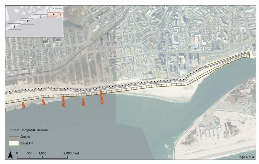
Figure 6-6d: Atlantic Shorefront Component of Recommended Plan (4 of 4)
