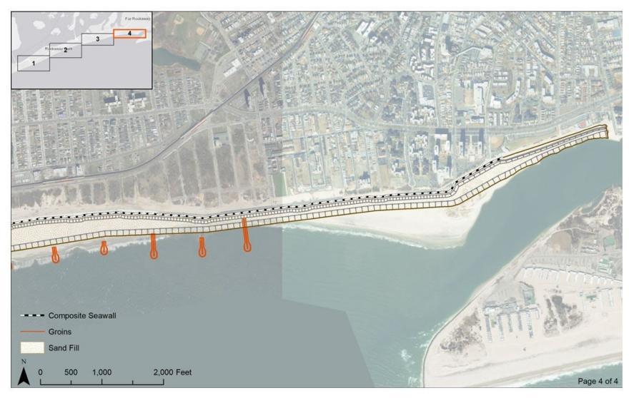
Figure ES-4d: Atlantic Shorefront Component of Recommended Plan (4 of 4)
