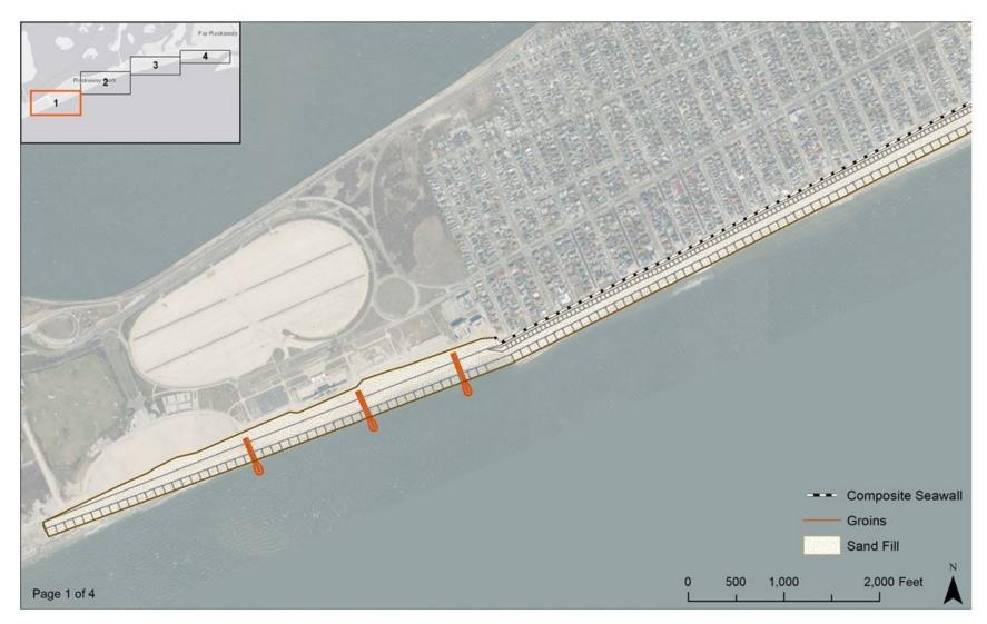
Figure ES-4a: Atlantic Shorefront Component of Recommended Plan (1 of 4)
