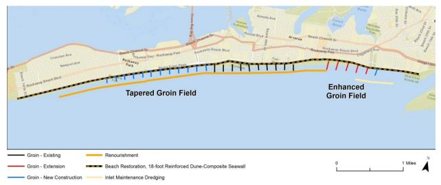
Figure 5-4: Beach Restoration with Beachfill, Groin Extensions, and New Groins
