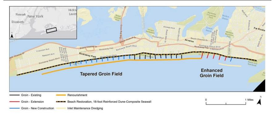
Figure 6-5: Atlantic Shorefront Component of the Recommended Plan - Overview
