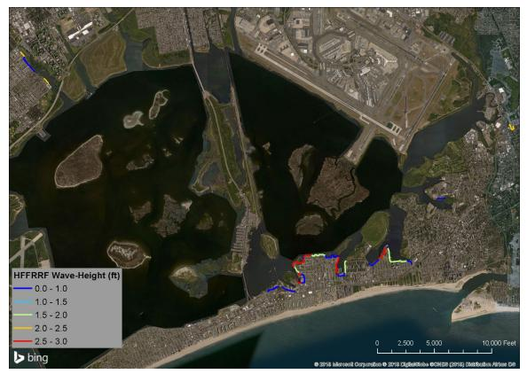
Figure 5-13: Calculated Wave-heights at HFFRRF Alignments
