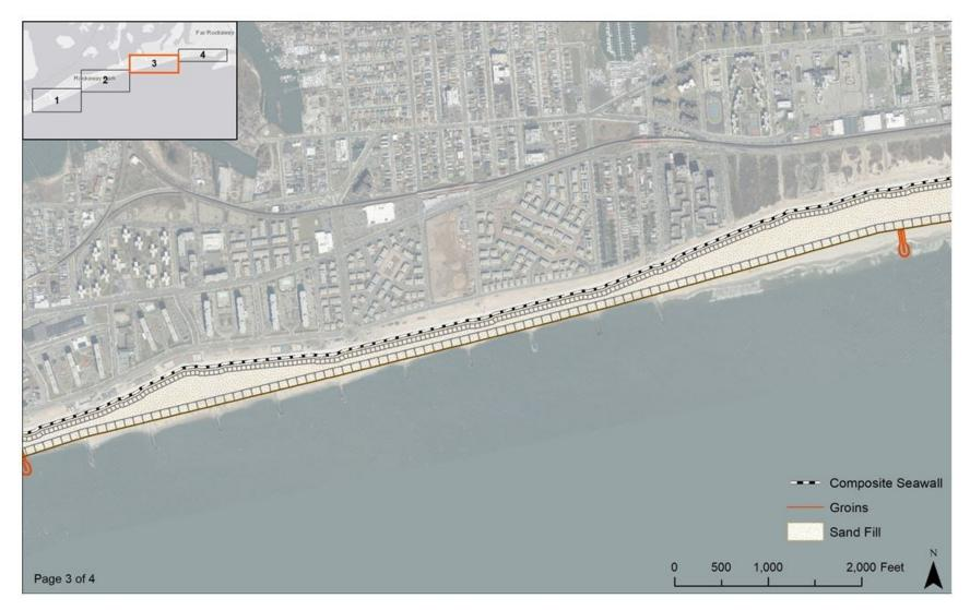
Figure ES-4c: Atlantic Shorefront Component of Recommended Plan (3 of 4)
