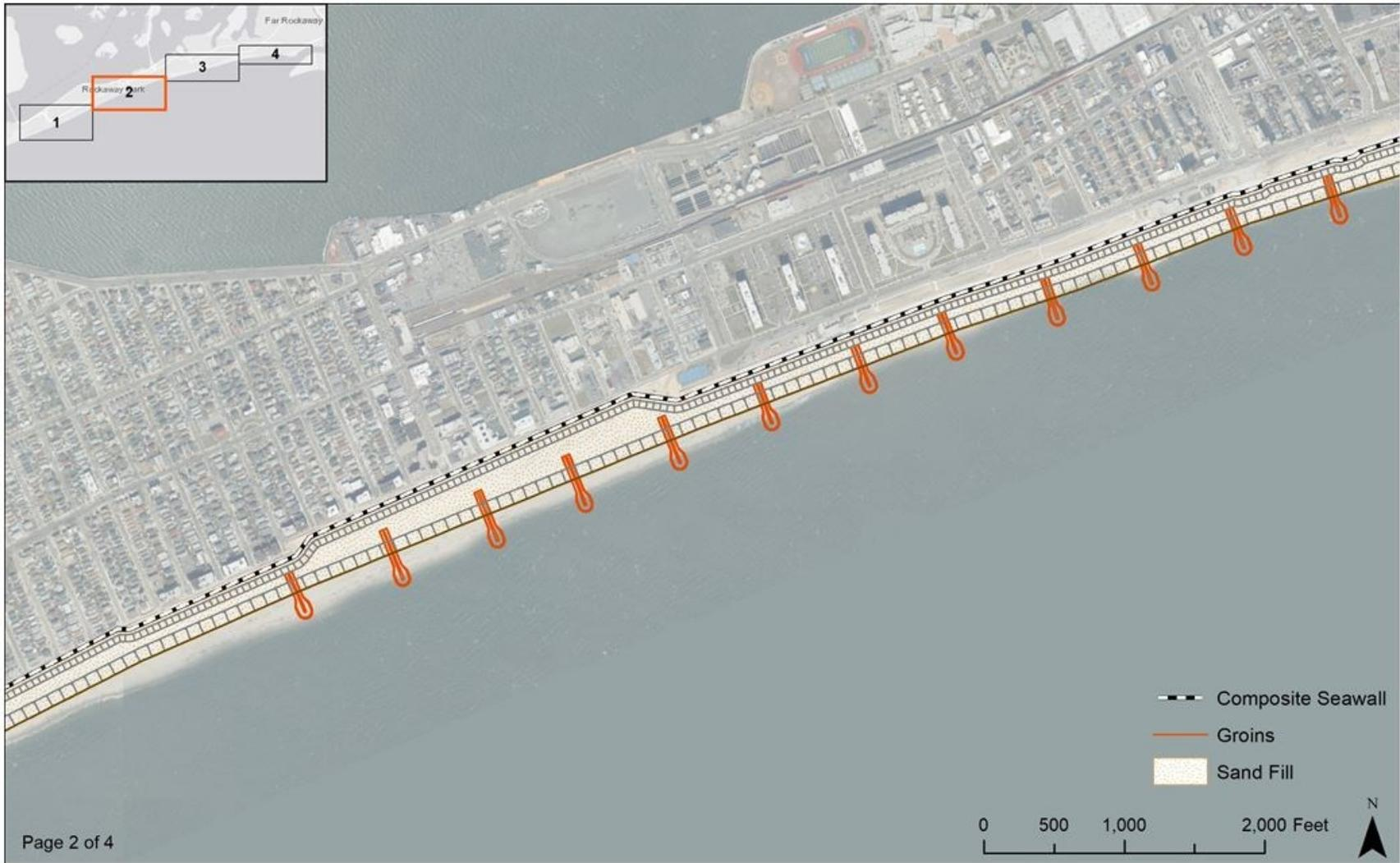
**Figure ES-4b: Atlantic Shorefront Component of Recommended Plan (2 of 4)**
