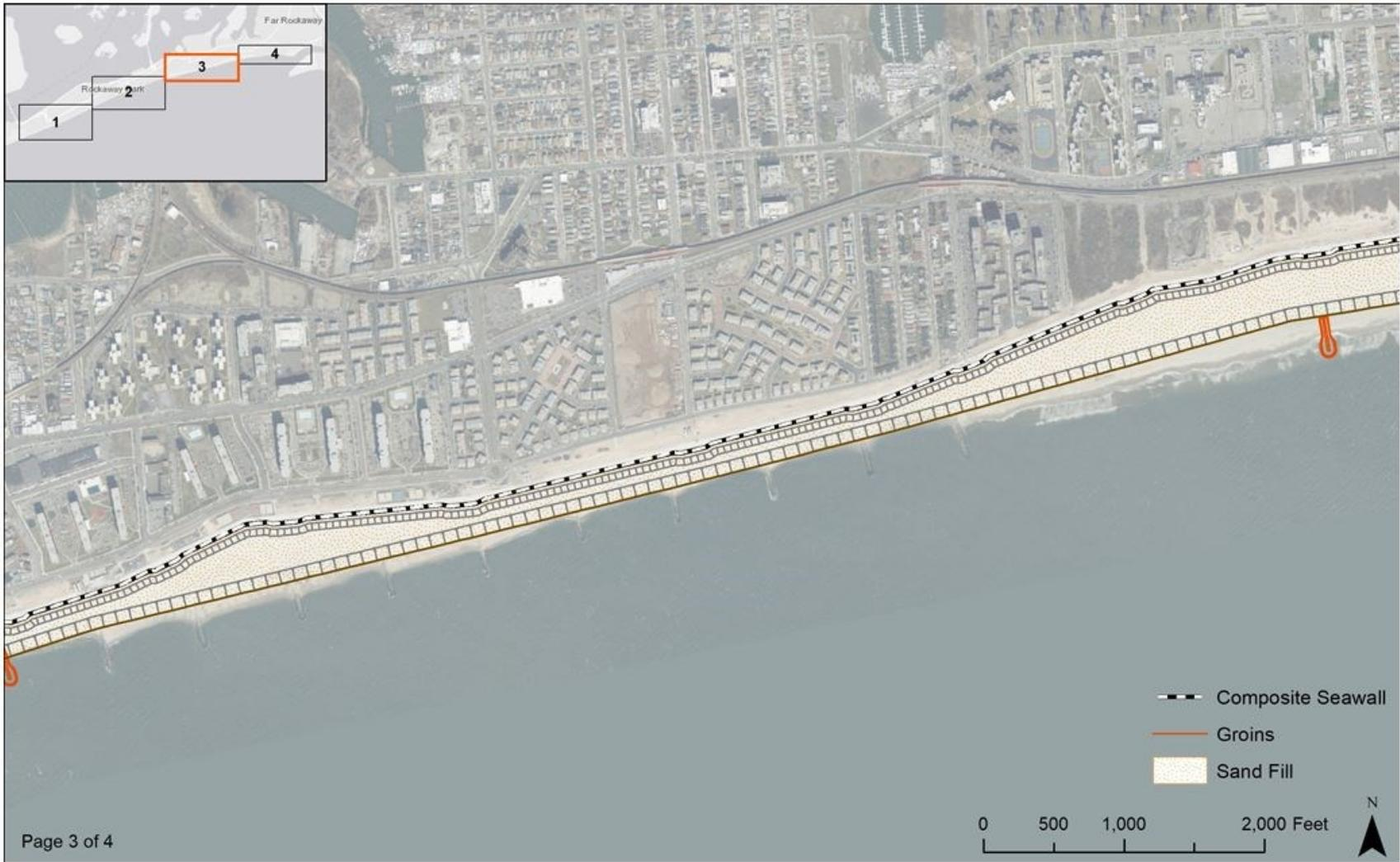
**Figure 6-6c: Atlantic Shorefront Component of Recommended Plan (3 of 4)**
