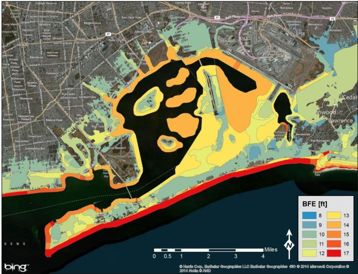
**Figure 2-1: Preliminary FEMA Map Elevations (NAVD88) for the Study Area**
