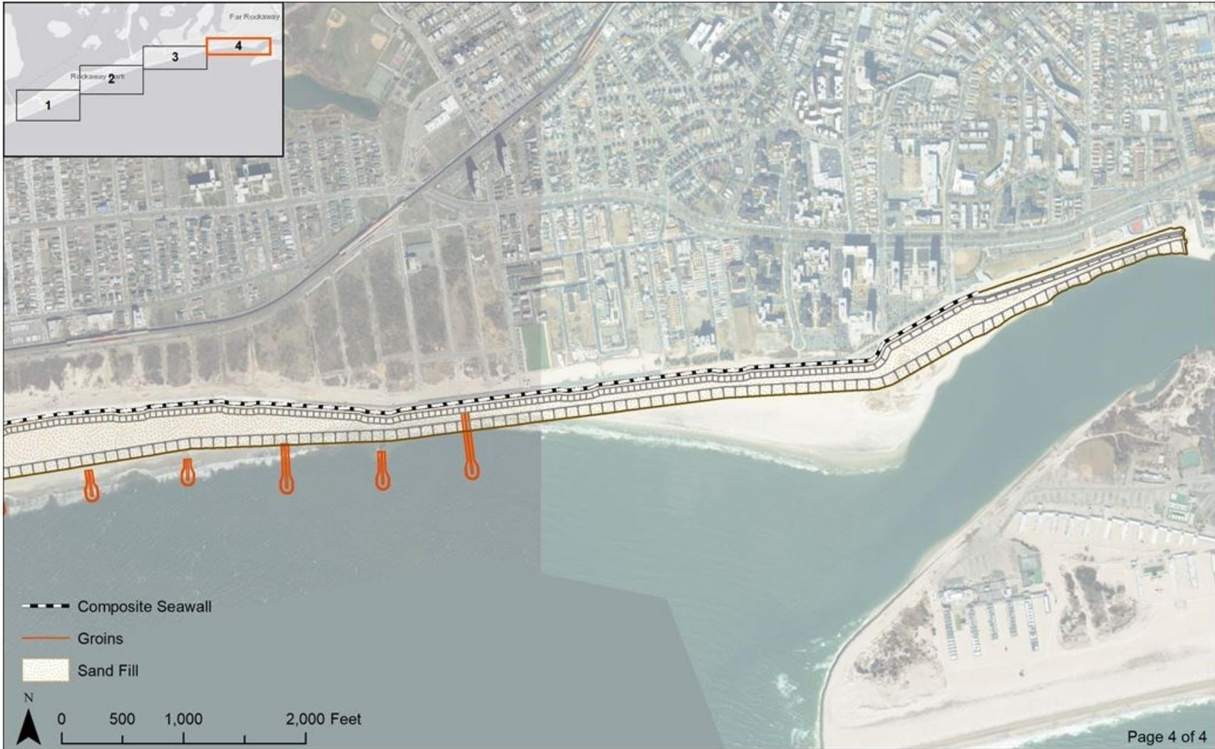
**Figure ES-4d: Atlantic Shorefront Component of Recommended Plan (4 of 4)**
