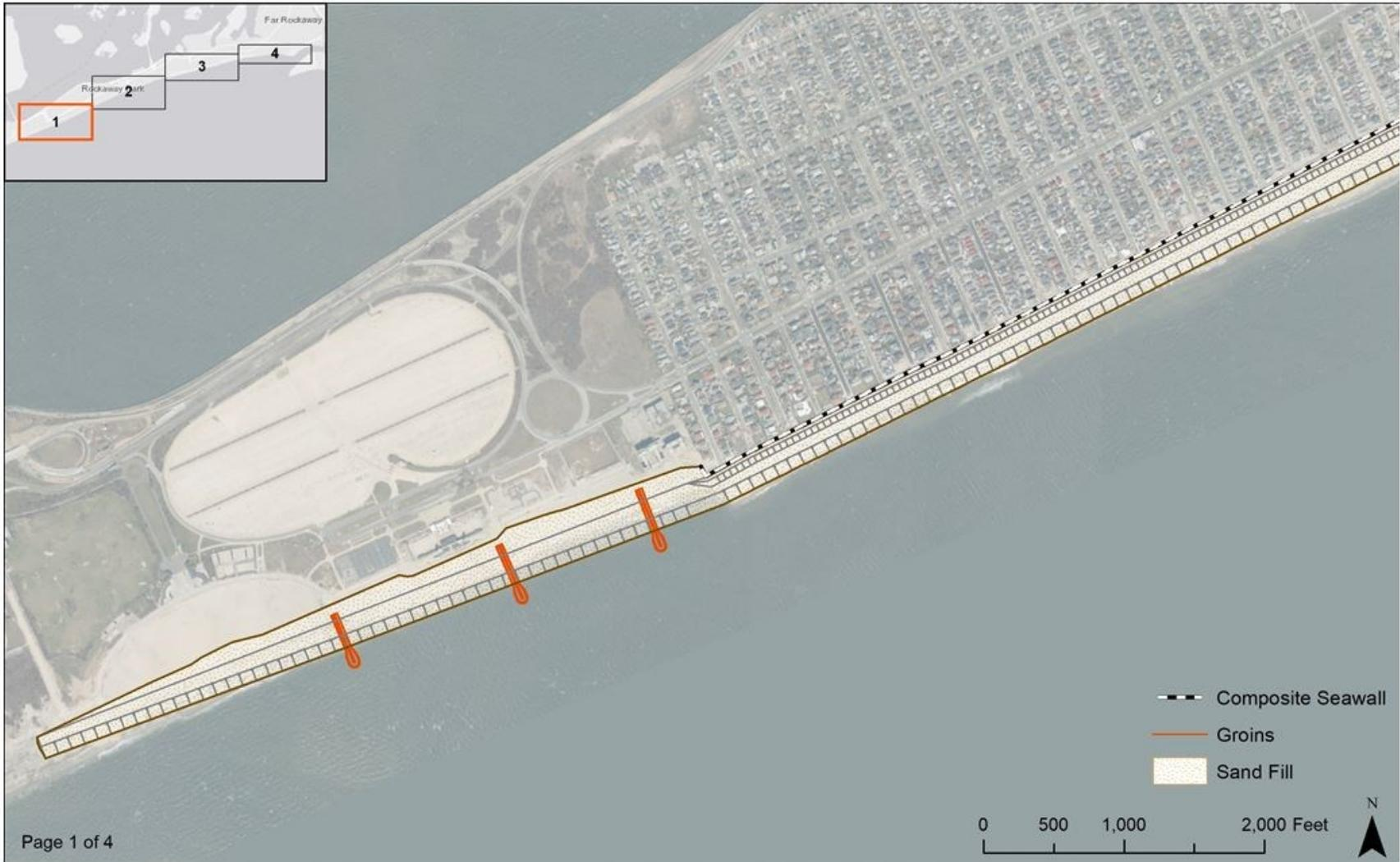
**Figure 6-6a: Atlantic Shorefront Component of Recommended Plan (1 of 4)**
