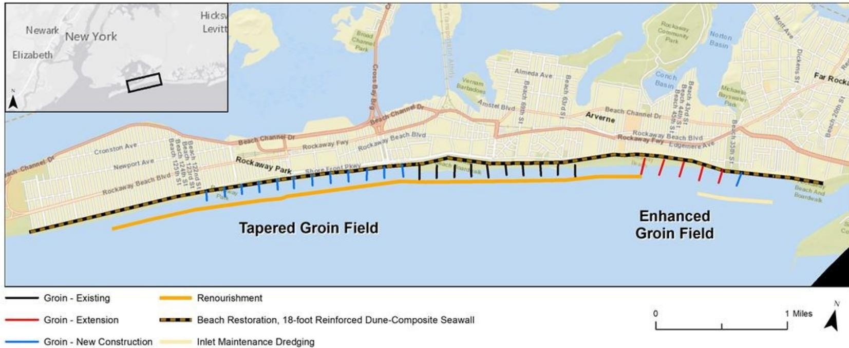
**Figure 6-5: Atlantic Shorefront Component of the Recommended Plan - Overview**
