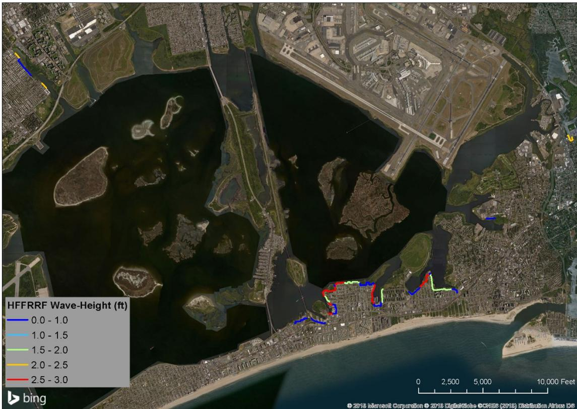
**Figure 5-13: Calculated Wave-heights at HFFRRF Alignments**
