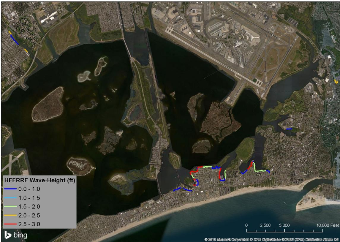
**Figure 5-13: Calculated Wave-heights at HFFRRF Alignments**
