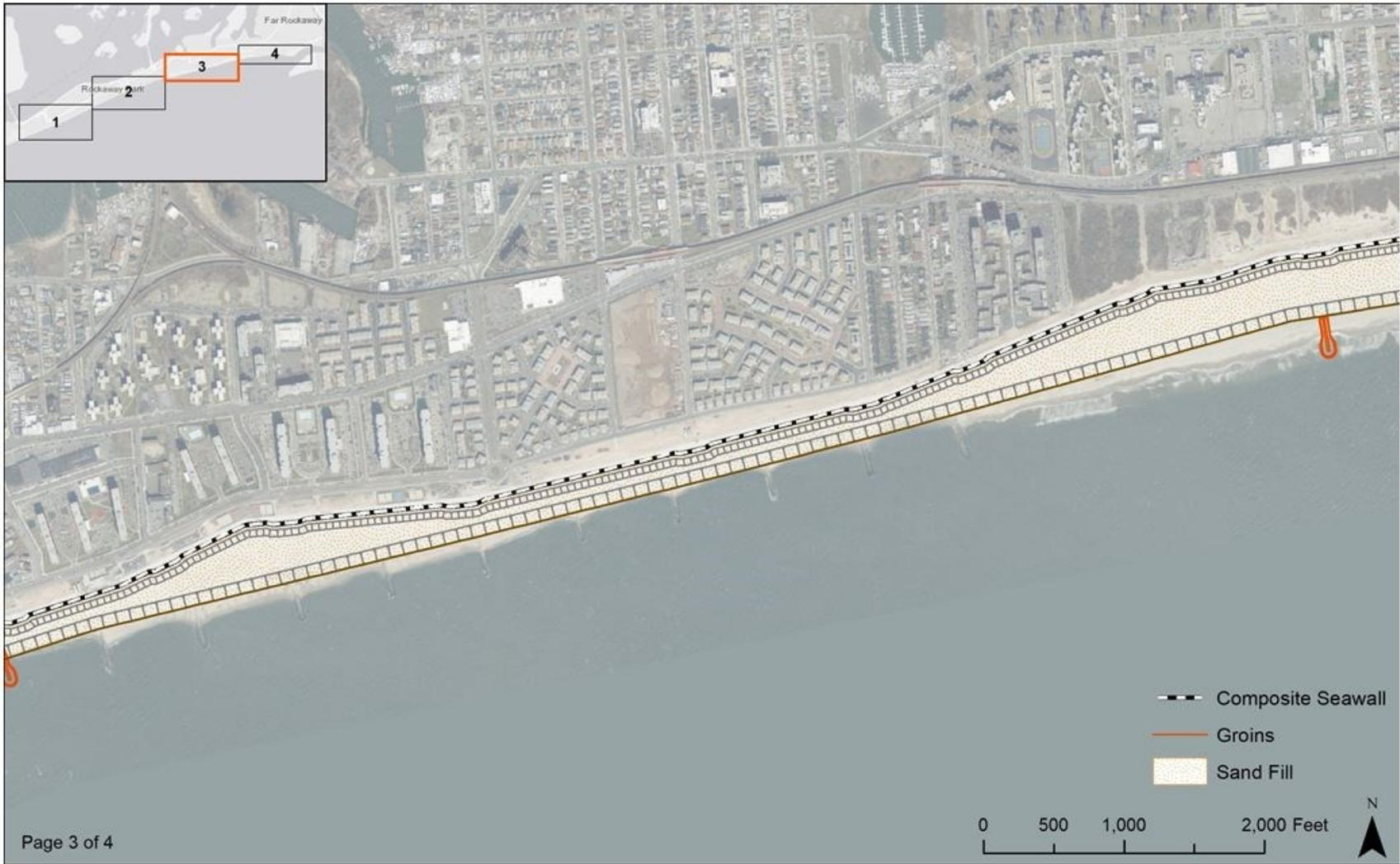
**Figure ES-4c: Atlantic Shorefront Component of Recommended Plan (3 of 4)**
