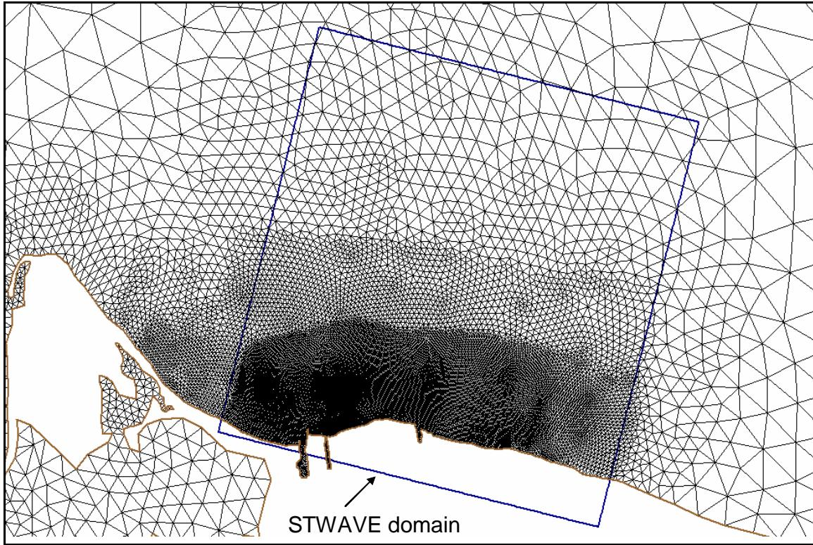
**Figure 24. STWAVE domain overlain on ADCIRC mesh to evaluate processes due to the presence of the power plant.**
