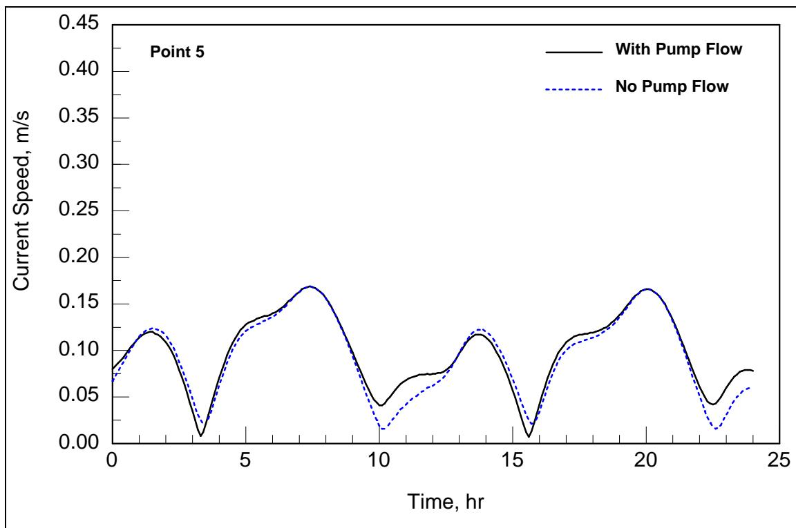
**Figure 41. Comparison of current speed at Point 5 (370m from shore) with plant discharge on versus discharge off.**
