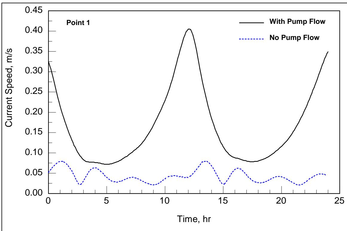
**Figure 38. Comparison of current speed at Point 1 (70m from shore) for conditions with plant discharge on versus plant discharge off.**
