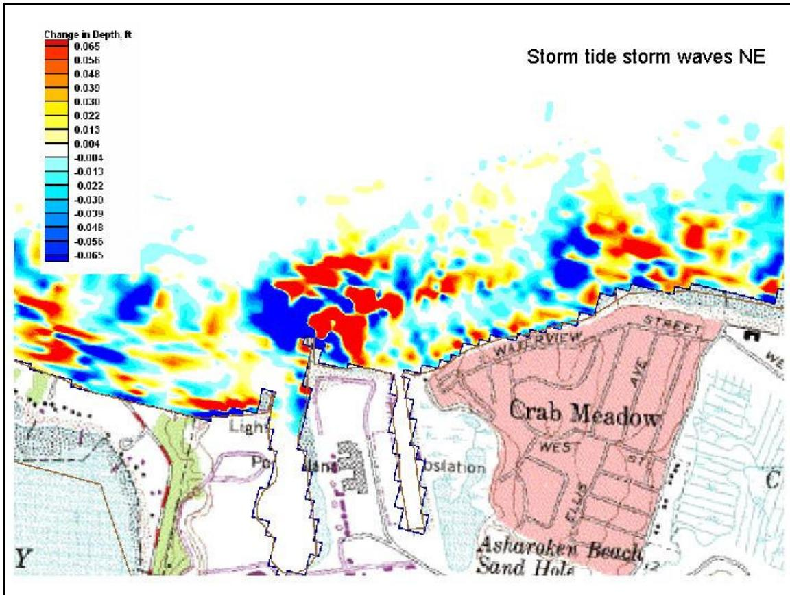
**Figure 31.** Depth changes from 24 hours of storm tidal currents and storm waves from the northeast.
