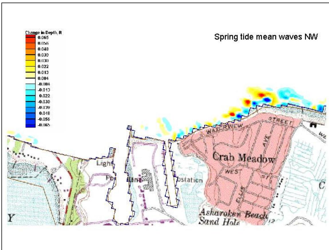
**Figure 30. Depth change due to 24 hours of spring tidal current with mean daily waves from northwest.**
