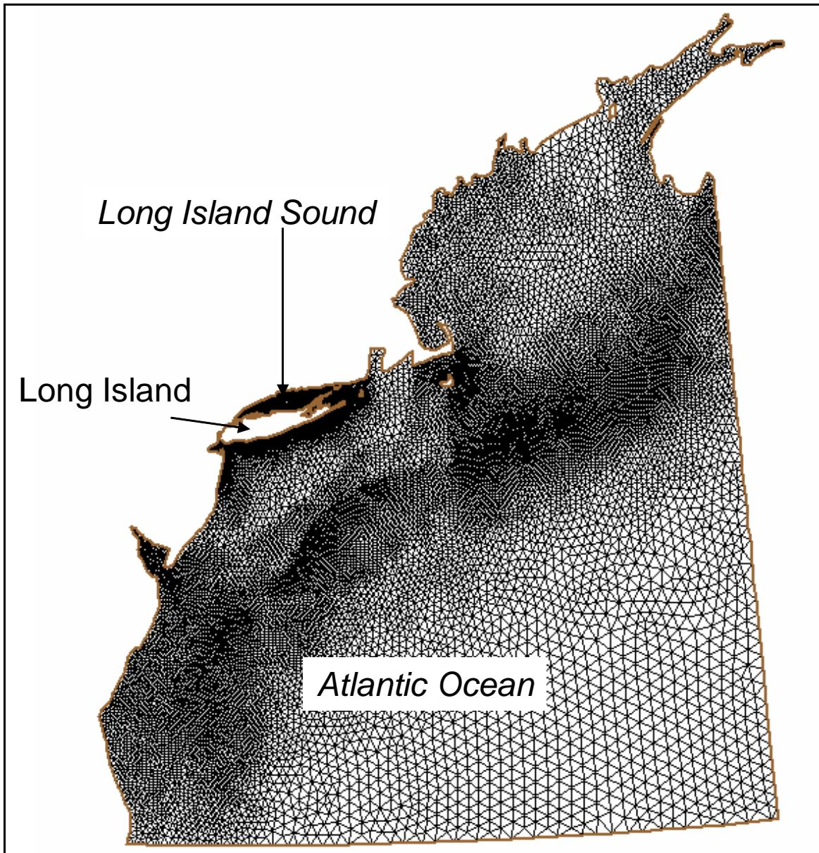
**Figure 14. Finite-element mesh used for ADCIRC modeling**
