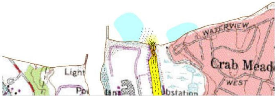
**Figure 35.** Difference at Hour 4 between spring tide flow field with discharge on minus discharge off (maximum flood tide).
