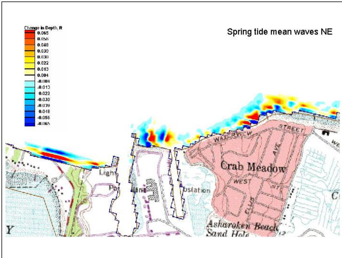
**Figure 29.** Depth change due to 24 hours of spring tidal current and mean daily waves from northeast.
