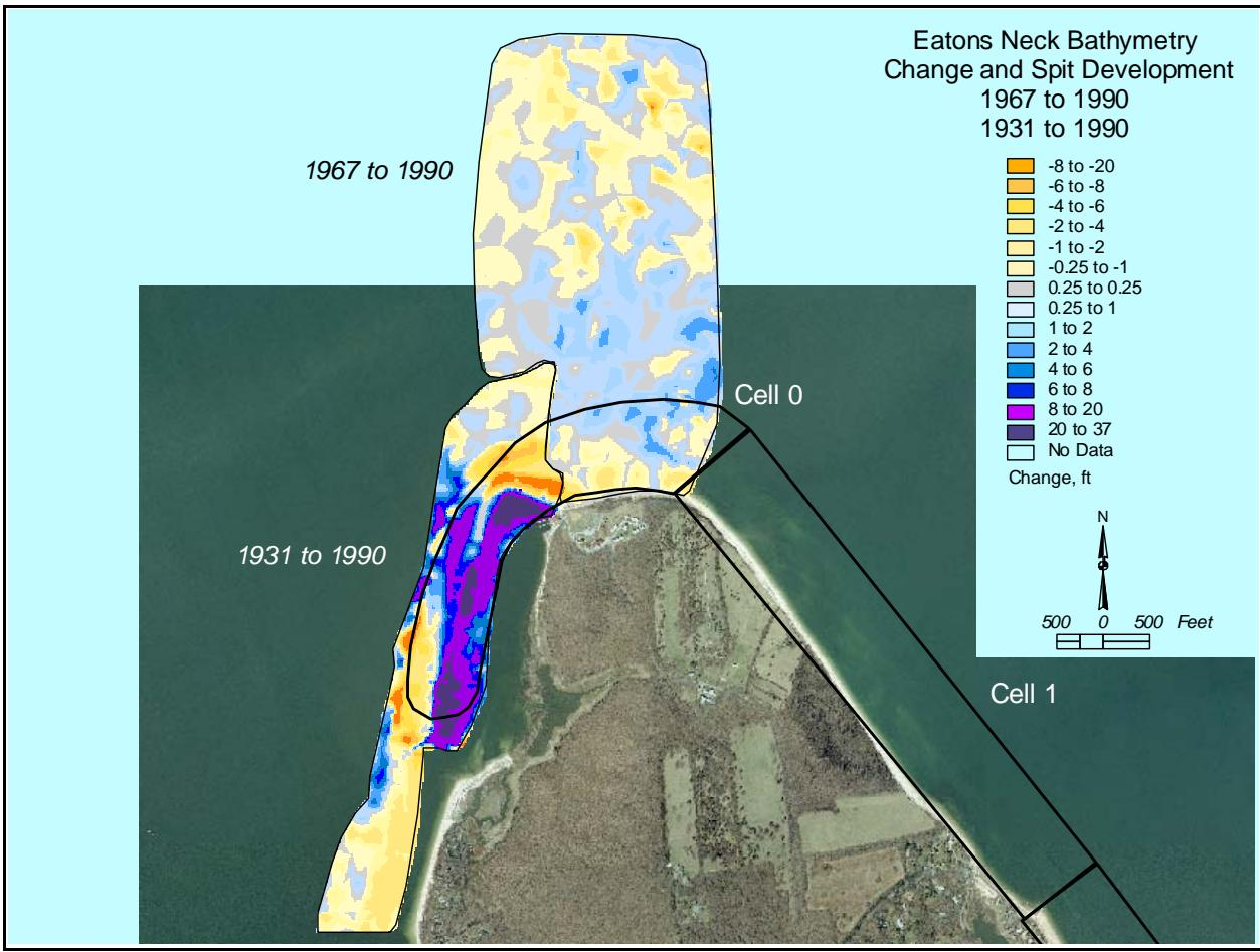
**Figure 11. Bathymetric change at Eatons Neck spit, 1931 to 1990.**
