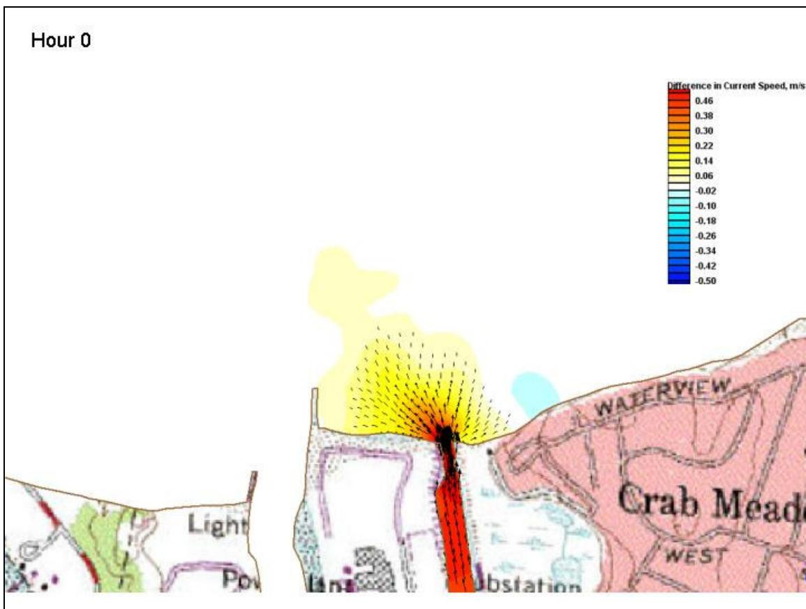
**Figure 34.** Differences at Hour 0 in flow velocity at spring tide between the discharge on and the discharge off (intermediate tide).
