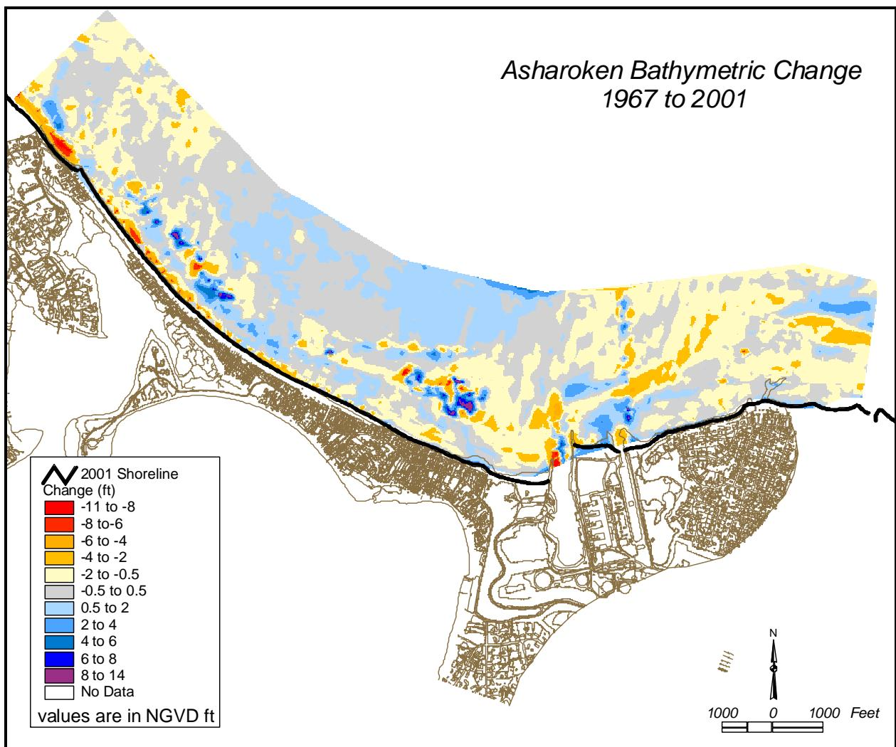
**Figure 10.** Bathymetric change surface, 1967 to 2001.
