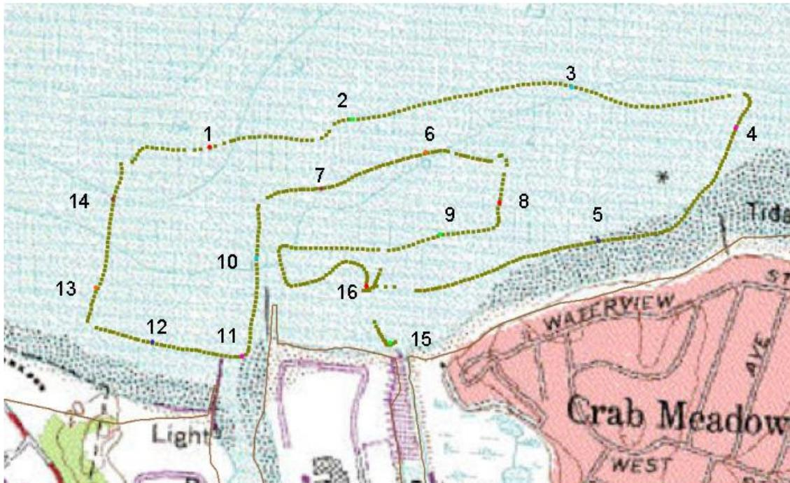
**Figure 22.** Model comparison locations (red dots) along field current measurement transects at 0824. Note that one transect was able to be traversed into the intake channel because of sufficient high tide.
