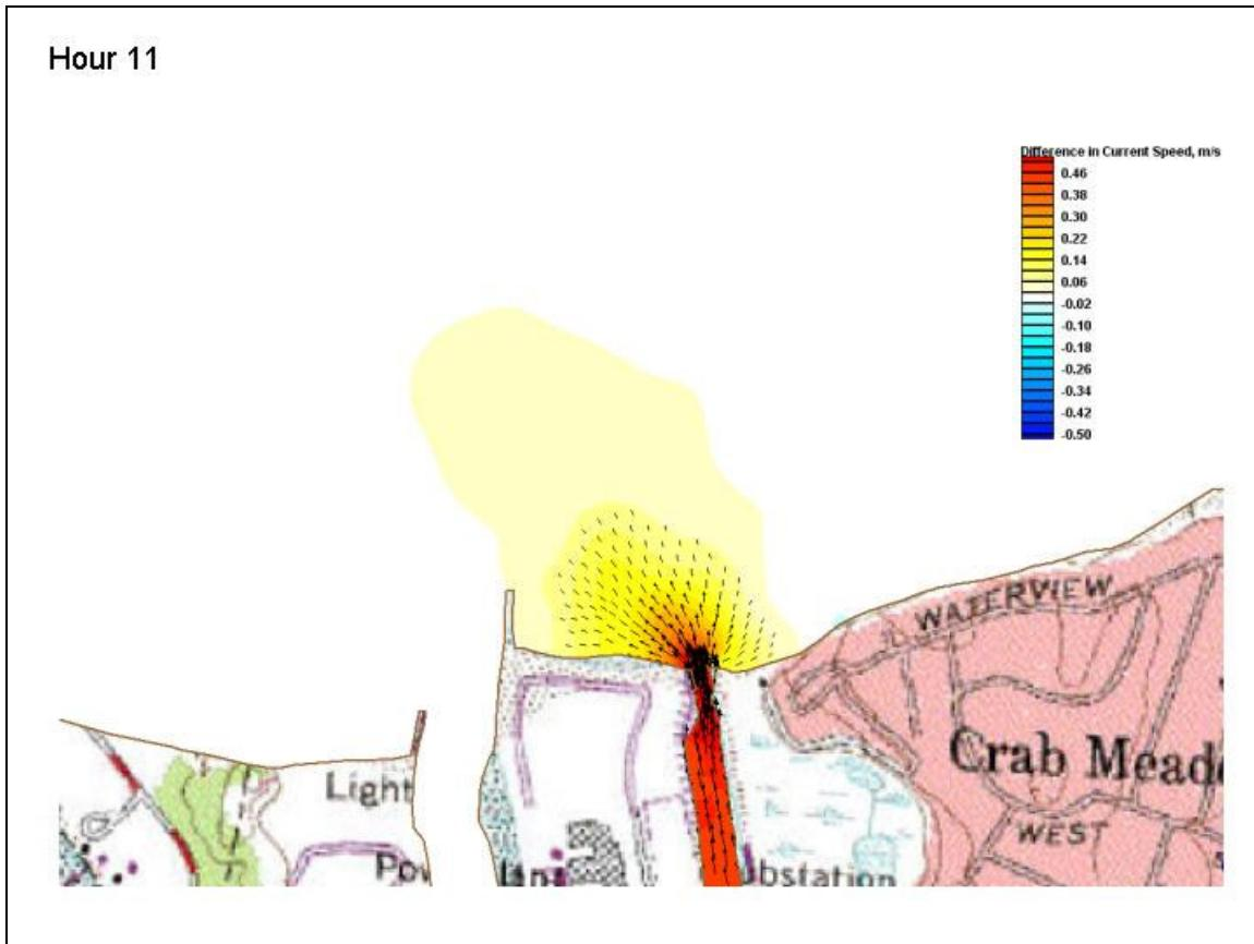
**Figure 36. Difference in spring tide flow field with discharge on minus discharge off (maximum ebb tide).**
