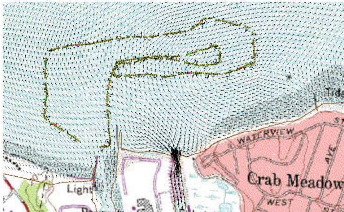
**Figure 21.** Comparison of model vector field and current measurements (green dots) at 1314.
