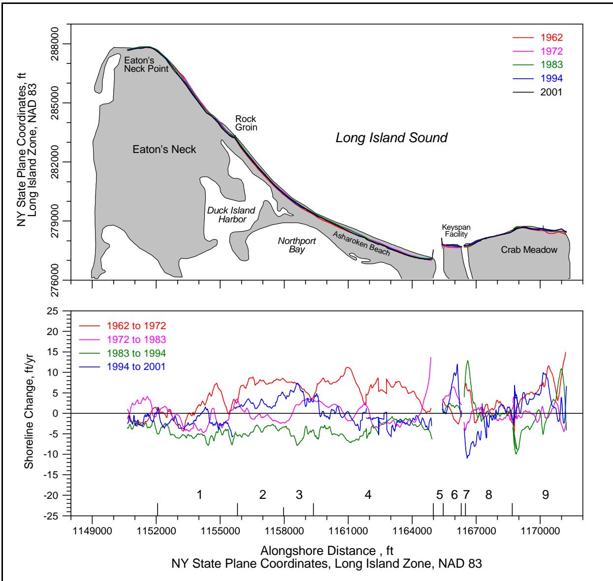
**Figure 4. Decadal shoreline change at Asharoken Beach between 1962 and 2001. Sediment budget polygon boundaries shown for reference.**
