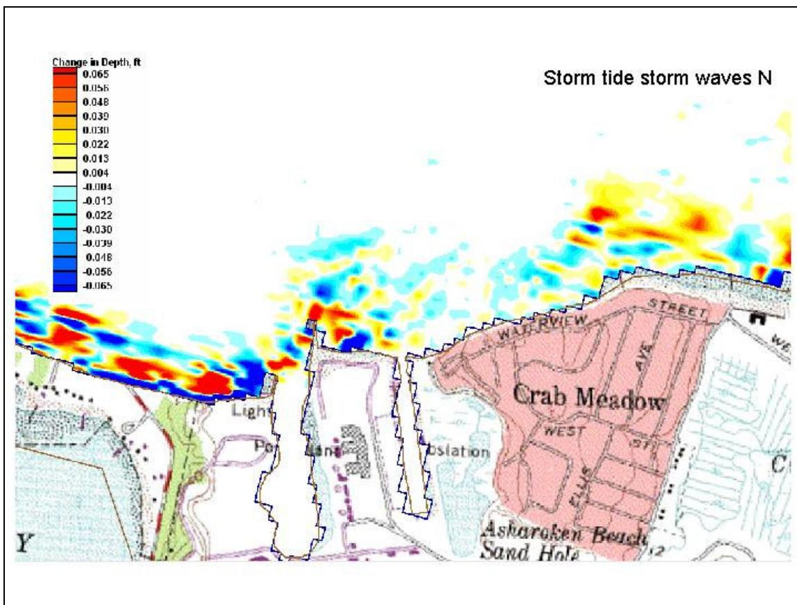
**Figure 32. Depth change due to 24 hours of storm tide and storm waves from the north.**
