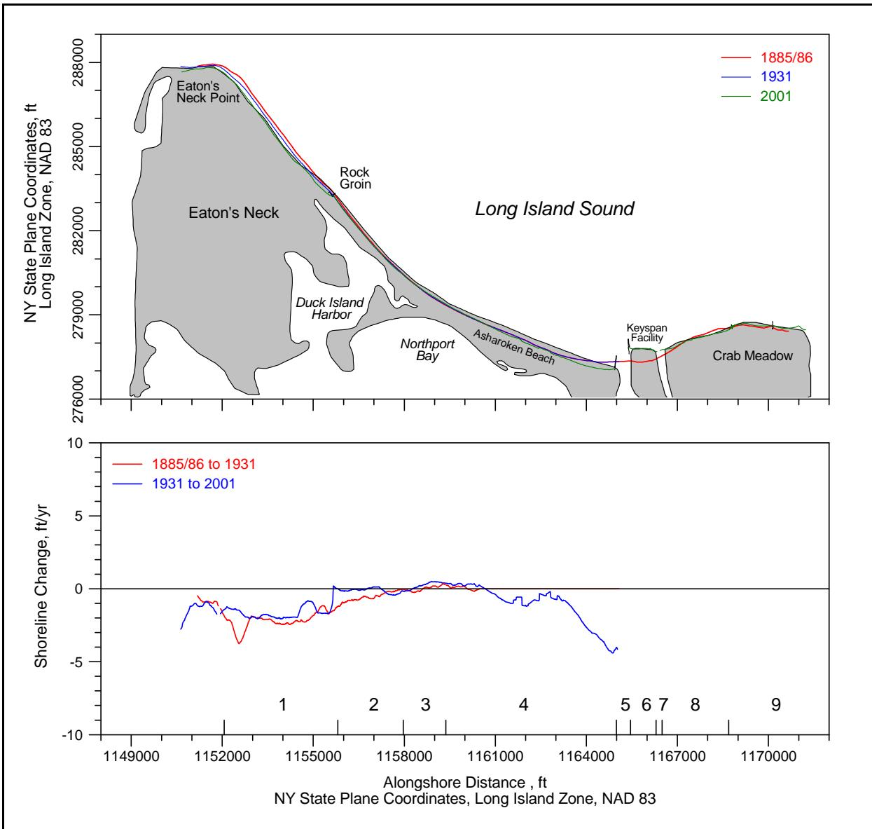
**Figure 5. Long-term shoreline change at Asharoken Beach between 1885/86 and 2001. Sediment budget polygon boundaries shown for reference.**
