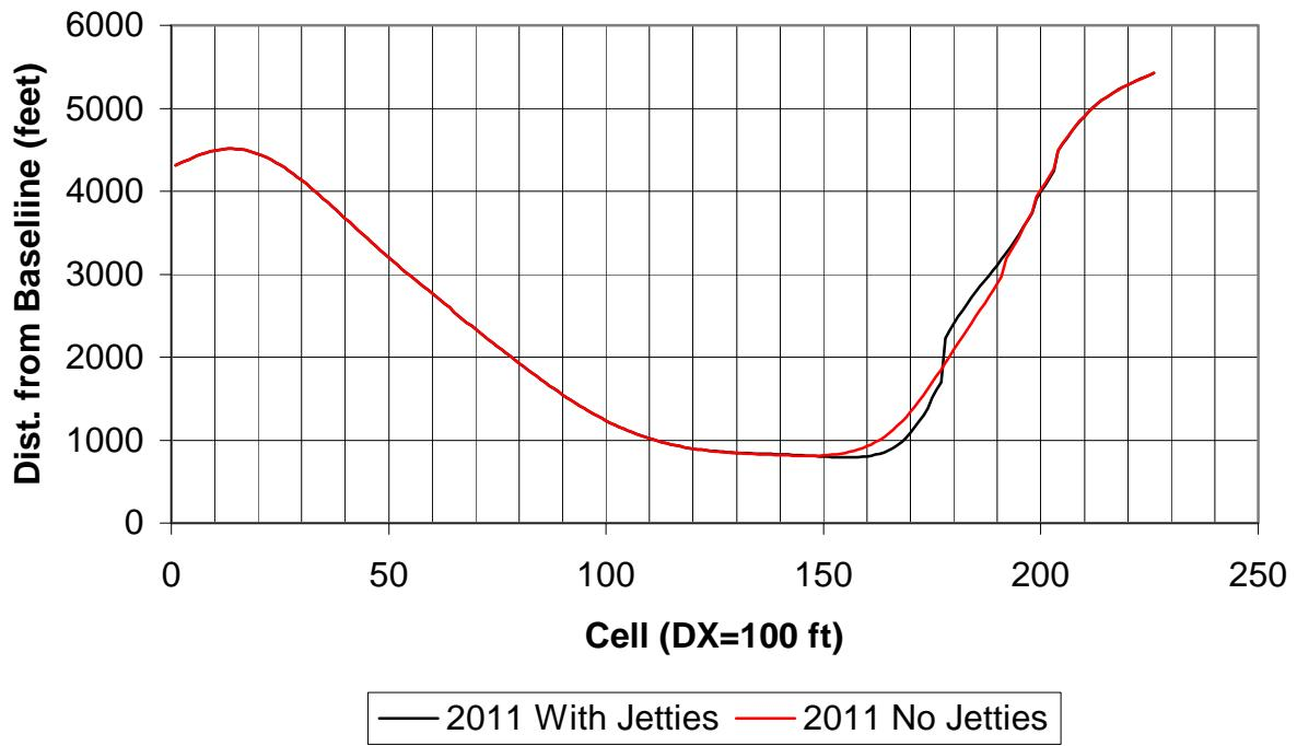
**Figure 50. Effect of removal of jetties at the power plant.**
