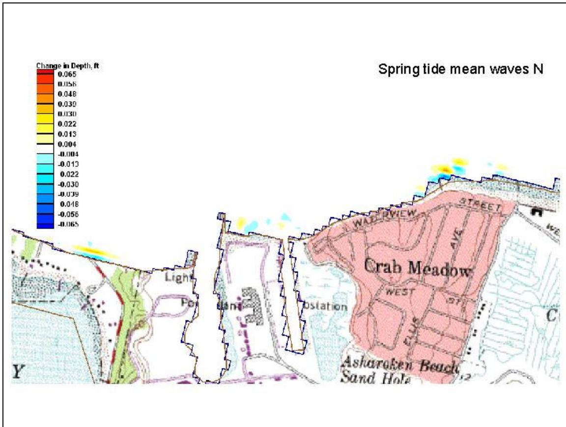
**Figure 28. Depth change due to 24 hours of spring tidal current with mean daily waves from the north.**
