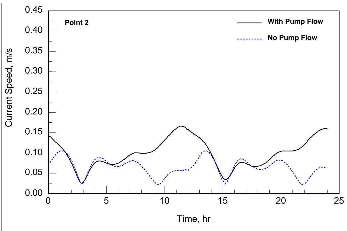
**Figure 39. Comparison of current speed at Point 2 (150m from shore) with plant discharge on versus discharge off.**
