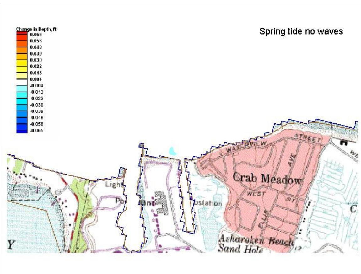
Figure 27. Depth change due to 24 hours of spring tidal current at Asharoken.
