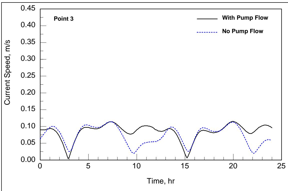
**Figure 40. Comparison of current speed at Point 3 (220m from shore) with plant discharge on versus discharge off.**
