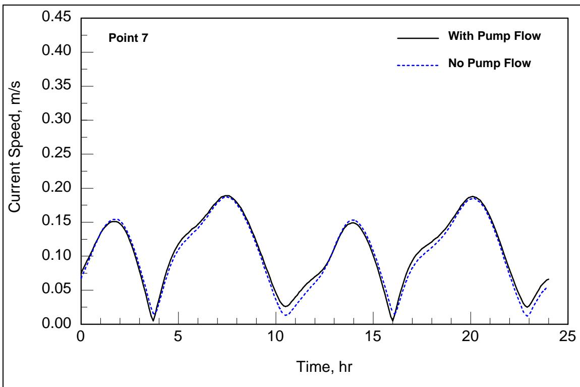
**Figure 42. Comparison of current speed at Point 7 (500m from shore) with plant discharge on versus discharge off.**
