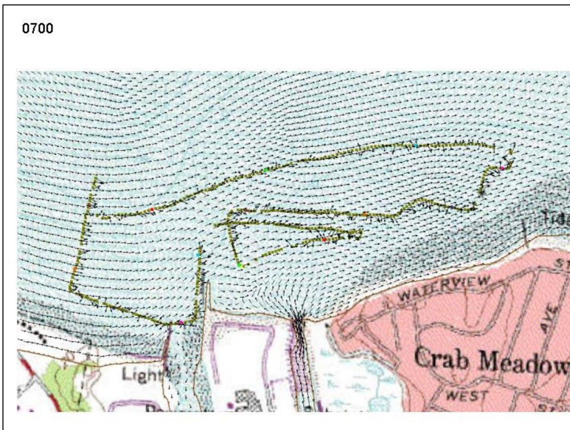
**Figure 19.** Modeled current vector field compared to measurements (shown at green dots) at 0700.
