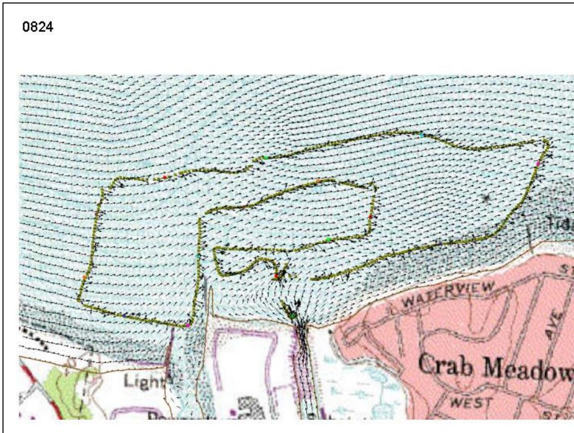
**Figure 23. Comparison of model current vector field versus measurements at time 0824.**
