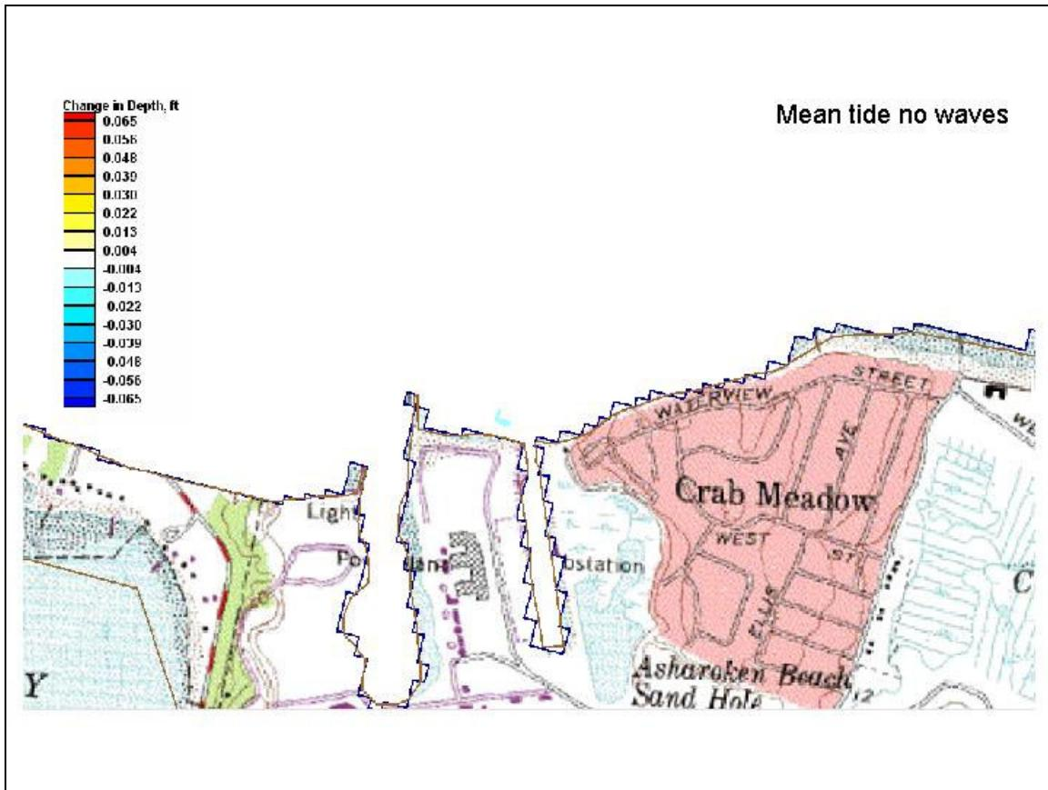
Figure 26. Depth change due to 24 hours of mean tidal current at Asharoken
