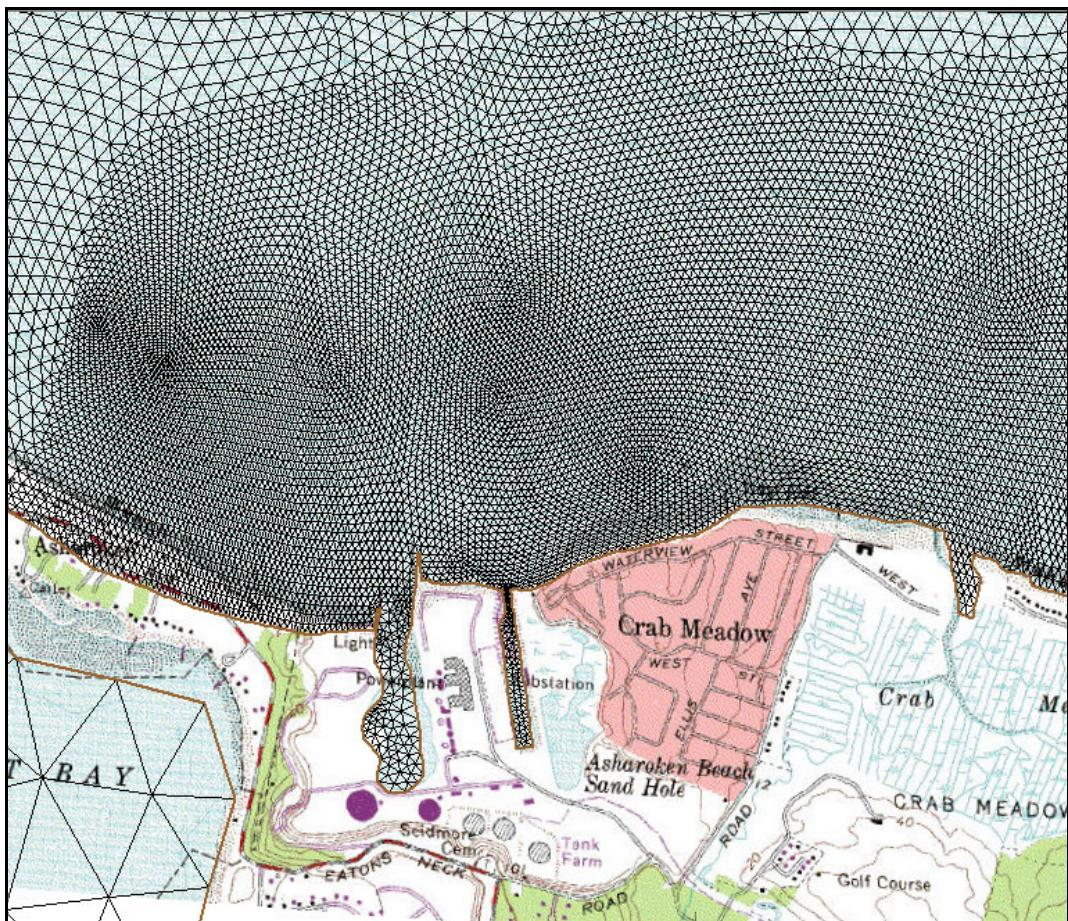
**Figure 16.** Detail of ADCIRC mesh in Asharoken area.
