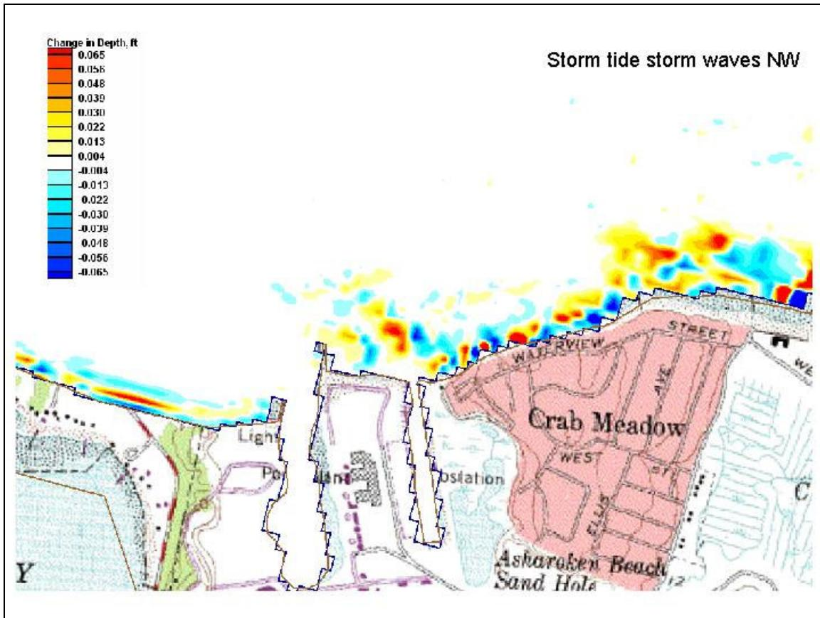
**Figure 33. Depth change due to 24 hours of storm tidal current with storm waves from the northwest.**
