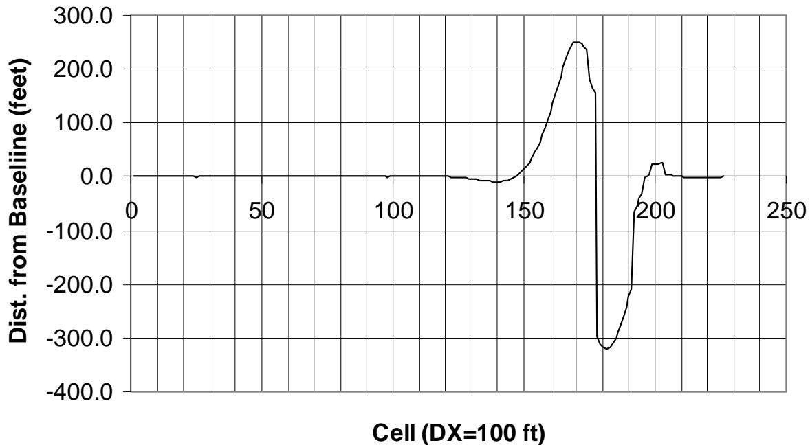
**Figure 51. Effect of the removal of the jetties at power plant.**
