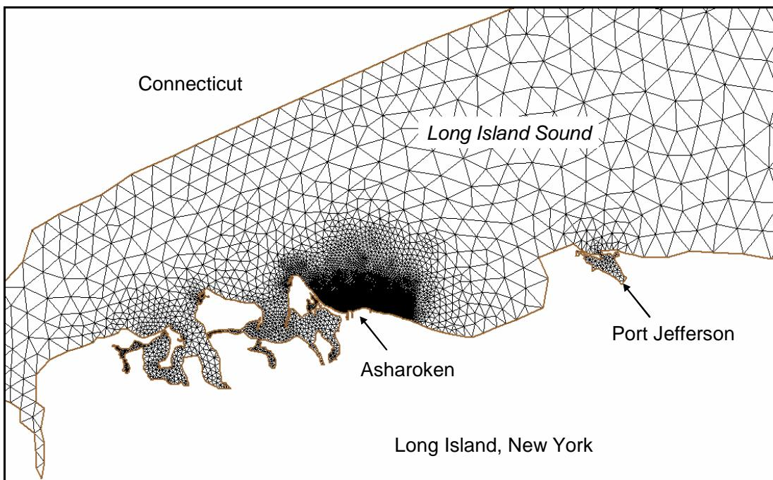
**Figure 15.** Detail of ADCIRC mesh in central Long Island Sound.
