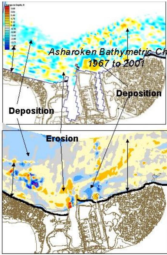
**Figure 43. Comparison of bathymetric change from 1967 to 2001 between the model (top figure) and surveys (bottom figure).**
